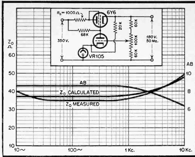
Fig. 14. (left) How Z<sub>o</sub> increases when Z<sub>s</sub> is in the form of a 1000-ohm resistance. Comparison with Fig. 13 indicates a considerable increase.
