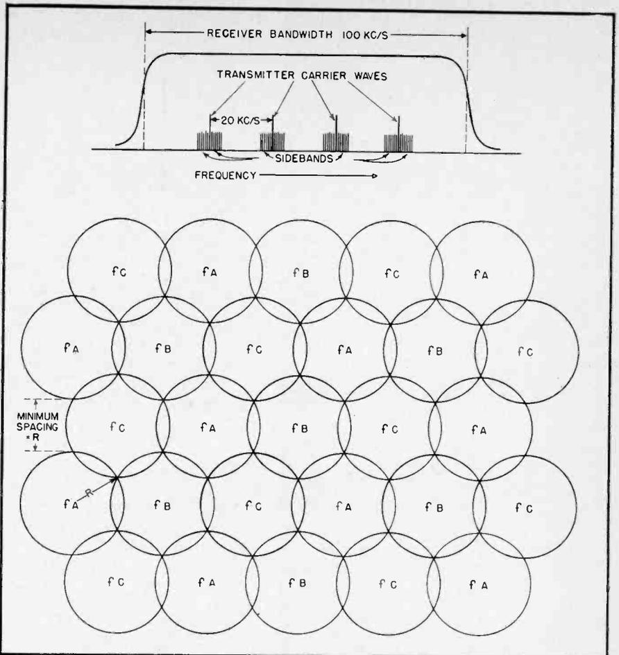
Fig. 1. (top) In the multi-carrier system, a number of transmitters, synchronously amplitude-modulated, are accepted simultaneously by the receivers, ensuring that in all locations at least one is adequately received. The above band widths, used in the development tests, are now being reduced to about one half.
