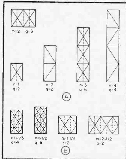
Fig. 1. (A) Commonly used integral winding patterns. Dotted lines indicate the "herringbones". No herringbones occur when the number of crossovers is even ( $n = 2, 4$ , etc.). (B) Less commonly used functional winding patterns.
