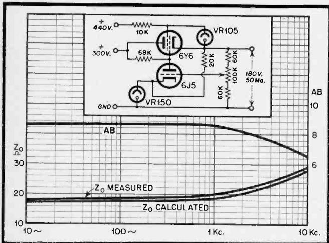
Fig. 16. (left) Even though  $R_p$  is higher with tetrode connection, the increase in  $\mu$  holds  $Z_0$  at about the same level. Compare with Fig. 13. The ripple reduction factor is lower, however, with this connection.
