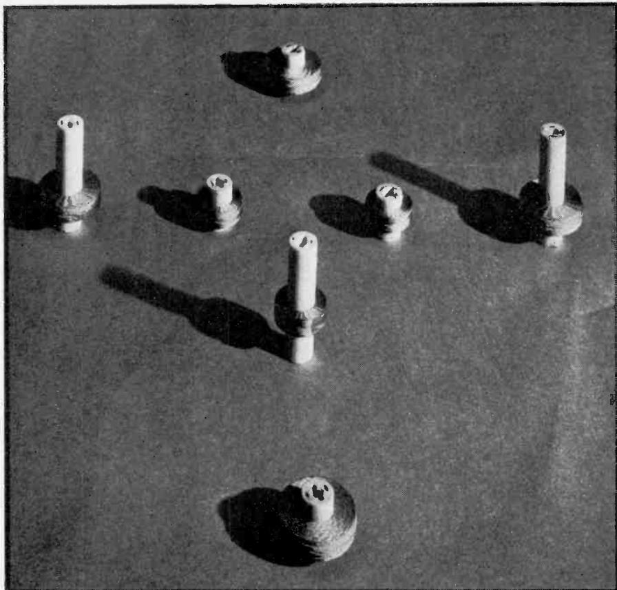
Fig. 2. Shown clearly are properly wound universal coils. The winding around the dowel appears to be a regular and flawless pattern.
