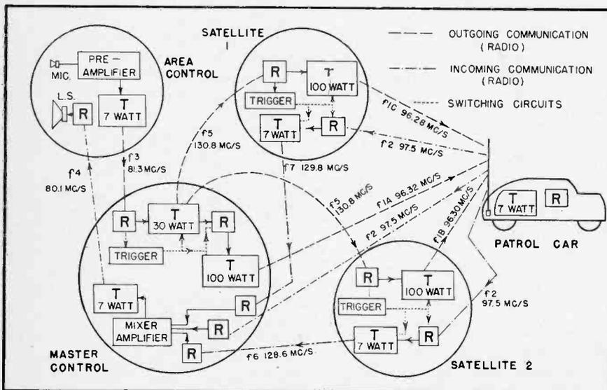
Fig. 2. Schematic diagram of a triple-carrier communication system, which has been given exhaustive field trials.
