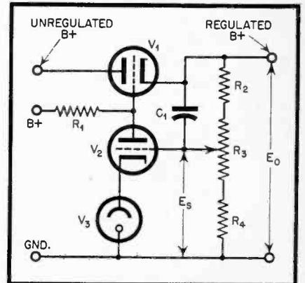
Fig. 1. (left) Simple degenerative regulator. Fig. 2. (center schematic) Simple regulator redrawn as a cathode follower with voltage feedback. Fig. 3. (right) Regulator with series impedance in the source.
