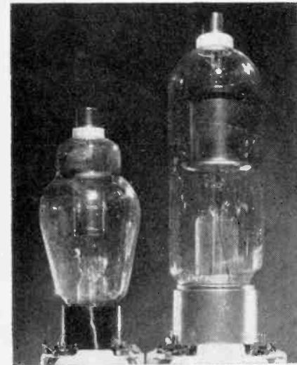
ment volts, peak inverse voltages as high as 10,000 volts, and a maximum average plate current of .25 amp. The 872A/872 has a 5-volt filament and carries a maximum peak inverse voltage rating of 10,000 volts and a maximum average current rating of 1.25 amp.
