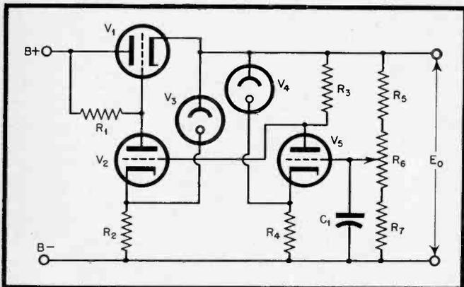
Fig. 6. (left) Regulator using a double triode amplifier tube.
