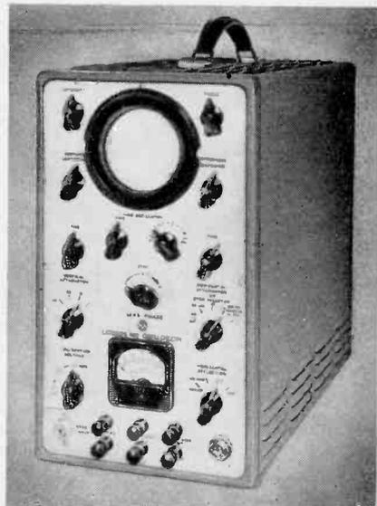
vision signal expansion for checking square-wave time, and for checking irregularly timed pulses. The intensifying amplifier increases the brilliancy of the waveform after the time-base generator is triggered, permitting examination and photography of small, otherwise, faint, and extremely short pulses. Signal-triggered deflection, line frequency deflection, and blanking are some of the other unusual features of this new RCA oscilloscope.
