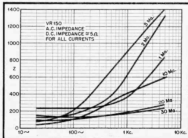
Fig. 20. (Left) Impedance characteristics of VR-150.
