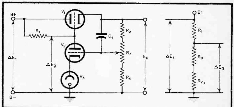
Fig. 7. Amplifier circuit redrawn to show the ripple voltage distribution. The equation for determining the ripple,  $\Delta E_g$ , is given in the text.
