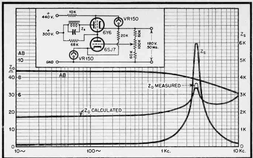
Fig. 18. Use of the tetrode connected series tubes reduces resonant effects. Compare with Fig. 15.
