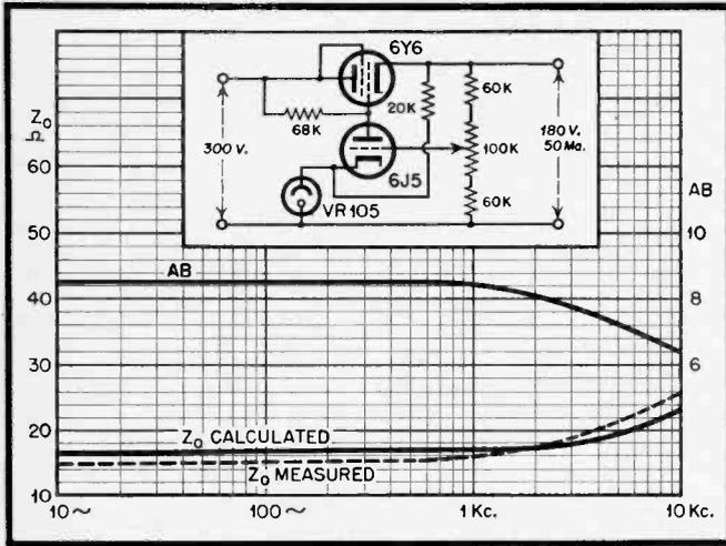
Fig. 13. (left) Comparison of calculated and measured values for  $Z_o$ . Note the increase of  $Z_o$  when AB decreases.
