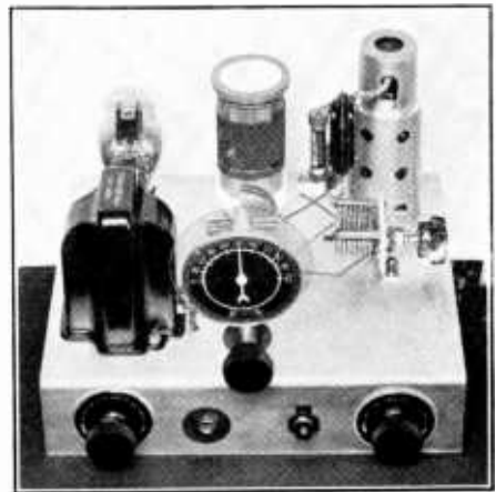
The AC "Gainer" with front panel removed to show correct arrangement of parts.
