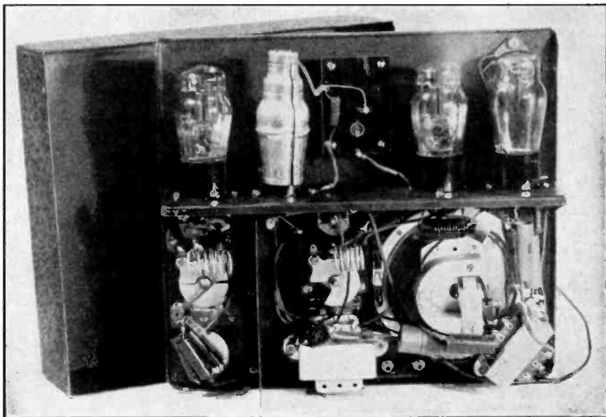
FIG. 24—Interior view of 5-meter auto set. Note shield partition between coils.
