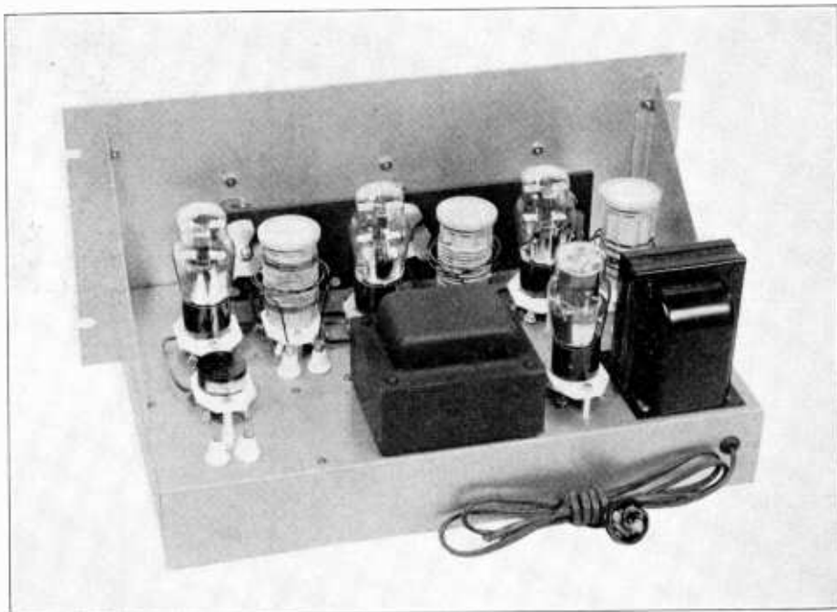
"3-53" 1936 Jones Exciter, 160 meters to 10 meters. The power supply, mounted on the Exciter chassis, makes this a complete and independent driving unit for a buffer-amplifier stage.
