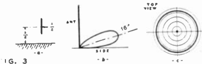
FIG. 3 Half wave antenna, same height as full wave antenna in Fig. 2. Here the radiation is known as 16-degree "low angle" radiation.
