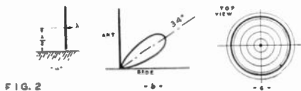
FIG. 2 Full wave antenna gives maximum radiation upward at an angle of 34 degrees from the horizon.
