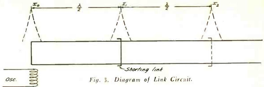
Fig. 3. Diagram of Link Circuit.
