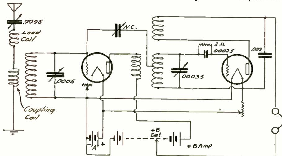
Fig. 2. Modified Browning-Drake Circuit.
