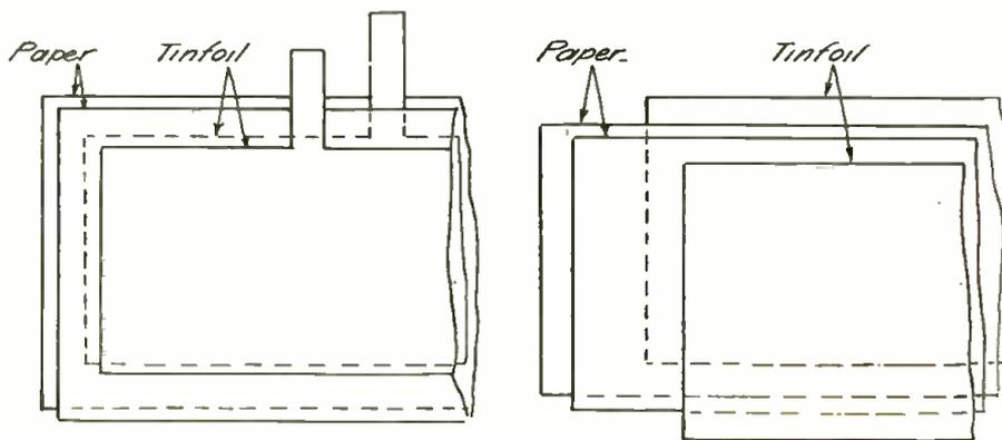
Fig. 5. Methods of Condenser Construction.
