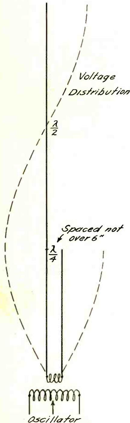
Fig. 3. Parallel Wire Antenna System Vertical Mast-Antenna.
