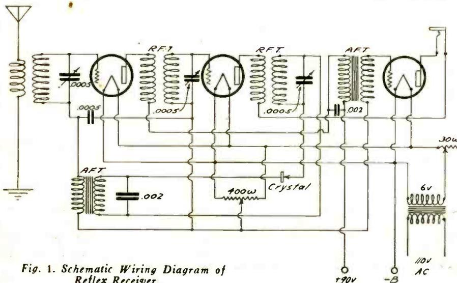
Fig. 1. Schematic Wiring Diagram of Reflex Receiver.
