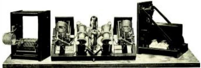
The illustration shows Mr. Best's short wave transmitter, using NATIONAL Type DXT transmitting condensers. These condensers are designed for continuous operation at 1500 volts—400 meters.
