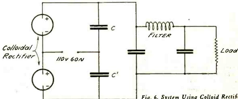
Fig. 6. System Using Colloidal Rectifiers.
