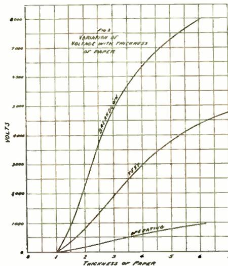
Fig. 2. Variation of Voltage with Thickness of Paper.
