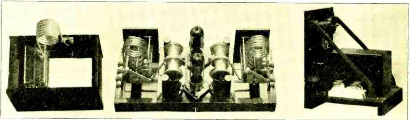
Fig. 2. Details of Transmitter, Showing Individual Panels.
