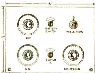
Fig. 7. Panel Arrangement for Anti-Static Instrument.
