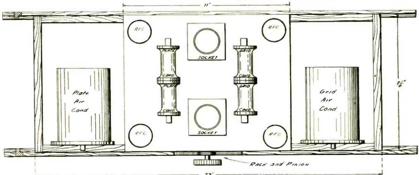
Fig. 6. Plan of Oscillator Frame.
