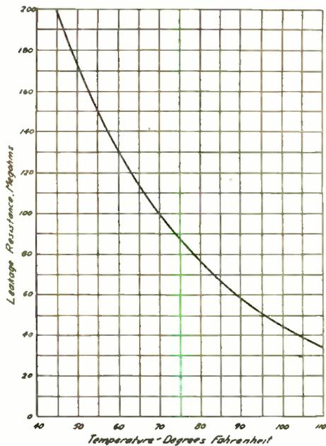
Fig. 4. Variation of Leakage Resistance with Temperature.
