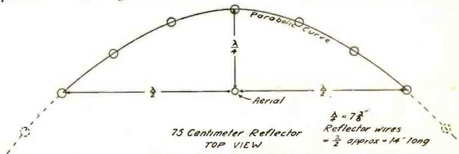
Fig. 4. Diagram of Reflector.
