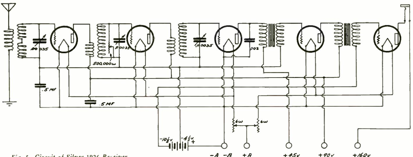
Fig. 5. Circuit of Silver 1926 Receiver.
