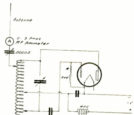
Fig. 2. Method of Coupling Oscillator to Antenna.
