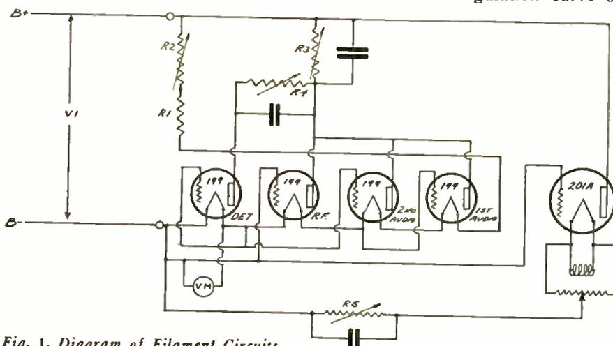
Fig. 1. Diagram of Filament Circuits.
