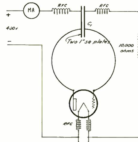
Fig. 1. Fundamental Oscillator Circuit.
