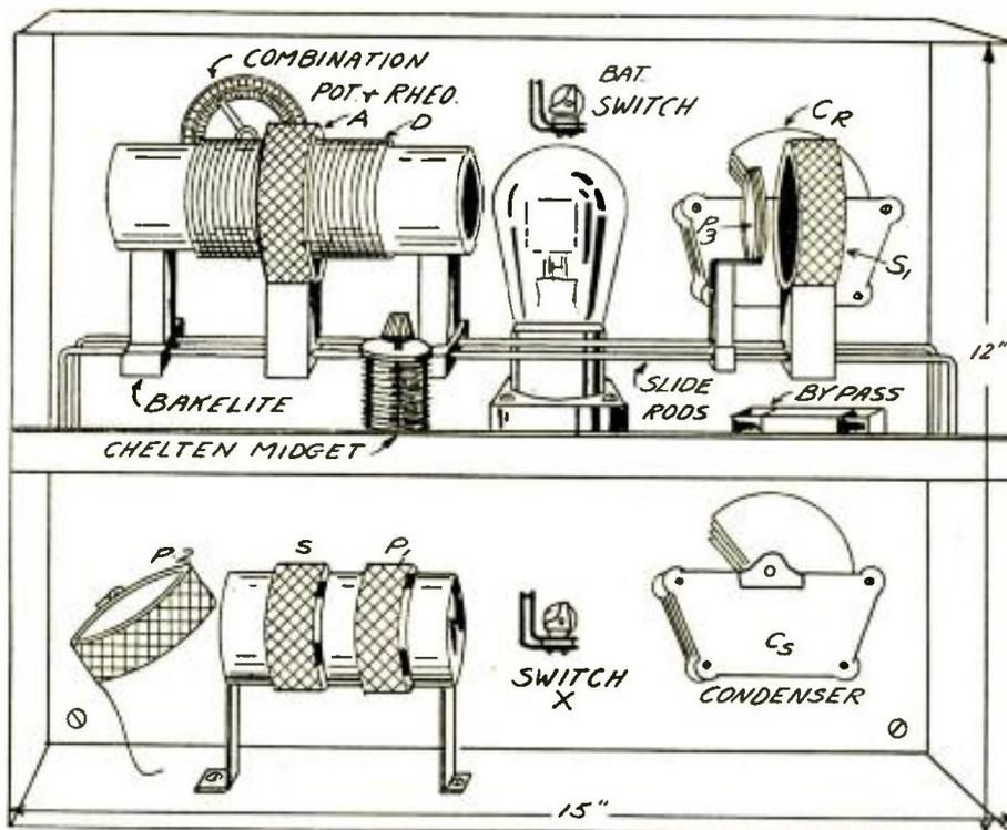
Fig. 6. Rear View of Anti-Static Instrument Assembly.
