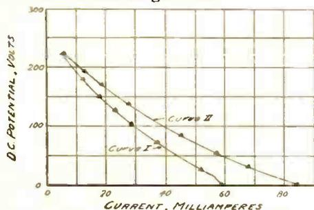
Fig. 4. Curve of Current Output, Using Western Electric 216-A Tubes.
