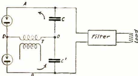
Fig. 1. Theoretical Diagram of Rectifier.
