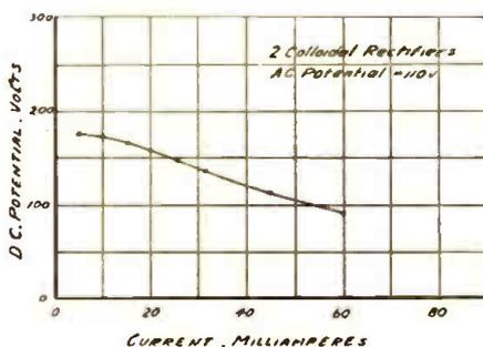
Fig. 7. Colloid Rectifier Current Output Curve.
