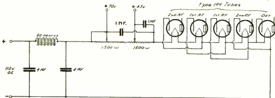
Fig. 1. ABC Battery Eliminator for 110 Volts D. C.
