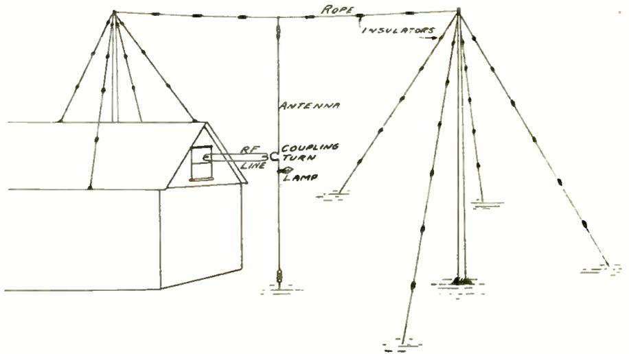
Fig. 1. Vertical Antenna, Using Transmission Line.
