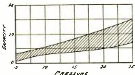
Fig. 1. Variation in Condenser Capacity at Different Pressures.
