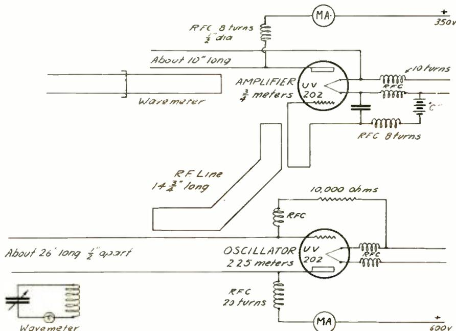
Fig. 2. Master Oscillator Circuit for 75 C. M. Work
