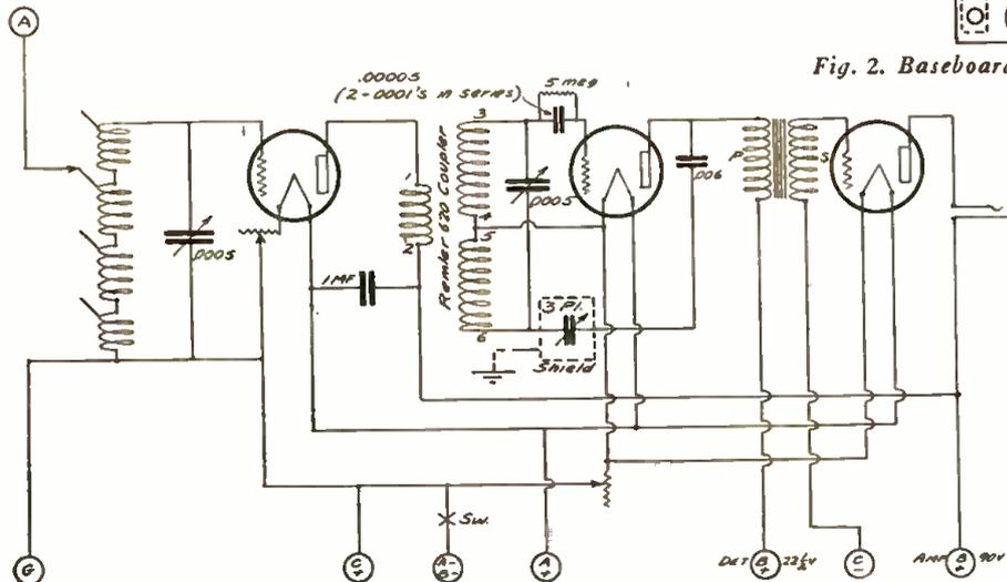
Fig. 1. Circuit Diagram for Efficient Three-tube Set.
