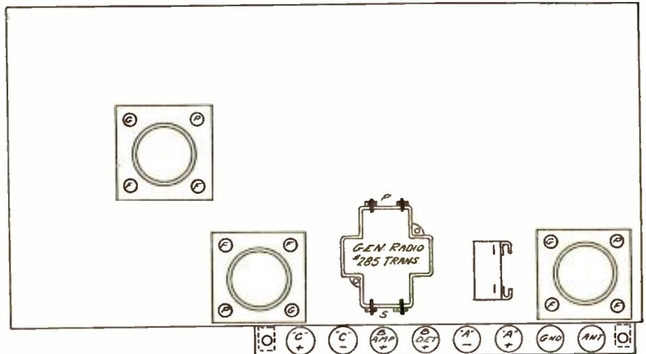
Fig. 2. Baseboard Layout for Three-tube Set.
