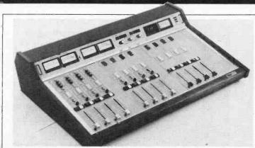
**Broadcast Audio Corporation** has introduced an analog version of its System 14 Digitally-Controlled Audio Console. Basic features and performance are similar, although prices are slightly lower for the System 14A. An optional 5-frequency EQ and pan pot are available on each mixing position. Delivery in 30 days.
