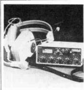
Ramko Research introduces Sidekick, a 4 channel portable mixer. Features include: AB power, 9V; Phantom power, 18V; built-in intercom; full cue with detent on each channel; line tone 1000 Hz, slate tone 400 Hz; clip and/or shoulder strap, case optional; internal ni-cad or alkaline battery com-
