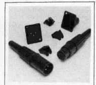
Connectronics Corporation is announcing a new range of XLR connectors at the 1984 NAB Convention. These connectors fill a demand in the audio industry for a high quality, inexpensive range of British-made components. The chassis sockets are rear- and frontmounting, with a P.C.B. mounting socket also available. They are made from glass-filled nylon which makes them durable. Silver plated pins give low-contact resistance and excellent solderability.
