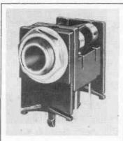
Switchcraft Inc. introduces its new Right Angle Phone Jacks, two in a series of four new low-profile phone jacks for snap-in PC mounting in telecommunications and audio connecting applications. Jack housing features molded tension fingers to provide stable mount. Location pin polarizes mounting for accurate insertion. Available with metal, plastic, and plain (non-threaded) bushings.
