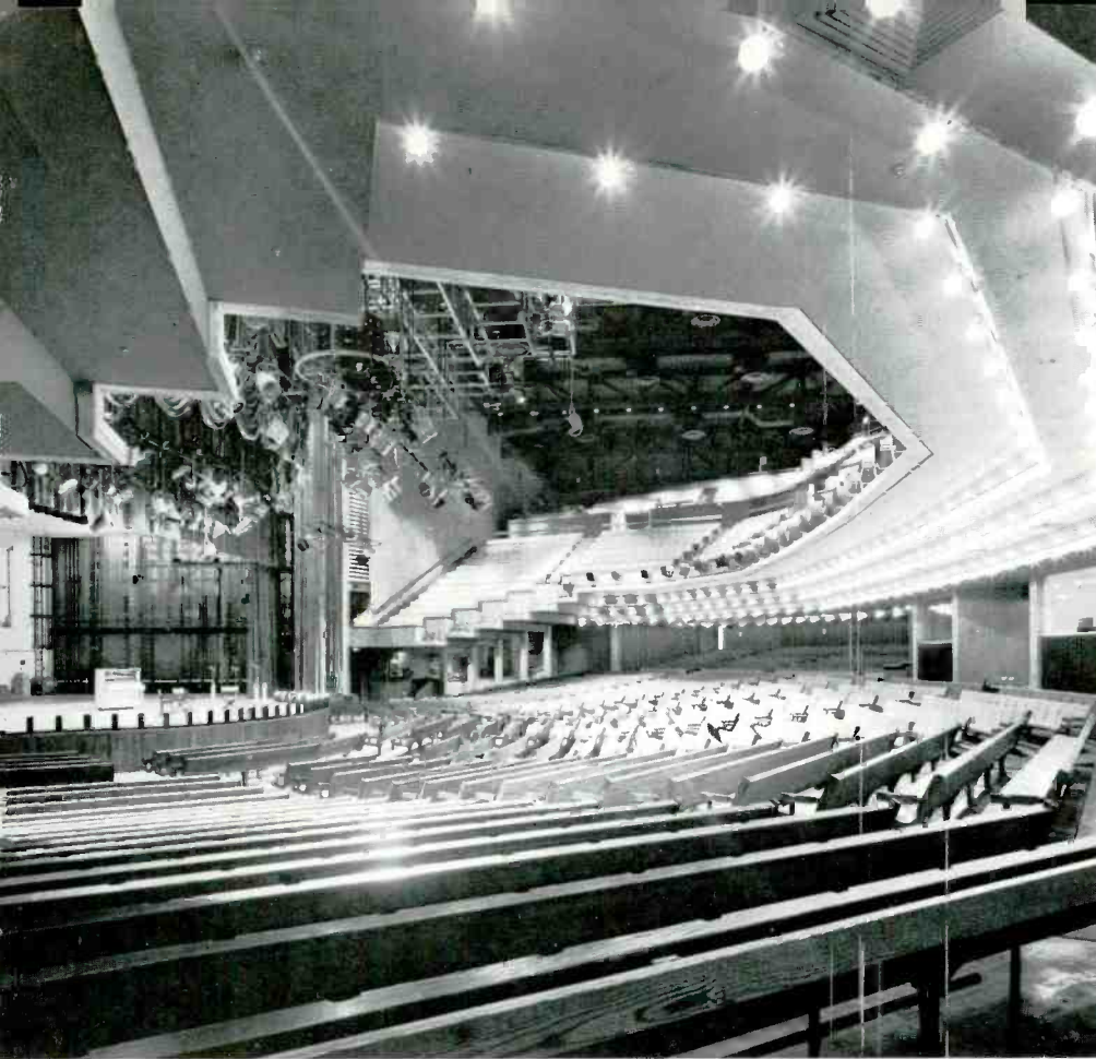
All but the very last eight rows of seats on the main floor are in direct line of sight of the central speaker cluster. (photo by Gordon H. Schenk, Jr.)
