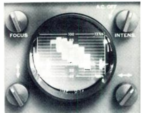
Figure 4: Waveform monitor colorbars display of "75% bars" (the first, white, bar is of 75 IRE units intensity) of 100% saturation (modulation level of the 6 intermediate bars of color between white and black). Color reference burst, S.C. precedes each horizontal sweep and appears here twice (the second time is preparatory to the next horizontal sweep of the bar's test signal).
