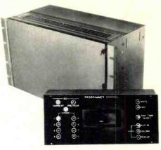
programmer is, in effect, a digital computer including the necessary interface electronics to communicate with the control elements within the console, and also containing sufficient memory capacity to store and retrieve all mixing control data.
