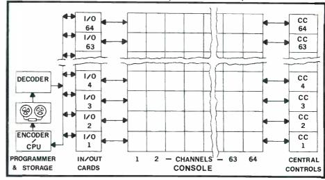
No. 3 level, mute, solo and group assignment sub-section." The 12 bit address defines the systems capacity as 4096 sources of data, each source having a 16 bit data capacity.
