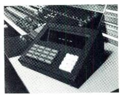
recorded on one track of the multitrack tape. To facilitate working with existing systems, including VTR and Film, the internationally accepted SMPTE edit code has been adopted. This code identifies any point on the tape in terms of an 8 digit number which reads Hours, Minutes, Seconds and Frames.
