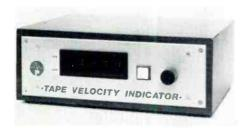
Ten-turn vernier speed control provides the fine adjustment capability to shave time off a "61 second" spot, sharpen a flat, compensate for off-speed tapes, and accomplish any number of special effects, such as flanging and delay. Front panel button switching selects between fixed (crystal) and variable speed.
