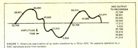
produce numbers which are both accurate and very large. 16-bits produces 2<sup>16</sup>, or 65,536 different descriptions of possible amplitudes; the dynamic range of the conversion is therefore 96dB. Similarly, the noise is one part in 65,536, or 96dB below clipping, and such errors produce a distortion of about .0015%.
