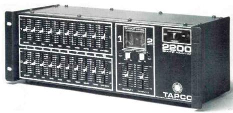
single-ended inputs and outputs can be used in any combination. That means the 2200 can be used in place of transformers between pro and semi-pro equipment. Separate EQ In/Out switches allow each channel of the equalizer to be programmed independently. And the 2200's VU meters can be set for any reference level with the calibration controls, accessible through the front panel.
