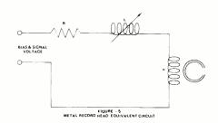
frequency. A third requirement exists if the head is tuned at the bias frequency. It must resonate with the bias coupling network.
