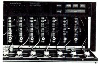
So is routine maintenance. Remove two front panel screws and the meter section swings down to give you immediate access to the EQ, bias, and level controls.
