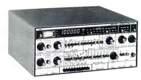
RMS, an autoranging digital frequency counter, a spectrum analyzer, a wave analyzer, a band pass, band reject, high pass, low pass filter and a four channel digital memory to store response plots.
