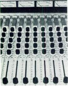
Designed primarily for recording studios, Interface Electronics mixers are also now increasingly being used in sound systems because of their flexibility, ruggedness, reliability and portability. Track masters are used as submasters (up to eight with the Series 300) and the mixdowns provide for feeding each submaster to right or left or any shading between, with mixdown masters used for right and left sound system masters.
