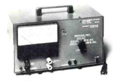
Specifications: 20-20,000 Hz, <0.1 dB. Useable to 20 kHz. The analog output (recorder) jacks provide 0 to +1 volt output for 0 to full scale, all ranges; accuracy and linearity <0.5%.
