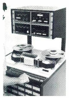
The new machine operates at speeds of 7½, 15 or 30 ips and is capable of handling 14-inch reels.
