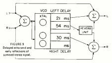
Figure 10 shows, a stereo delay unit with four outputs connected to delay reverb and adds a delayed pair of early reflections (which could also be criss-crossed and panned back in quad).
