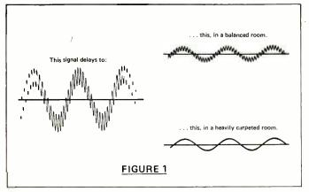
$*T_{60}$  is defined as the interval in which sound pressure decreases by 60 dB after a steady-state sound has been abruptly shut off.
