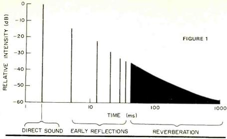
iar, common ground of acoustic space. In addition, digital delay can create a variety of special effects and enhance the sound of single performers or small ensembles.
