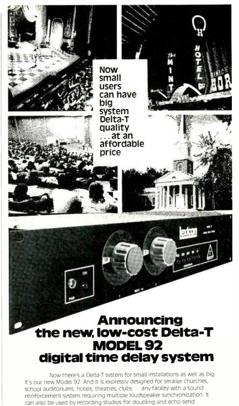
Wherever you install the Model 92, you can do it with confidence. At a price competitive with even run-of-the-mill systems, the new Model 92 delivers the same unsurpassed audio quality and performance reliability that have made Delta-T the standard of the industry. Noise and distortion are held to less than 0.1% Dynamic range is better than 90 dB. Signal delays are selectable to 120 ms.
