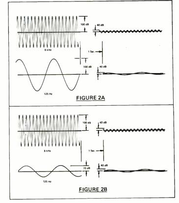
non-flat. By contrast, the balanced room of Figure 2a has a flat direct sound, an unchanged tonal balance for the entire decay period and both frequencies reach inaudibility together. Clearly this is a much more desirable situation than the heavily carpeted, heavily equalized room of Figure 2b. The wonderful result of this balanced room is that a speaker that is flat in an anechoic chamber will sound flat at the mixer's ears, too, *without equalization*.
