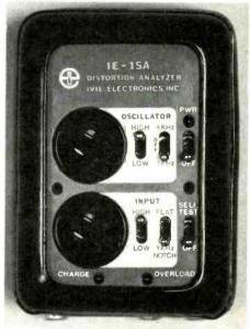
Built into the IE-15 $\Lambda$  is an ultra-pure sine wave source having selectable frequencies of either 1 kHz or 4 kHz and output voltages adjustable over a 60 dB range. In addition to distortion testing, the oscillators can be used in troubleshooting applications, or in any other task requiring a stable, clean signal source. Professional perfection in most exacting microphone applications
