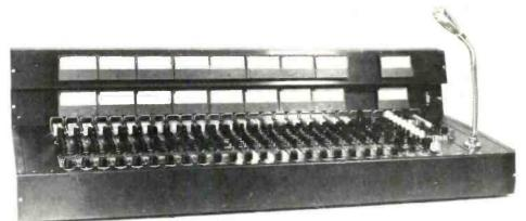
tave graphic equalizer. Mainframe includes 18 four-inch lighted VU meters having industry standard response, ultra reliable regulated power supply, and masters. Construction is entirely modular and plug-in and uses new high-slew rate internally compensated plug-in integrated circuits throughout. Numerous options are available in both input and output sections, and mainframes may be ordered with less than a full complement of input modules and more modules added later.
