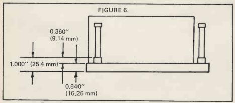
Front elevation view of Ampex head plate and fixed guides. Figure 6.
