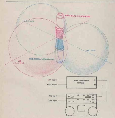
Figure 2: A simplified block diagram of a modified MS/XY recording system using two separate phase and amplitude matched microphones. The mid signal is picked up using a true cardioid pattern, and the side(s) by using a figure-of-eight pattern. By varying the controls the width of the sound source can be varied through a 0 to 65 degree arc.
