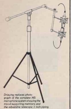
Photograph 2, the support system was designed around an Atlas SS-2 speaker stand. A 10-foot extension pipe can be purchased from an electrical supply house. It is advisable to shock mount the microphones, since the tubing has a
