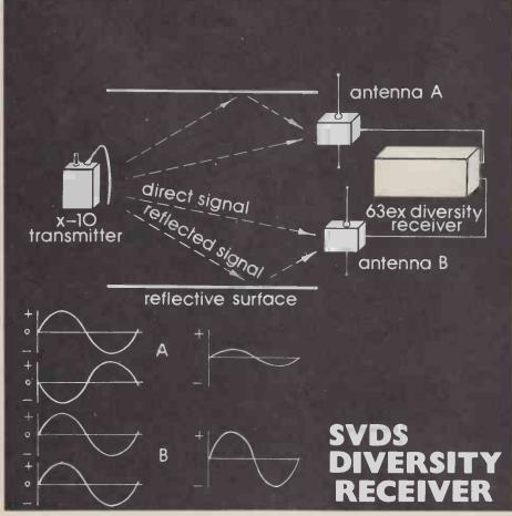
In actual performance usage, this Diversity system guarantees a minimum 100 yard (typically 500 feet) fade-proof range, with the ultimate system audio specs the same anywhere within this area. (The actual distance measurement might be the locus of the two antennas — which are dipole type antennas, normally taped to the top of a guitar amp, either side of the stage.)
