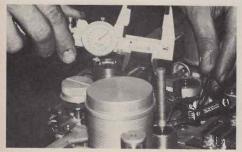
Studer pinch roller-capstan clearance adjustment. Figure 11.
