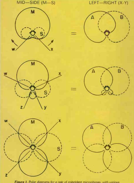
Figure 1. Polar diagrams for a pair of coincident microphones, with various directional characteristics, showing MS to XY transformation due to the matrixing of a sum and difference circuit.
