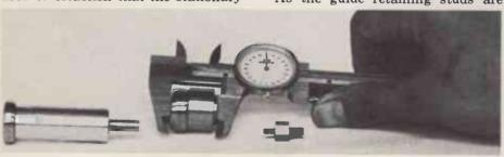
Ampex rotating guide height measurement.
