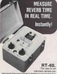
cise reverb time measurement in instant real time digital readout. No more chart recorder or time-consuming chart re-corder analysis. The RT-60's integrated circuitry incorpor-ates a one-third octave band pass filter system with frequency centers on 250,500,1000,2,000, and 4,000 Hz. It operates on self-contained ni-cad batteries. Mounted in a rugged carrying case, the RT-60 weighs only 3.5 pounds. The dealer net cost, FOB San Diego, is just \$460. Write for your free technical
