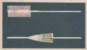
The next photograph (Figure 3) illustrates the action of a fully saturated transmission system which clips off the leading edge of the sharp wavefront. As we explained, in the demonstration system the long spike is definitely a part of the wave train, and is necessary to reconstruct the burst.
