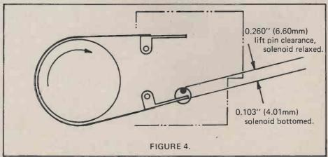
Top view of Studer reel motor and brake assembly showing critical dimensions.
