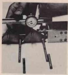
Ampex tape lifter mechanism solenoid travel adjustment.
