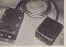
The author's portable MS/XY matrix system showing separate output module featuring a bypass switch.
