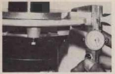
Ampex reel platform height measurement. Figure 3.
