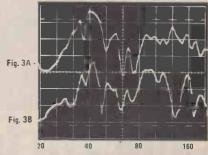
Figure 3A: Long room mode response, 20-200 Hz., sine wave sweep "8"
