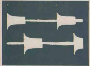
Figure 4 is a close view of the input to the compressor and output after the expander when the leading edge is clipped by the transmission medium. Without the steep wavefront transmitted to the expander there is no way to recreate the original tone burst. If any transient sound such as piano,
