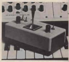
Modification of the sound is realized as the joystick is moved in any direction on a 360 degree horizontal plane. The X axis or left/right of center movement controls pitch bend. The 'Y' axis or forward/backward movement is assigned to filter sweep. Switches are included to allow the player to
