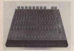
The input modules feature a  $4\frac{1}{2}$ " conductive plastic slide fader; 6 knob, 3 band parametric equalization; 8/16 track assignment buttons; post echo send; monitor send control; 2 cue sends; solo button which allows stereo panning when engaged; a mic/line switch; and an attenuation switch of -10 or -20 dB.
