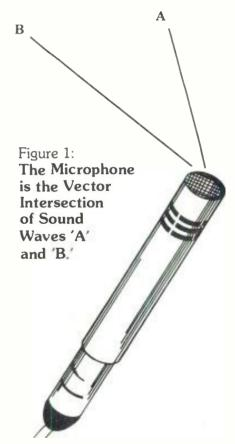
It is helpful to consider how this interference effect acts down through the audio spectrum. Comb filter interference can radically affect the overall frequency response even though the system components are flat. Let us assume that a microphone diaphragm is actuated by the combination of two signals, a signal direct from the mouth of one talking, and the same signal delayed 0.1 millisecond. Without the
