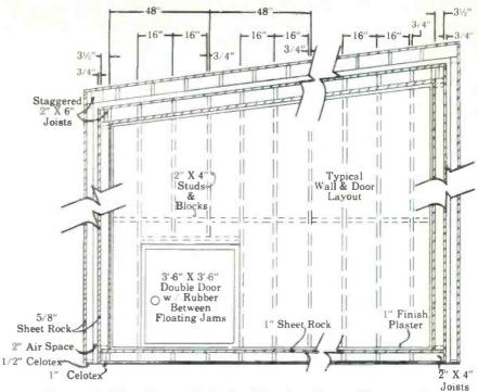
Figure 6: Elevation of Interior Showing Door Placement
