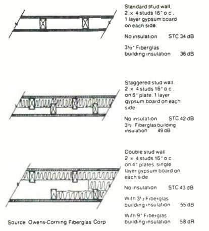
Figure 3: Comparison of Stud Wall Construction and Transmission
