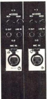
From the discrete microphone preamplifier, equivalent input noise is -126dB (weighted). With one input assigned to one output buss, signal-to-noise is 76dB (weighted).
