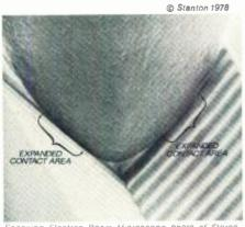
Scanning Electron Beam Microscope photo of Stereohedron® stylus, 2000 times magnification, brackets point out wider contact area
