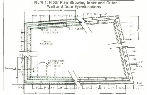
enough space, the next step is to design a floor plan (Figure 1). When laying out the sides of the room none of the walls should be parallel or even near to parallel. The ceiling should not be parallel to the floor. This is very important if the room is to have maximum random reflections and a smooth decay. It's at this stage that a bit of math should be introduced:
