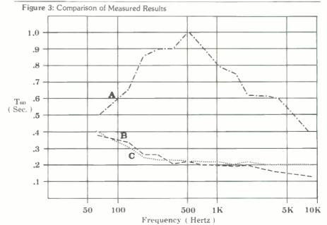
seconds. This way, you are certain not to run off the bottom of the graph if later measurements have lower T60s and you wish to overlay the new curves on the old. Also, changes in the reverb curve will be shown in their proper perspective, that is, in relation to the total amount of T60.
