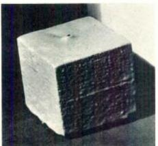
Latex Coated Fiberglas Insulation Block
