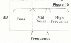
all the ingredients for generation of comb filter perturbations of response in the crossover region. The same process is active at f2 between the midrange and tweeter units. Actually a narrow band of frequencies is affected, the width limited by relative amplitudes of radiations from the two adjacent units. The steepness of the crossover curve determines the width of the frequency range affected. This is a highly
