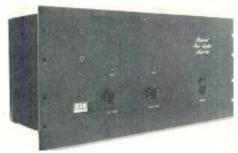
The 600 retains these BGW features: Modular design with massive heat sink assemblies; redundant output stages utilizing ten 150 watt complementary transistors each; sophisticated loss-offeedback clipping indicators; high speed 15 MHz Op-amp front end; independent front panel gain controls; separate signal and chassis grounds and rugged, heavy-gauge steel construction.
