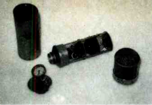
The ubiquitous U-47, showing the VF-14 suspension system used to minimize mechanically generated harmonics.
