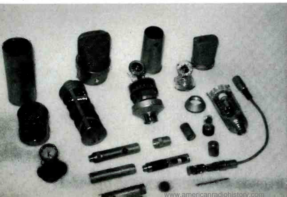
THE FAMILY OF NEUMANN TUBE MICROPHONES. Top row: The large capsule models, left to right, top row are the U-47, M-49B and the U-67. Small capsule microphones appear top to bottom, center; KM-66 (next to it is a Z-29, 10dB pad), the KM-84, and the U-64us. Photo is from the author's collection.
