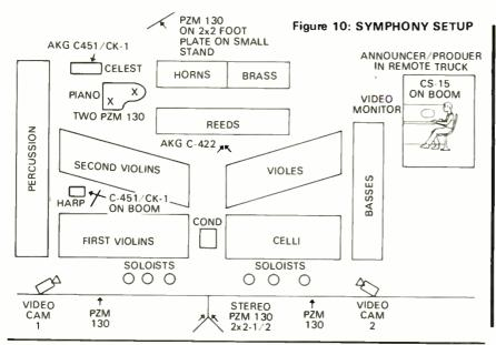
the van and was able to observe the action on stage on a pair of video monitors being fed by a pair of cameras left and right. The announce mike was an Electro-Voice CS-15, chosen for its crisp sound, and when used with its wind screen is relatively immune to popping.
