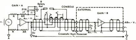
Figure 6 - Forward Referenced Amplifier
