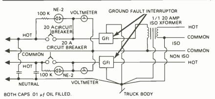
FOR SINGLE PHASE 210 VOLT POWER SEND THE COMMON AND THE NEUTRAL ARE BOTH TIED TO THE NEUTRAL BUS AT THE MAIN POWER SEND POINT.
