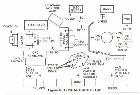
hyper-cardioid pattern and smooth response independent of working distance makes them an ideal choice for live radio production. They are also, in the Electro-Voice tradition, nearly impossible to destroy. In addition, their hyper-cardioid response makes them less sensitive to leakage from other instruments which is a particular problem in a loud rock set up.
