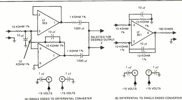
Figure 5: CIRCUITS FOR CONNECTING UNBALANCED TEST EQUIPMENT TO BALANCED DUT'S
