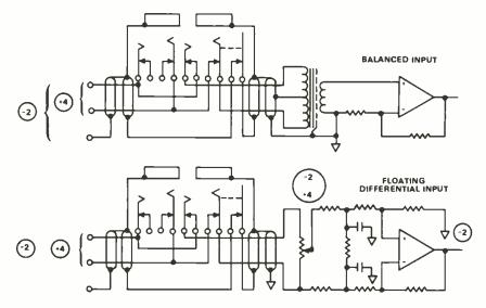
Figure 9 - Isolation Inputs with Bi-Level Patching
