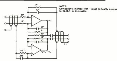
Figure 7 - An Electronic 6 dB Step-Up Output with Forward Referenced Isolation and Differential Input
