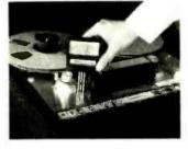
The Tentel Tape Tension Gage is designed to diagnose problems in your magnetic tape equipment. Virtually all recorder manufacturers use and recommend the TENTELOMETER® for use with their equipment.
