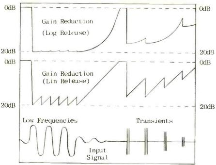
Figure 2 — Pictographic representation of Log Response Shape vs. conventional Linear Release. Note that, although the overall release rates are similar, the Log shape produces significantly less gain modulation on low frequency material (lower distortion), and on recurring transients (less pumping and envelope distortion).
