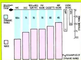
To help you overcome these restrictions you need a compressor/limiter which can 1) compress the dynamic range of a signal down to fit that of a more restricted medium and 2) maintain an overall maximum level (or limit).
