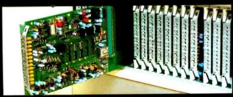
Single card audio electronics contains record, reproduce, synchronous and timing circuits
