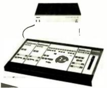
Sony broadcast U-matic videocassette recorders to store the digital information, the editor allows the sequencing and combination of varied material for a finished product with extremely accurate, undetectable edits. The preview function of the DAE-1100 makes editing fool-proof, and lighted buttons which flash in sequence show the order of operation.
