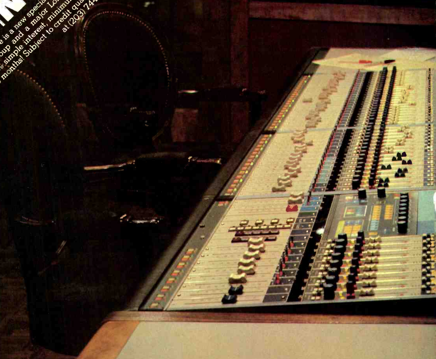
Picture shows Model 8108 console fitted NECAM Computer Mixing System at Studio B, The Village Recorder, Los Angeles. Their Studio D is equipped with a Neve Model 8078 and NECAM.
