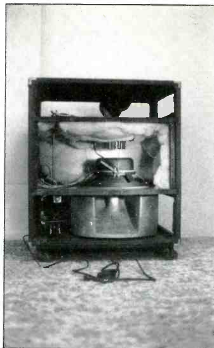
Figure 11: Customized Leslie Cabinet with tandem bass and treble rotors. The stock treble horn is driven from a tandem drive shaft coupled to the lower bass rotor. An Atlas P.A. driver is connected to the treble horn, while a JBL D120 12-inch speaker handles the lower frequencies.
