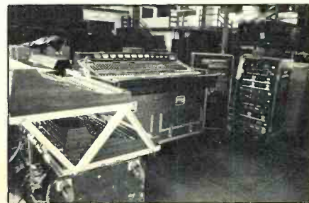
Figure 6: Piggyback stand for M-916 submixers (left), PM-1200 front-of-house mixer, and processing racks
