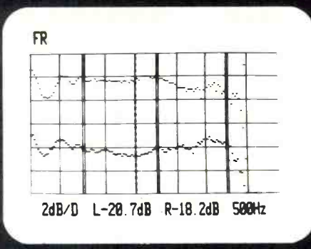
From left to right: Third Harmonic Distortion, showing a decrease in distortion as the signal level is reduced to residual noise; two channels of Frequency Response on a scale expanded to 2 dB per division; and Azimuth Misalignment, for which the tape machine heads are adjusted for minimum vertical bar height.
