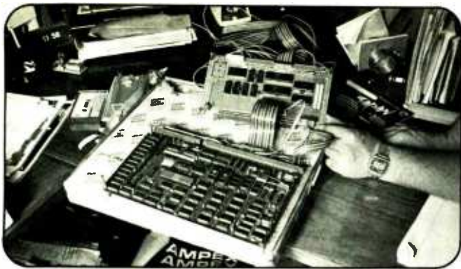
Bryan Bell's custom-designed 16-bit computer controller/interface for the Apple II+.
