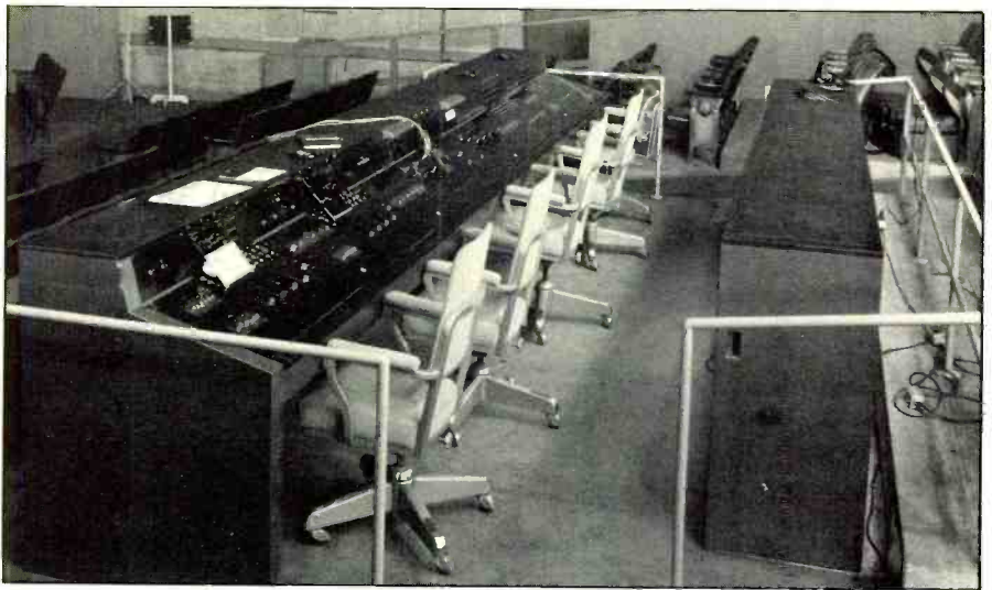
Westrex re-recording console built for the six-track mix of "Oklahoma!" and equipped with 96 inputs divided into 16, six-track groups.
