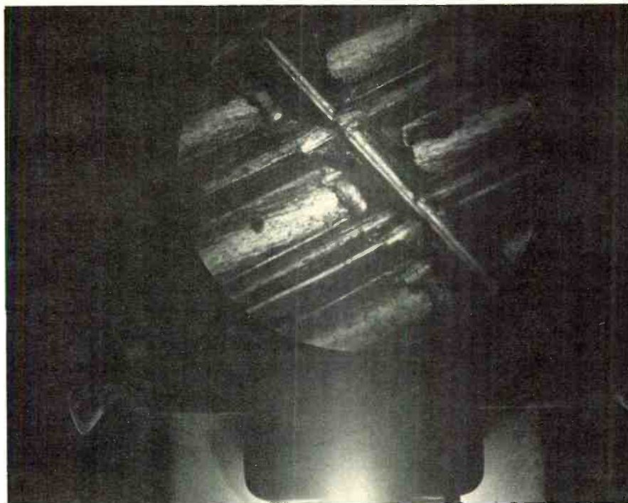
An optical comparator magnification of a scratch across the grooves on an aluminum disk. (Photo by Bill Storm.)
