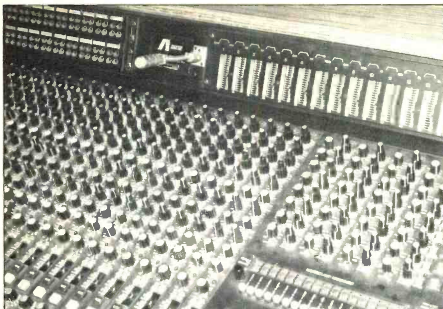
Figure 1: Gamble HC40-24 house console, with built-in 16-ladder spectrum analyzer for measuring system response.
