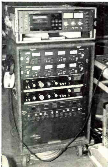
Figure 3: House electronics rack with Showco crossovers, dbx compressors, and MICMIX Master-Room reverb.
