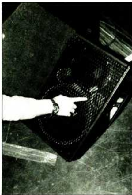
Figure 8: Meyer UM-1 stage monitor slant houses a single 12-inch bass driver, and a conical horn mid-range.
