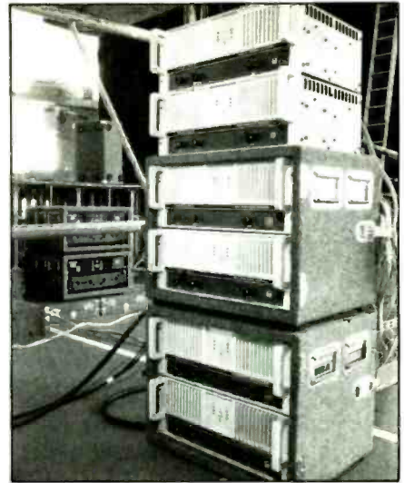
Crown PSA-2 amps powered the main system, while Ashly FET200 and QSC Series III amps served as backup units.
