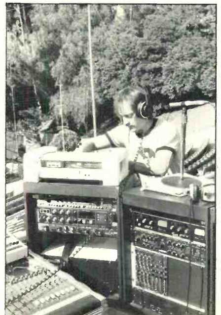
Figure 5: House mix electronics racks with comprehensive patching access includes a White RTA.
