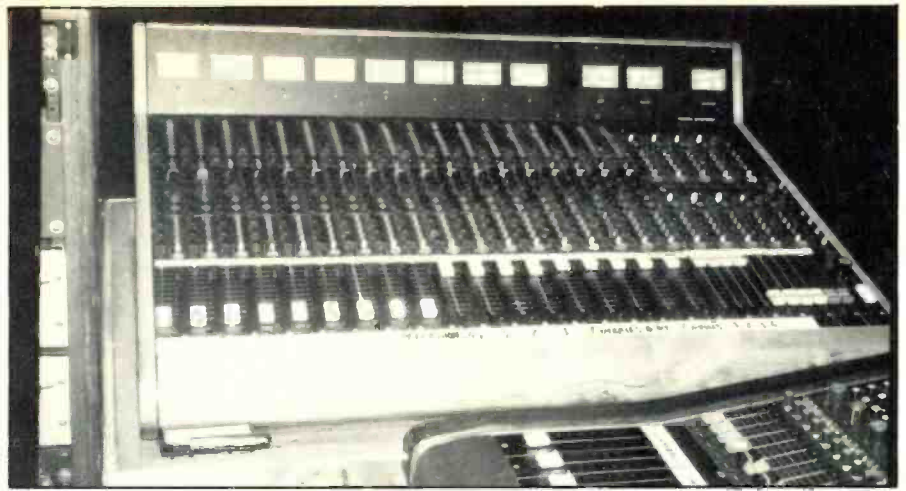
Figure 6: Additional house mix inputs were handled by an auxiliary 18-channel Trident Trimix submixer for drums and percussion.
