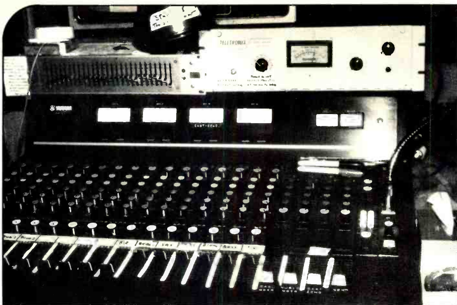
Custom-built 53-input house mixing console in NBC's Studio A provides a wide variety of subgrouping and output options.
