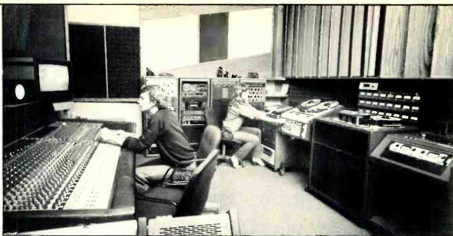
EFX System's video sweetening room features an AMEK 2500 automated console, BTX Soft Touch synchronizer, MCI JH-24 multitrack, and MCI JH-110B video layback.
