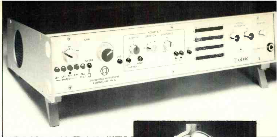
Calrec Mark 4 Soundfield Microphone with cover removed (right), and control unit, capable of capturing a total 360-degree soundfield.
