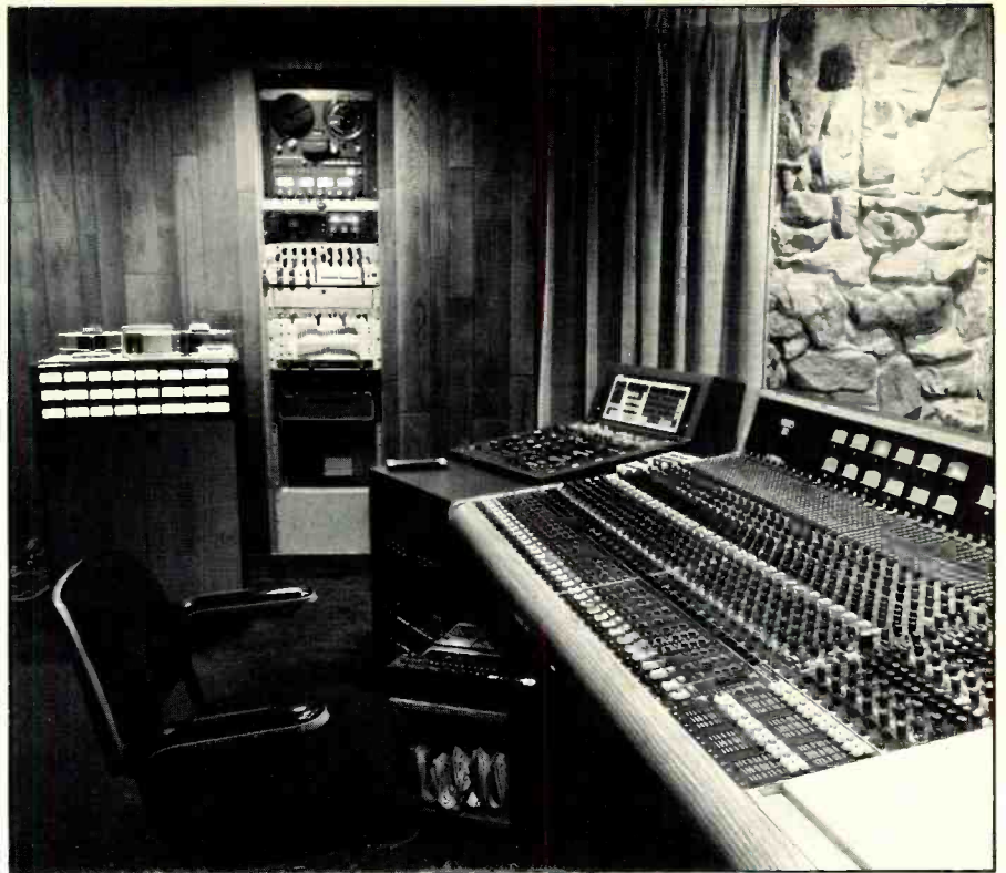
The Warehouse control room houses a Trident Series 80 console, Ampex MM-1200 multitrack and ATR-100 mastering machines, plus a full rack of outboard equipment.
