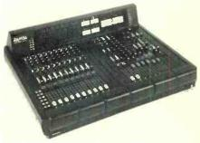
Input channel signals can be routed through any one or combination of the group output channels to the L-R master output channels, or routed directly to the pan control. In broadcast applications, such a format allows up to three simultaneous stereo mixes. A mono ouput master provides a simultaneous mono output with the L-R master outputs.
