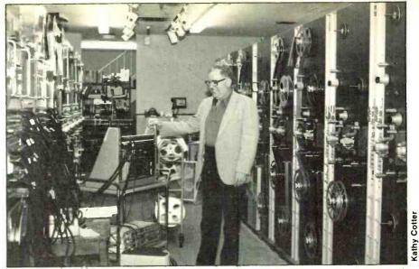
Head of TBS Post-Production Sound Department, Tom McCormack, in Dubbing 5's machine room, which houses RCA PM-85 and -86 mag dubbers and recorders, plus portable Dolby M16H noise-reduction rack.
