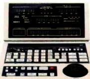
Practices for Digitally Controlled Equipment." Which means the interfacing problems between video, audio and film equipment will be problems of the past. This Sony "Sync Master" synchronizer has a built-in distributed intelligence network that makes it able to talk to an entire universe of diverse machines developed by diverse manufacturers.
