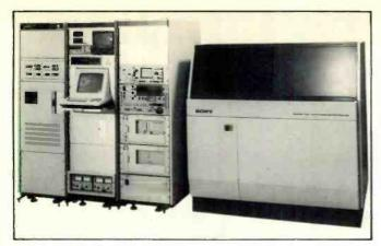
A Sony DMC-1100 Disc Master Code Cutter; Terre Haute will be equipped with two such laser cutting systems.
