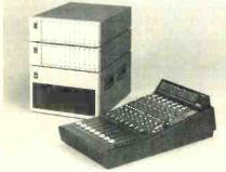
The system's processor unit connects directly to Sony digital equipment, and is designed to mix 16-bit linear quantized digital signals. The unit accepts eight digital input channels and provides three separate digital outputs: a two-channel main output, two-channel sub-output, and eight-channel direct output. The utilization of the control unit with the processor permits up to eight digital signals to be
