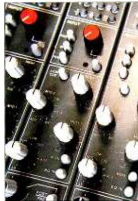
Equalizer combines continuous control and detents for reset-ability
