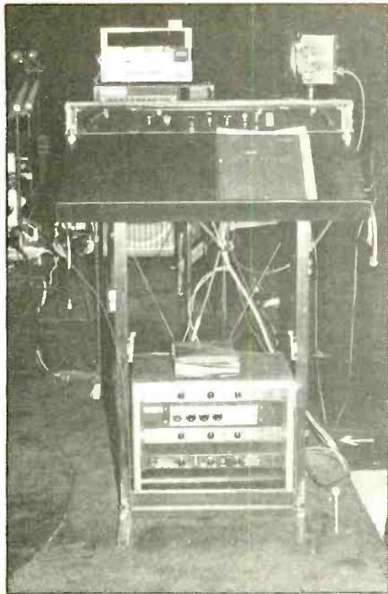
Conductor's control center and music stand, with Auratone monitor, BGW amp and Shure mixer.
