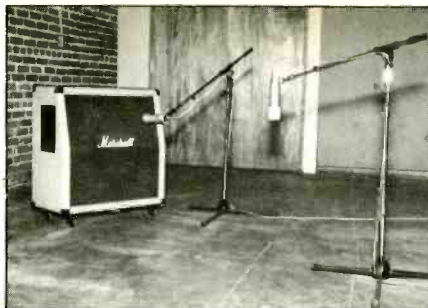
Marshall stack for "Gypsy 68" — close mike is an EV RE-20, and distant a Neumann U87 (sometimes used instead of an AKG C452).
