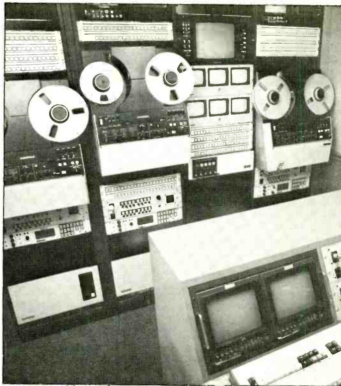
The Video Production Area (left) house a Grass Valley 300-A-3 Series video switcher, and an Ampex ADO Digital Video Effects Unit; the Videotape/Chyron Graphics Generation Area (right) serves as home for Ampex VPR-2B one-inch, C-Type videotape machines, with full timecode and Slo-Mo capabilities.
