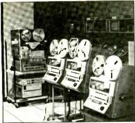
Four Sony BVU-2000 VTRs provided main and backup video replay plus PCM digital audio playback at the satellite uplink site.
