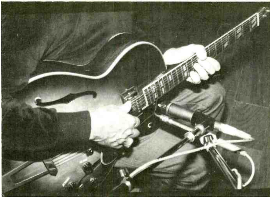
Guitar microphone technique for "Tune for Tal" — a Gibson 175 played acoustically and covered with a combination of a Shure SM57 and AKG C452 mounted close to the bottom of the fret board, to pick up the sounds of the low and high strings, respectively.
