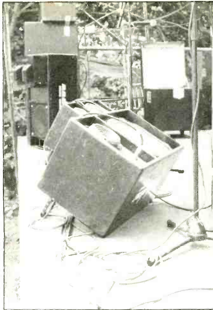
Figure 5: Modular's stage monitor cabinets consist of a two-way non-slant box housing a 12-inch speaker and a one-inch driver. An additional auxiliary HF section is removable.
