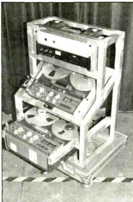
Front and rear views of custom-designed carrying frame to hold two Revox B77 two-tracks, and companion dbx Model 157 noise-reduction unit.
