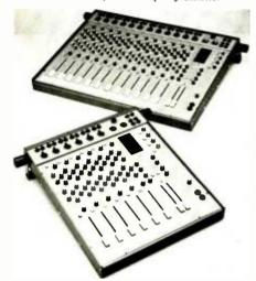
The microphone/line input switch on each input channel selects either a low or high impedance input. Both are electronically balanced, and together cover the range -55 to +10 dBm, with 25 dBm overload margin. Three-band EQ offers  $\pm 15$  dB of midrange sweep control from 330 Hz to 6.5 kHz.
