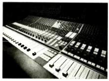
Mainframes for the new system will accept from eight to 56 mono or stereo inputs. Special panning and width enhancement circuitry is provided to simplify the matching of stereo perspective with video. Up to six stereo or 12 mono auxiliary sends may be provided, along with as many as eight stereo IFB/Cue select matrices. (These features are said to speed and simplify the creation of the multiple cue and communication feeds required for stereo teleproduction.)
