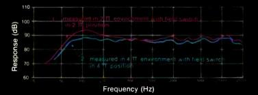
Monitor response will always vary from a 2 pi steradian environment (wall or soffit mounting) to a 4 pi steradian environment (free field or console mounting). The Fostex RM-Series Point Source Monitors provide a front panel Field Switch to provide the same response in both environments.
