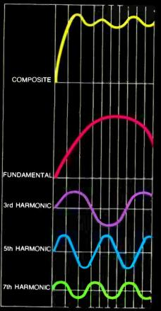
The completed figure to the left is a composite illustration of how a transient pulse looks when the fundamental, 3rd, 5th, and 7th harmonics are all in phase.
