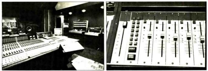
The first production GML Automation System installed to a 48-input Neve 8108 console at Conway Recorders, Hollywood. Shown right is a close up detail of the master select panel and a section of the input fader bank.
