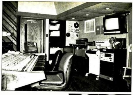
Music II's recording equipment (above) includes a Harrison 4032C console, MCI JH-24 multitrack, Studer B67 stereo decks, and a full collection of outboard signal processors. The Harrison board (right) features 40 input channels and 32 routing busses.
