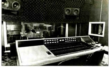
Treasure Isle's control room features a 32-input Trident Series 80 (with additional A-Range input modules), Studer A80 multitracks and half-inch mastering machines, plus a large collection of outboard delay lines, and reverb.
