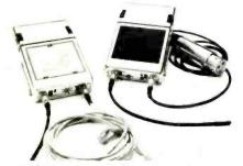
All battery-operated equipment incorporates a DC-DC voltage converter that maintains the operating voltage of the unit as the supply voltage drops, thereby avoiding audio distortion and carrier frequency drift. Powered by three AAA batteries, the units are equipped with special compander circuitry, crystal-controlled oscillators, and select features which vary from model to model. SENNHEISER ELECTRONIC
