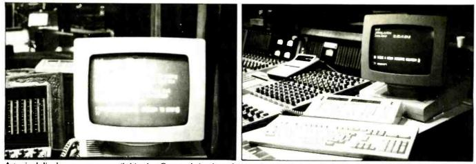
A typical display screen menu (left), plus Conway's keyboard control surface and video display unit. The keyboard (shown in greater detail below) enables labels and annotations to be added to the mix data, and provides enhanced system control.
