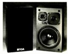
The two-way 265-ME is said to be ideal for either primary or secondary reference applications, and handles continuous program at 75 WRMS. Response is a quoted 60 Hz to 20 kHz. Components comprise a 6.3-inch woofer, and a 1.2-inch soft dome tweeter with diffuser.
