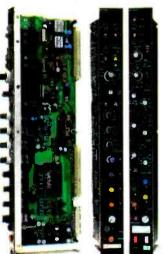
Basic input modules feature 3 or 4 band EQ, microphone/line inputs, 5 pre/ post-fade auxiliary sends, and channel overload indicators. Options include transformerless mic preamps on a subcard, separate transformerless TAPE input for remix, stereo input modules, stereo EQ, internal stereo X-Y/MS active matrix, stereo blend control, dual line inputs, variable HP and LP filters, user defined panel switches, and the list goes on. Listen to the quiet. The
