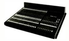
Each input offers pushbutton selection of tape signals and electronically balanced mike and line. Phantom 48-volt power is individually switchable for each channel, and a phasereversal switch is included for line and mike inputs. Each input channel has its own direct output and insertion point for external signal processors. A sweepable three-band EQ section with an on/off switch and an 80 Hz highpass filter is also included.
