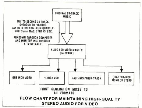
automation process, we were able to preserve the continuity of the mixes and complete the project in half the time. Also, first-generation mixes from the audio-for-video multitrack master can be passed across to any format needed for the job, the result being a
