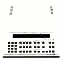
Features include pre-programmed loops with optional preview; pre-programmed or "hot" Master or Slave record in and -out; offsets up to 24-hours; selectable interlock speed and type; synchronization accuracy within 333 microseconds; a system memory; plus standard transport control and autolocation capabilities.
