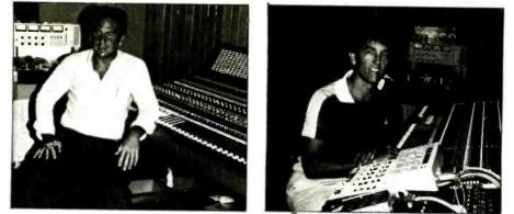
Mix Magic chief engineer Gary Fradkin (*left*) and owner Jim Corbett at the facility's 40/24 Trident-TSM console, linked to Otari MTR-90 and MTR-10 tape transports via an Audio-Kinetics Q.Lock 3.10C synchronizer.
