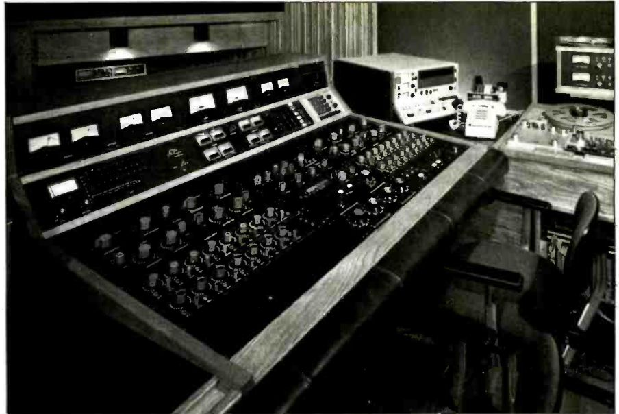
The custom-designed disk mastering console at Bernie Grundman Mastering is built entirely from discrete components. Tape replay is from a rebuilt Scully deck; playback from Sony PCM-1610 and Mitsubishi X-80 two-track is also available.
