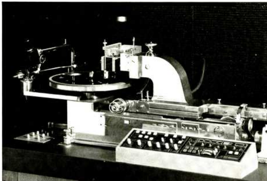
One of the two tandem Scully lathes, refitted with phase-locked motors, Sontec Compudisk computer control, and customized cutter-head suspension. The cutting head combines a Haeco magnet assembly with Westrex drive coils.
