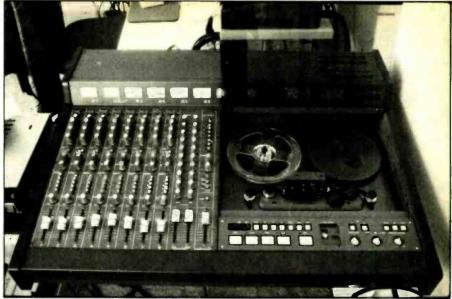
The Tascam Model 388 Studio 8 comprises an eight-input mixer and integral eight-track on quarter-inch tape deck with dbx noise reduction. Each input channel offers mike trim, three-band EQ, two effects sends, track routing and pan.
