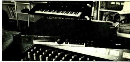
The Lexicon PCM-70 features 36 factory presets and 50 user registers, plus Dynamic MIDI for real time control via an external mod wheel and/or after-touch.
