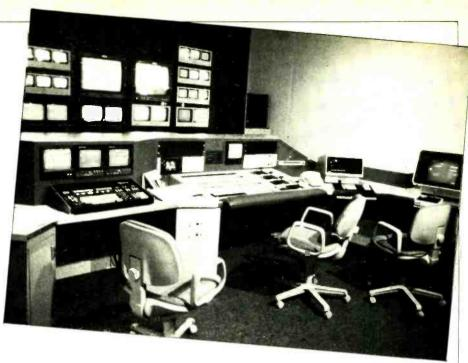
Close-up detail of the completed Video Production Control Room, showing the various Preview and Program video monitors, central switcher and routing panel, plus controls for a variety of graphics and visual special-effects units.
