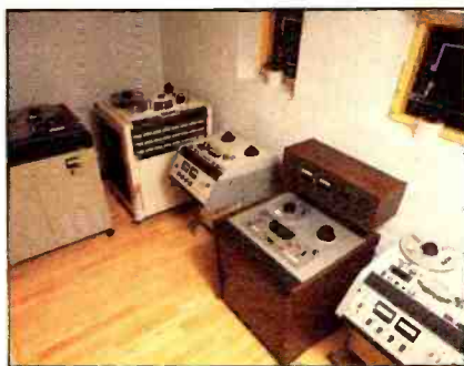
A dedicated tape machine room houses (from left to right) a Mitsubishi X-800 digital 32-track, an Otari MTR-90 24-track, MTR-10 2-track, Mitsubishi X-80 digital 2-track and a second MTR-10 2-track.
