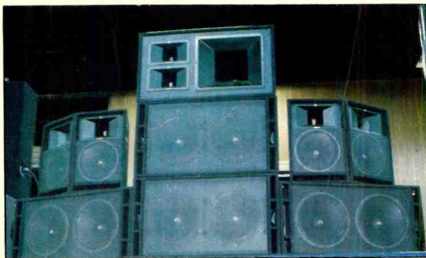
Figure 6. Each loudspeaker stack for the 6,000-person audience contained eight 18-inch PAS speakers, four 15-inch EV-15L speakers, a single Renkus-Heinz SSD-5600 midrange compression driver and six 2-inch compression drivers.
