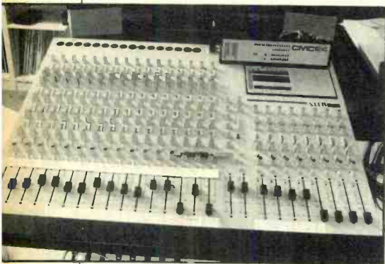
The 24-input CMC-24 console incorporates the CARS microprocessor-controlled routing and mute system.
