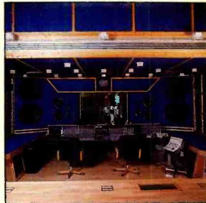
View from the performance area in Control Room A, which features a 56-input Audio+Design/Catrec UA-8000 console and custom 5-way monitoring system.
