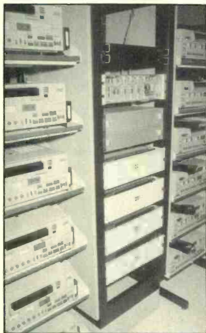
A central control module provides start, stop and rewind commands for dozens of slaved VCRs.
