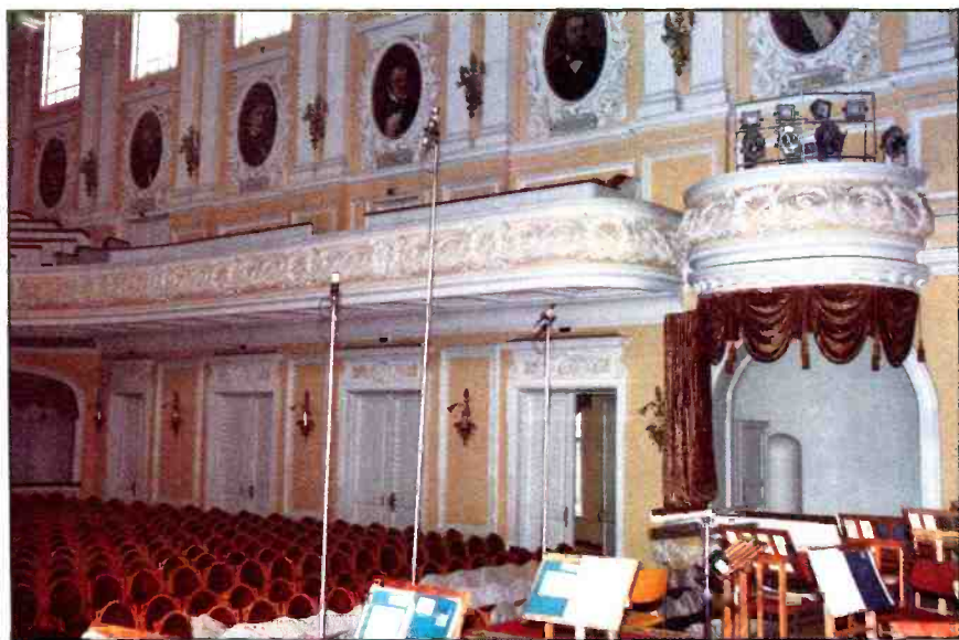
Photo 3. Reverse view, main microphone pickup. Center AKG C422. Violin and cello sweeteners AKG C414/P48.
