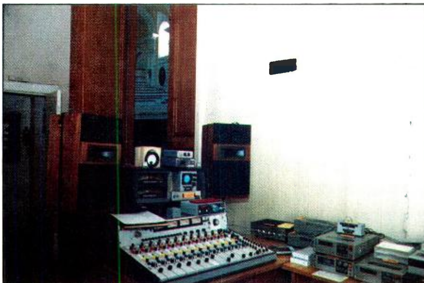
Photo 8. Off-stage "control room" setup modified Quantum mixing console, Norberg BCS-16 close-field monitors, Dorrough loudness-monitor meters, Sony PCM-F1 and Nakamichi DMP-100 digital processors, Audio Engineering Associates MS-38 DM MS matrix, Loftech TS-1 test set.
