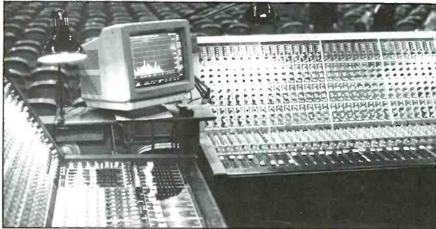
Figure 9. The house mix position features a pair of Clair's custom 32-input mixing consoles. The video monitor is displaying the output of dbx's RTA-1 real-time analyzer.
