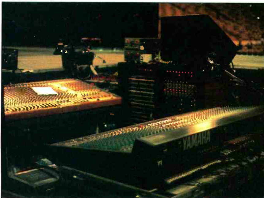
Figure 11. Stage monitor mix position, featuring a Harrison HM-5 and a Yamaha PM-3000.
