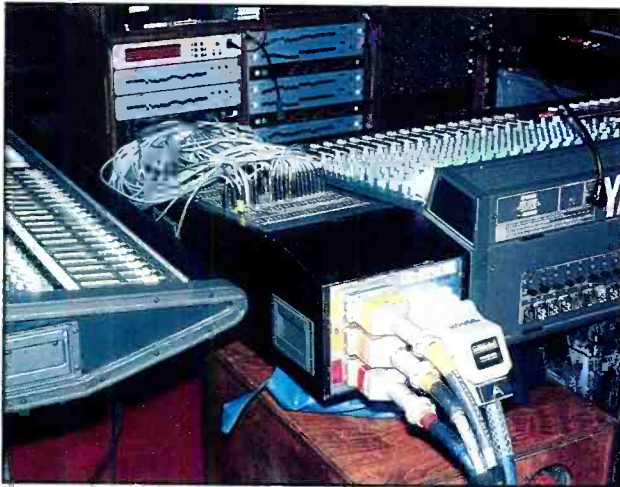
Figure 12. A pair of Yamaha PM-3000 consoles were used at the house mix position. Each console was custom-modified by dB to include an attached patchbay unit.
