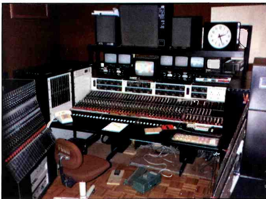
Photo 1. ABC Studio 59 where “Dolly” was mixed. Console is 36x16x4. L, M, R.
