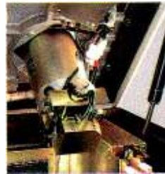
Reel motors that approach one horsepower are driven by pulse width modulation amplifiers to tape speeds up to 474 ips.
