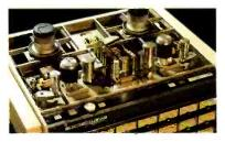
Otari isn't in the toy business. The MX-80 and MTR-90 sport 2" thick cast alloy deck plates. heavy duty swing arms, and motor shafts designed to handle the exceptional acceleration characteristics of these machines.
