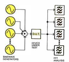
Figure 1. Block diagram of multitone test setup.
