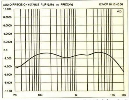
Figure 3. Frequency response plot obtained by measuring amplitude at stimulus frequencies only.
