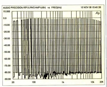
Figure 2. Spectrum of a 60-tone (1/6-octave) test signal.
