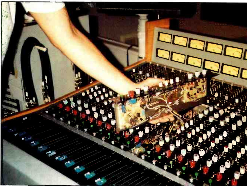
Individual modules can be removed and worked on while still connected and operating.
