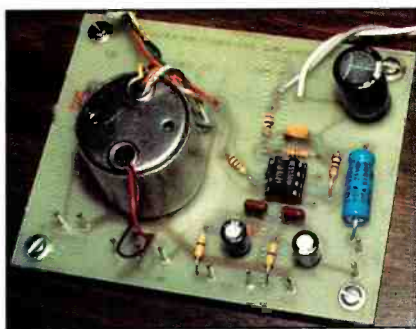
Mic pre-amp/line driver card, with Jensen transformer.
