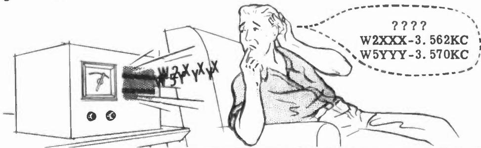
MORE RF STAGES ARE NEEDED WHERE SIGNAL FREQUENCIES ARE CLOSE TOGETHER
