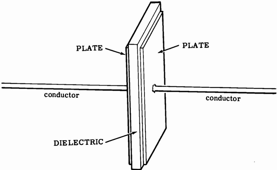
Plates are made of solid metal or metal foil.
