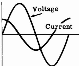
**CAPACITIVE REACTANCE** — The action of capacitance in opposing the flow of AC current and in causing the current to lead the voltage.
