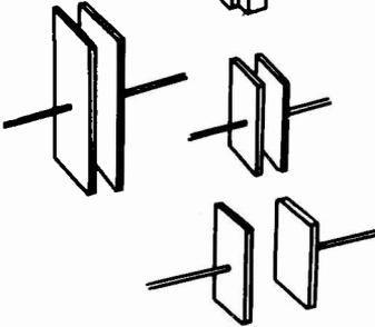
**CAPACITOR PLATES** — Metallic or metalized plates which can be charged.
