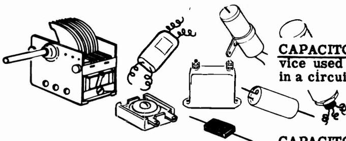
**CAPACITOR** — An electrical device used to supply capacitance in a circuit.
