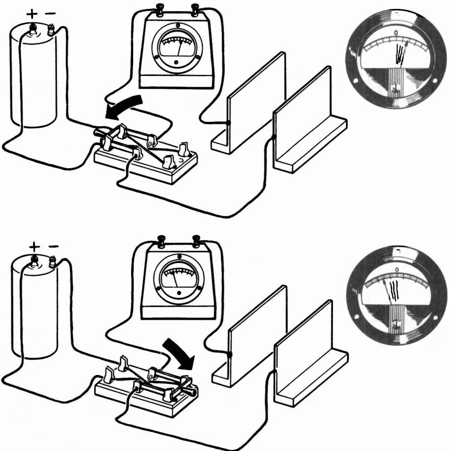
Suppose you switch the cell polarity fast enough so that at the instant the condenser plates become charged in one polarity, the cell polarity is reversed. The meter needle now moves continuously—first showing a current flow in one direction, then in the opposite direction. While no electrons move through the air from one plate to the other, the meter shows that current is continuously flowing to and from the condenser plates.
