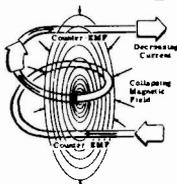
**INDUCED EMF** — A voltage which is generated within a circuit by the movement of the magnetic field whenever the circuit current changes, and which opposes the current change.
