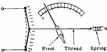
**HOT-WIRE AMMETER** — Meter movement based on the expansion of a wire heated by current flow through it. Used only to measure current.
