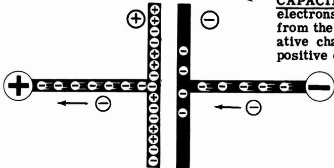
**CAPACITOR CHARGE** — Flow of electrons into one plate and away from the other, resulting in a negative charge on one plate and a positive charge on the other.
