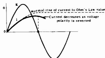
**INDUCTIVE REACTANCE** — The action of inductance in opposing the flow of AC current and in causing the current to lag the voltage; measured in ohms and symbolized by letter  $X_L$ .
