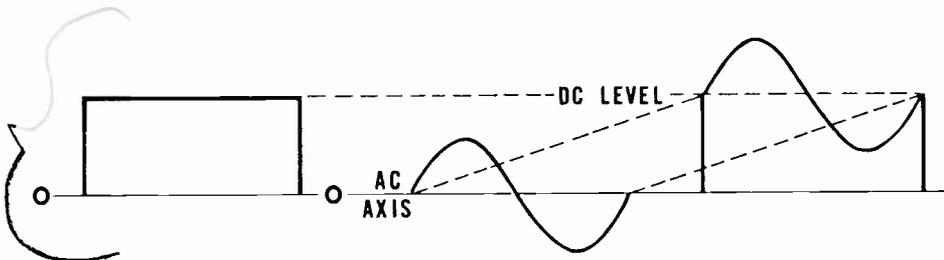
DC waveform + AC waveform = Superimposed AC waveform
