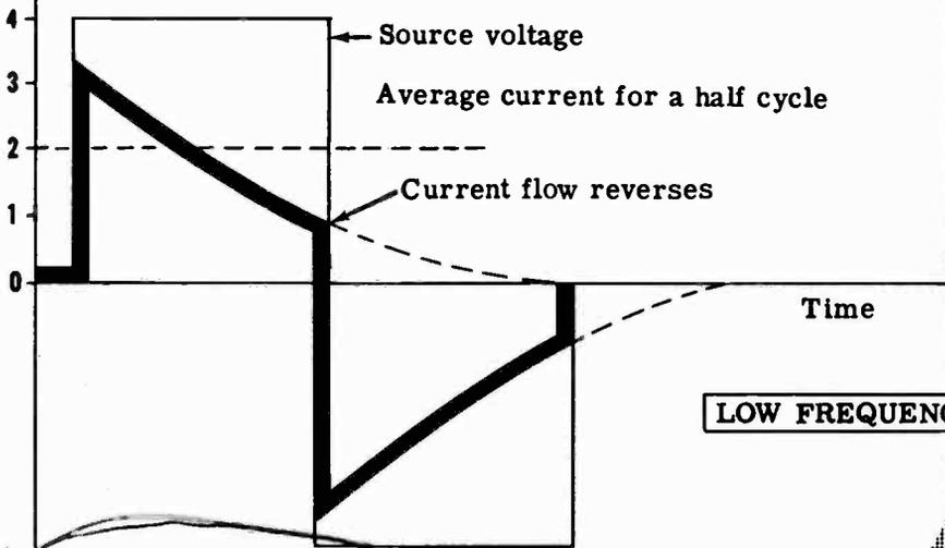
The lower the frequency, the lower the average current.
