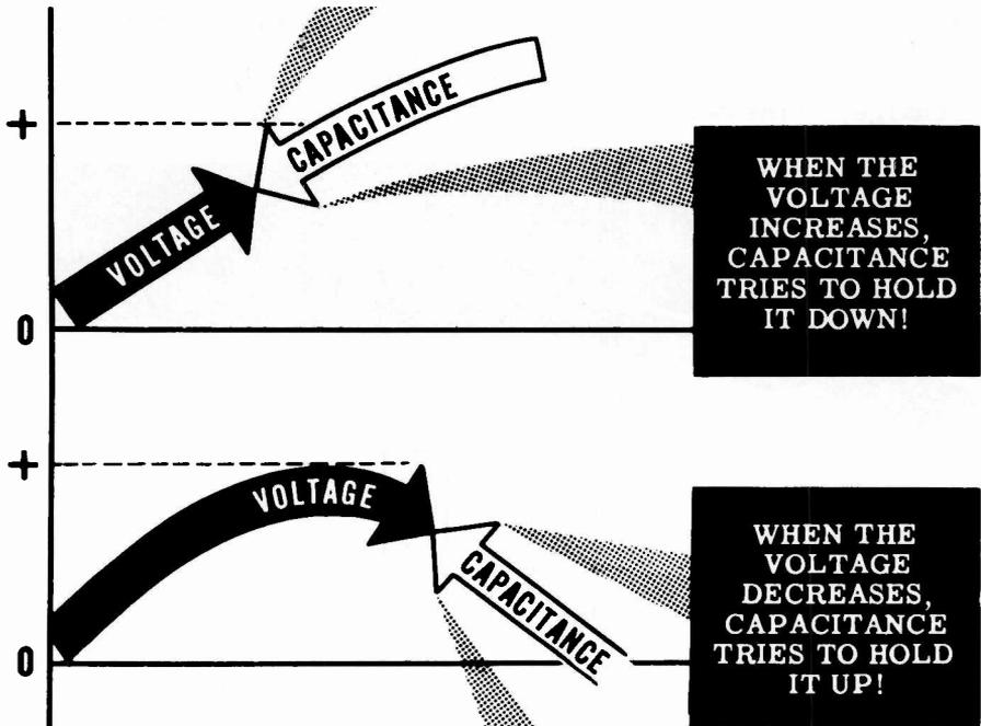
Because DC voltage usually varies only when it is turned on and off, capacitance affects DC circuits only at these times. In AC circuits, however, the voltage is continuously changing, so that the effect of capacitance is continuous. The amount of capacitance present in a circuit depends on the physical construction of the circuit and the electrical devices used. The capacitance may be so small that its effect on circuit voltage is negligible.
