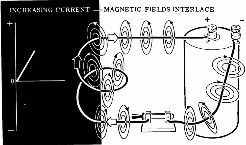
The lines of force around each turn continue their expansion and, in so doing, cut across adjacent turns of the coil. This expansion continues as long as the circuit current is increasing, with more and more lines of force from the coil turns cutting across adjacent turns of the coil.
