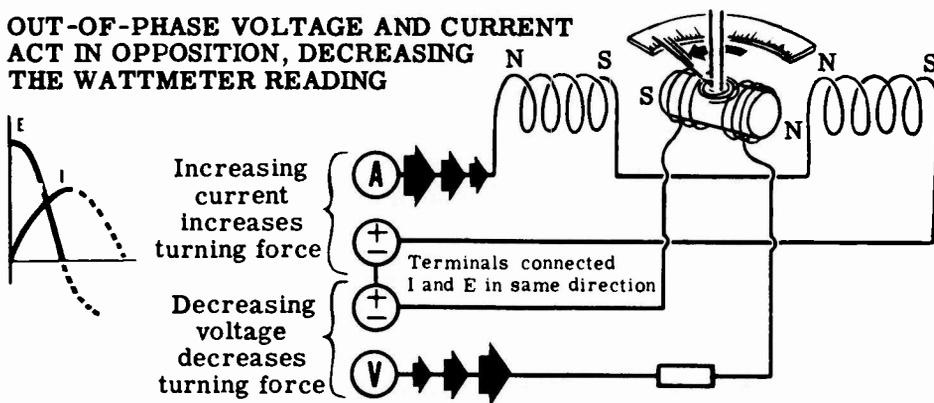
Similarly, if the current leads the voltage, the meter field strength and the moving coil current will not increase at the same time. This results in a lower wattmeter reading, the actual power used by the circuit again being less than the apparent power.
