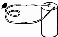
**INDUCTOR** — A coil of wire used to supply inductance in a circuit.
