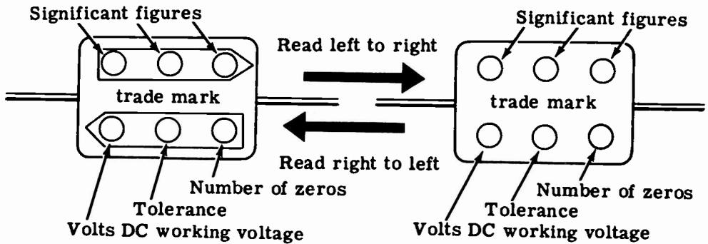
Suppose the six dots read in the correct order are brown, orange, green, red, silver and blue. The capacitor then has a capacitance of 13,500 mmf, a tolerance of 10 percent and a voltage rating of 600 volts.
