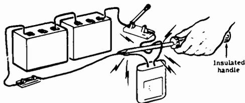
**CAPACITOR DISCHARGE** — Flow of electrons from the negatively charged plate of a capacitor to the positively charged plate, eliminating the charges on the plate.
