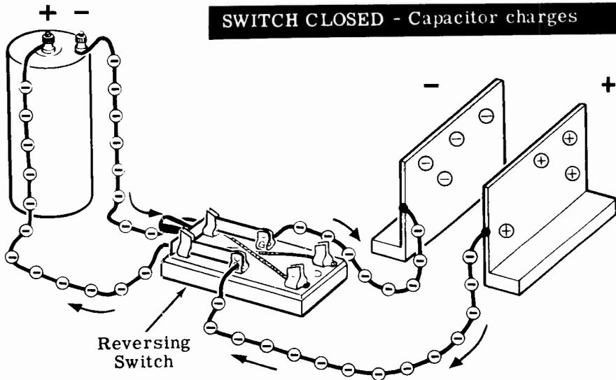
Whenever the switch is opened, the condenser retains the charges on its plates equal to the cell voltage.
