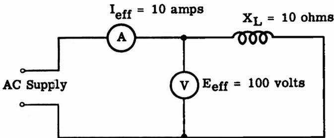
$$I_{\text{eff}} \times E_{\text{eff}} = \text{Apparent Power (VA)} = 1000$$
