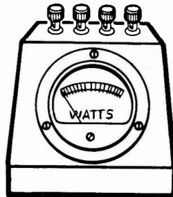
Remember that the power formula ( $P = EI$ ) can be used to find the power used in a resistive AC circuit, provided effective values of  $E$  and  $I$  are used.
