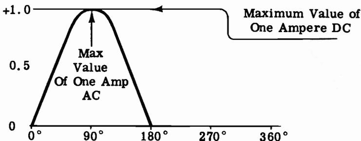
$$\text{AC } I_{\text{EFF}} = \frac{\text{The Heating Effect Of 1 Maximum AC Ampere}}{\text{The Heating Effect Of 1 Maximum DC Ampere}}$$
