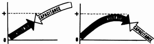
**CAPACITANCE** — The property of a circuit which opposes any change in the circuit voltage.
