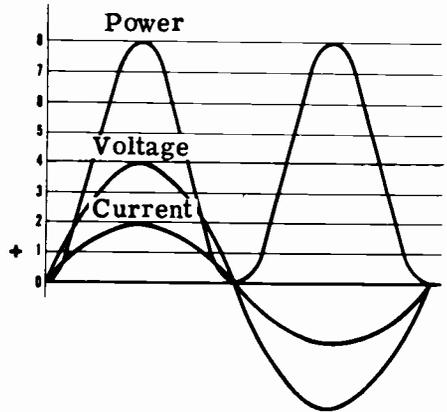
**AVERAGE POWER** — A value equal to the axis of symmetry drawn through a power wave.
