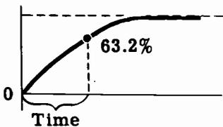
**CAPACITIVE TIME CONSTANT** — The product of RC which gives the time in seconds required for a capacitance to reach 63.2 percent of full charge.
