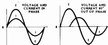
**PHASE ANGLE** — The amount in degrees by which the current wave lags the voltage wave.
