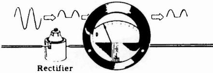
**RECTIFIER TYPE AC METER** — A basic DC meter movement with a rectifier connected to change AC to DC. Commonly used as an AC voltmeter.
