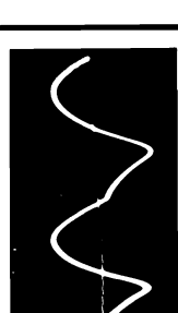
14 V101 PIN 9 HORIZONTAL OUTPUT GRID HORIZONTAL RATE 85V P-P
