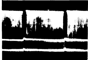
1. TP-3 Second Detector Vert. Rate 0.9V P-P
