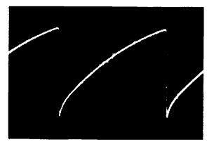
8. 17J78 Pin 6-7 Vertical Output Grid Vert. Rate 31V P-P
