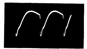
12 SR201 CATHODE JUNCTION HORIZONTAL PHASE DETECTOR HORIZONTAL RATE 12V P-P
