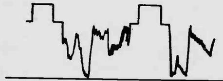
Envelope of Video Modulated Carrier Signal with Two Synchronizing Pulses. Average Rectified Voltage Varies a Great Deal.
