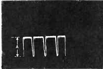
Vertical Sync Amp Grid Tube V6 Pin 4
