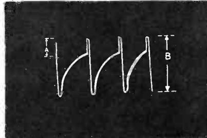
Vertical Saw Gen Grid Tube V7 Pin 4
