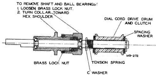
SOME MODELS MAY HAVE EXTRA SPACING WASHER TO INCREASE CLUTCH FRICTION
