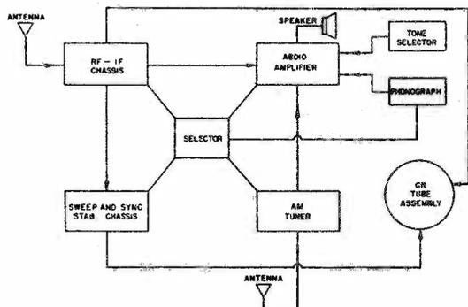
Figure 1. Block Diagram of RA-101 Receiver
