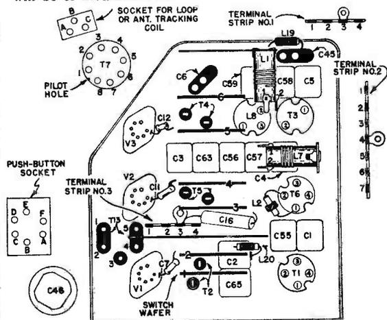
Figure 4—Physical Location of Components
