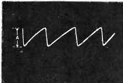
Horizontal Saw Gen Tube V2 Pin 5
