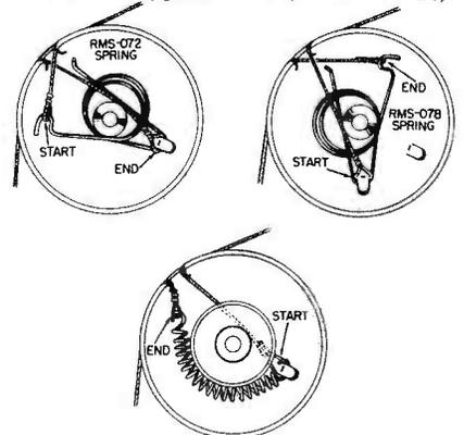
Figure 1—Dial Stringing Diagram Showing Later Production Springs
