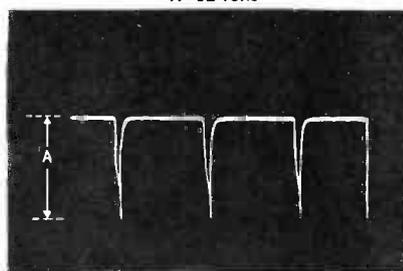
Damping Tube Plate Tube V5 Pin 2
