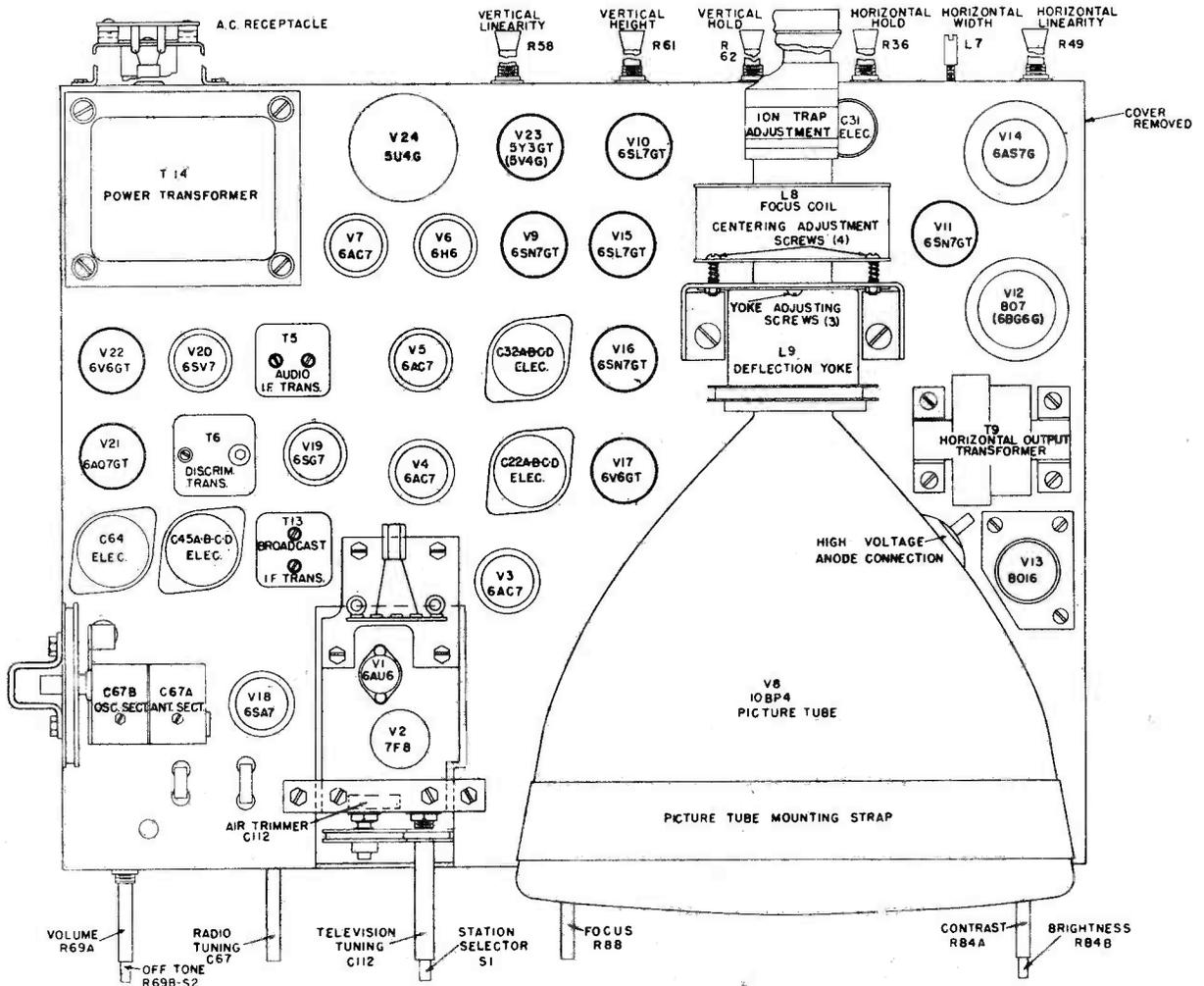
Fig. 13. Component Location, Top View of Chassis
