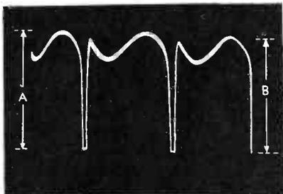
Cathode of Discriminator Tube V2 Pin 8 Sync Stab
