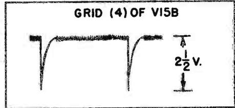
Fig. 48. Vert. Sync at V15B. (Osc. Synced at Half of Vert. Sweep Speed)
