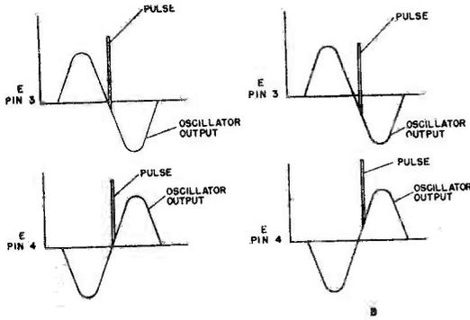
7(a) Oscillator Synchronized to Pulse Frequency
