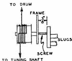
DETAIL OF FM COLLAR STRINGING AND CORRECT SETTING OF SLUG TUNER WITH TUNING CONTROL FULLY COUNTER-CLOCKWISE.
