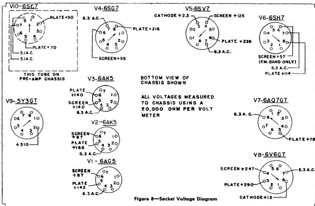
Figure 8—Socket Voltage Diagram
