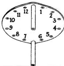
Figure 5—Identification of Switch Lugs
