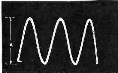
Oscillator Grid, Tube V3 Pin 5 Sync Stab
