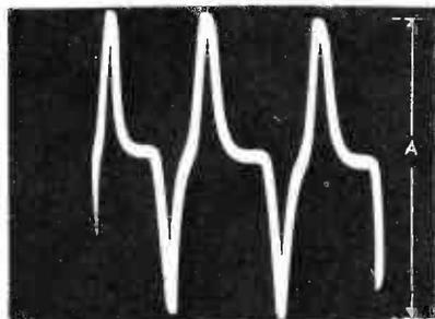
Horizontal Saw Gen Grid Tube V2 Pin 4
