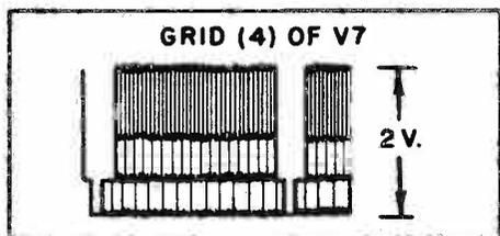
Fig. 35. Video Output of Detector (Osc. Synced at Half of Vert. Sweep Speed)
