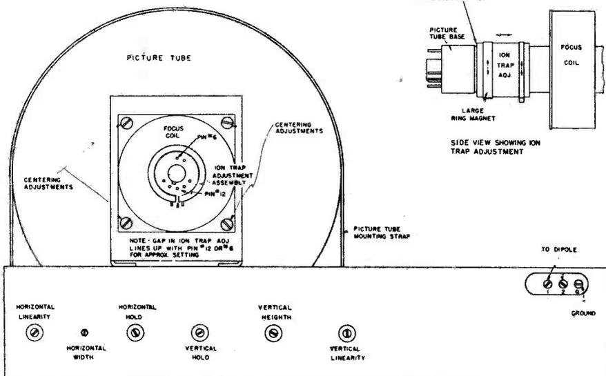
Fig. 17. Location of Installation Adjustment Controls
