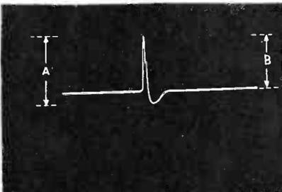
Vertical Sync Amp Plate Tube V6 Pin 8
