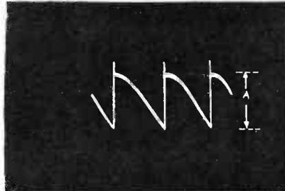
Vertical Amp Plate Tube V8 Pin 2
