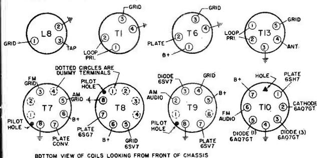
Figure 3—Terminal Identification of Coil Assemblies
