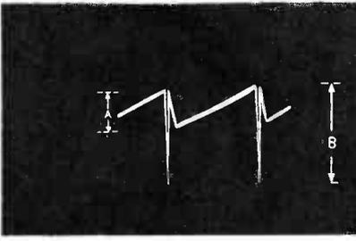
Vertical Saw Gen Plate Tube V7 Pin 5
