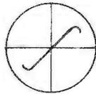
This presentation will be helpful for final alignment and balance of the discriminator transformer. Make sure that the straight center position crosses the exact center of the screen and that the distance from the vertical center line to each peak is approximately equal.
