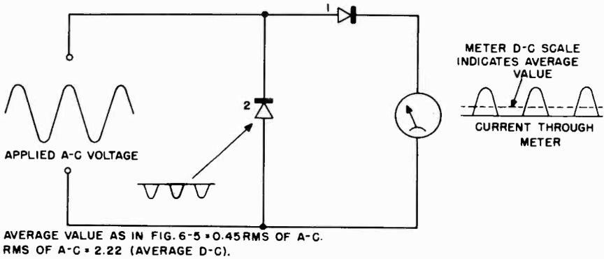
Fig. 6-3. Double-rectifier arrangement, which minimizes "back-current."
