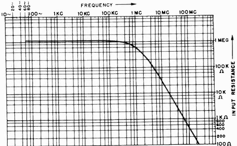
Fig. 9-24. Input resistance vs frequency curve for RCA type WV-75A.
