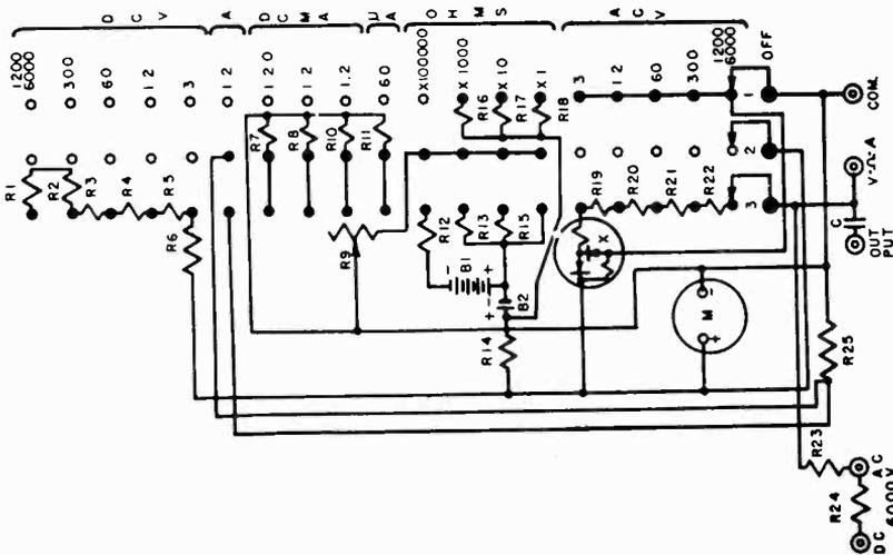
Fig. 8-11. Schematic of Triplett Model 630A VOM.
