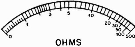
Fig. 4-5. Typical meter scale for shunt type ohmmeter.
