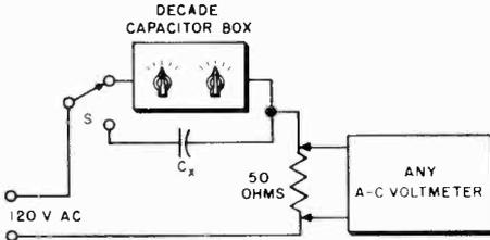
Fig. 10-17. Comparison method for measuring capacitance.
