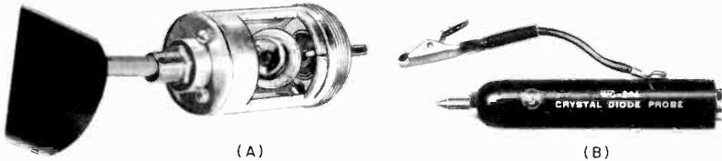
Fig. 9-14A. Vacuum tube diode probe.
