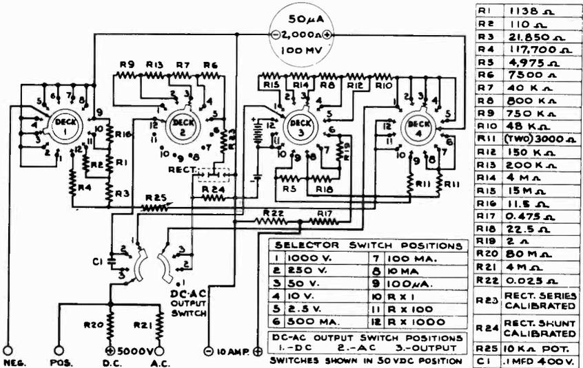
Fig. 8-12. Schematic of Simpson model 260 VOM.
