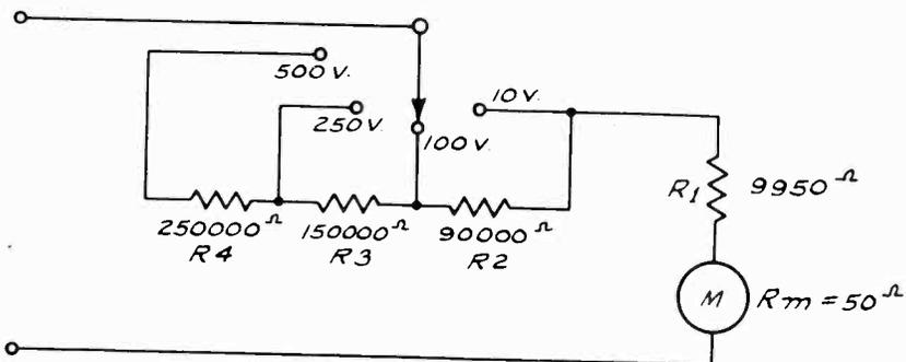
Fig. 8-7. Switching system for series connected voltmeter multipliers, using  $50 \mu$  meter for 500-volt maximum scale.
