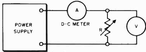
Fig. 10-19. Determining voltage regulation of a power supply.
