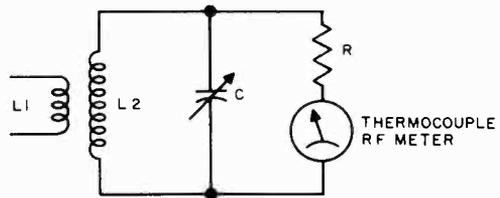
One type of indicator is a loop of wire whose ends are connected to a thermocouple milliammeter as shown. The r-f energy is coupled into the wire loop when the latter is held close to the plate tank coil and registers on the meter.
