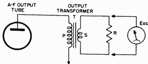
Fig. 10-54. Measuring the power output of an a-f amplifier.
