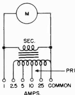
Fig. 8-5. Circuit of multi-range a-c ammeter with tapped current transformer.
