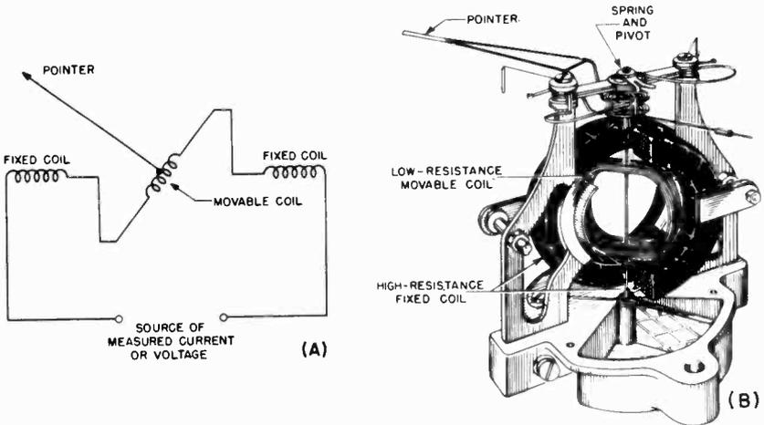
Fig. 2-8. (A) Schematic diagram showing the principle of the electrodynamic meter. The magnetic fields of the fixed and movable coils interact to cause the latter to rotate.
