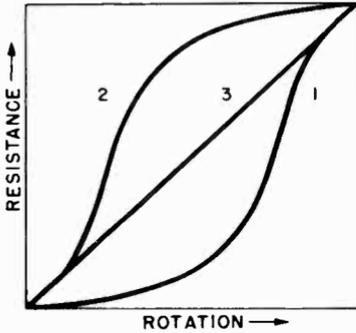
Fig. 10-29. Resistance variation and application of various tapers in volume controls.
