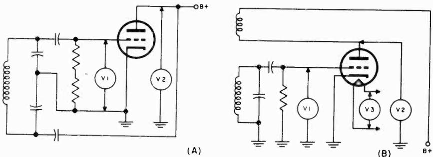
Fig. 10-40 (A) Examples of d-c operating voltages in Colpitts oscillator.
