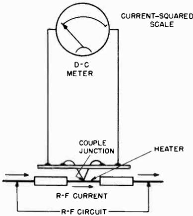
Fig. 7-1. Basic principle of the thermocouple meter. R-f current through the heater generates heat which raises the temperature of the thermocouple junction. The increased temperature of the couple causes it to produce a voltage, deflecting the pointer of the d-c instrument accordingly.
