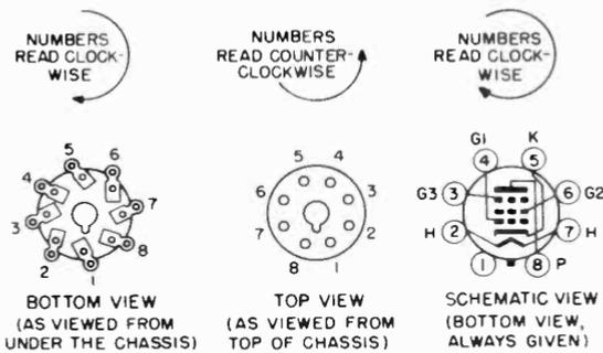
Fig. 10-25. Relation between the top and bottom views of an octal socket and schematic diagram of the tube as it would appear on a circuit diagram.
