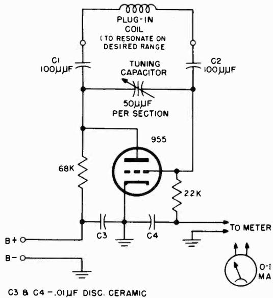
circuit to which the coil is coupled, the grid current “dips.” The dial connected to the variable capacitor is calibrated to read frequency. Thus, the resonant frequency of a circuit in a transmitter or receiver can be determined.
