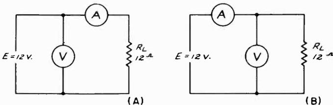
Fig. 5-2 If the ammeter A is connected as shown in A at the left, only the current drawn by the load  $R_L$  will be indicated on it; if it is connected as in B, right, then the ammeter reading will be the current drawn by both the load and the voltmeter, V.
