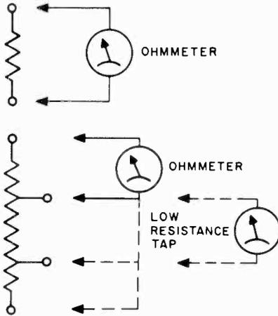
Fig. 10-27. When the resistance of a tapped resistor is being measured, each tap should be checked against a common point at one end, as indicated by this Figure. In addition, if the resistance of one section is relatively low, a separate reading directly across it is in order.
