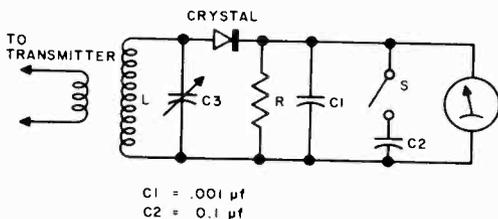
Fig. 11-6. Circuit suitable for measuring modulation percentage.
