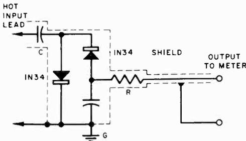
Fig. 9-21. Simple peak-to-peak r-f probe for VTVM.
