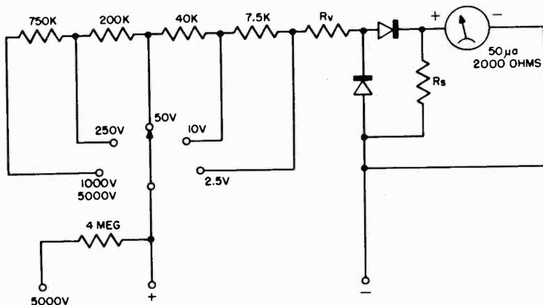
Fig. 8-8. Multiplier arrangement for a multi-range a-c voltmeter.
