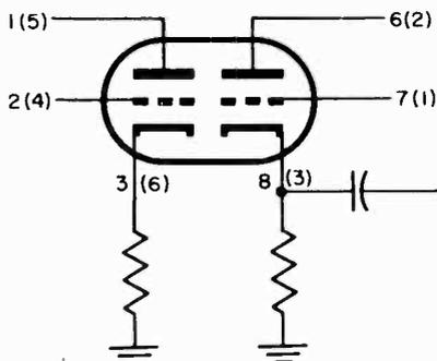
viewed from opposite directions, pin numbers run in *opposite* directions in top and bottom views, although the same pin number always applies to the same pin. For applications in which an alternate tube is suggested, a receiver schematic may show two sets of pin numbers. An example is given in Fig. 10-26. The alternate tubes in this instance are a 12AU7 and a 6SN7GT.
