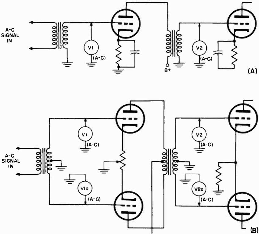
Fig. 10-53. Measuring gain in transformer-coupled amplifier.
