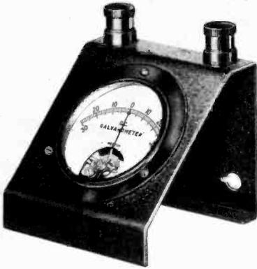
Fig. 1-5. A Weston center zero galvanometer.
