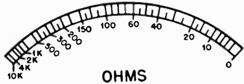
In this way the remainder of the meter scale is calibrated for ohmmeter use. A typical series-type ohmmeter scale is shown in Fig. 4-3. Notice how crowded the divisions become at the high-resistance (low current) end of the scale. For this reason, readings should always be taken in the higher-current (lower resistance) three-quarters of the scale, and the scale (or range) used should be chosen to make this possible.
