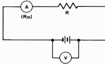
Fig. 4-1. Circuit for the volt-meter-ammeter method of measuring resistance.
