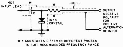
Fig. 9-20. Peak-reading r-f probe for VTVM.
