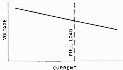
Fig. 10-20. Typical voltage regulation characteristic.
