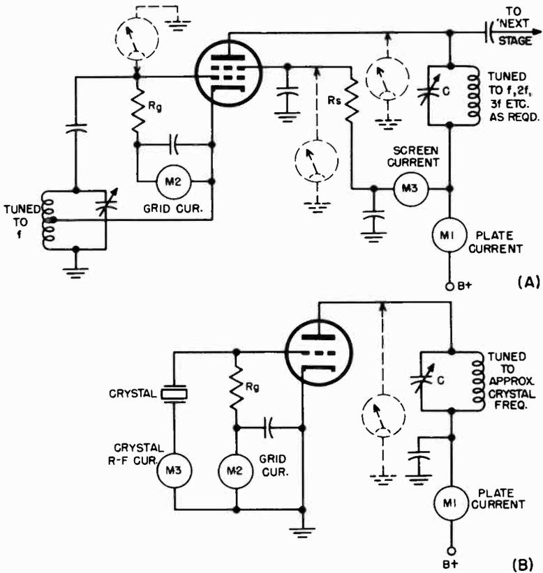
Fig. 11-(A) Electron-coupled oscillator circuit, such as is used for the frequency-controlling circuit of transmitters, and locations of typical meter measurements.
