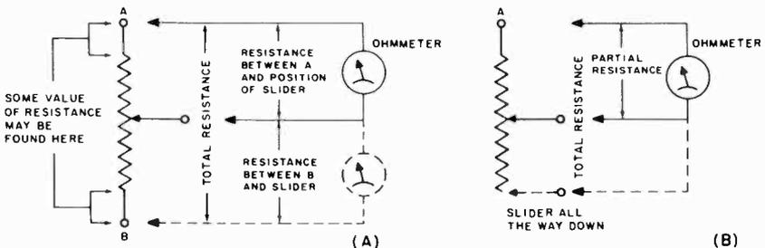
Fig. 10-28. Diagrams illustrating the measurement of variable resistors.
