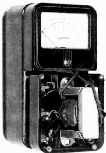
Fig. 8-4. Internal view of Simpson a-c current meter with current transformer.
