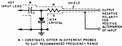
Fig. 9-20. Peak-reading r-f probe for VTVM.
