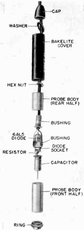
Fig. 9-19. Disassembled RCA duodiode probe used for measurements from audio frequencies up to about 250 mc.
