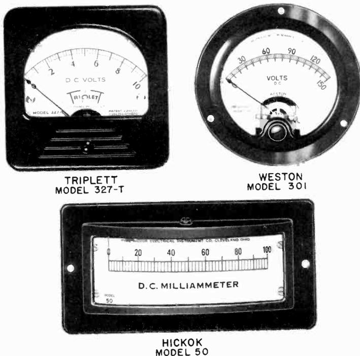
Fig. 10-1. Photographs of typical, modern panel meters. (Note: The above photos are reproduced through the courtesy of the manufacturers indicated.)
