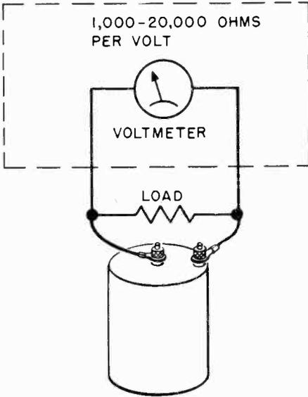
Fig. 10-8. Determining terminal voltage of a battery.
