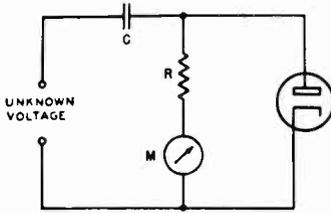
Fig. 9-10. Shunt type peak VTVM.
