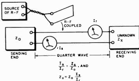
Fig. 10-13. How the r-f impedance of a device may be determined by use of a quarter-wave line and two thermocouple r-f ammeters.
