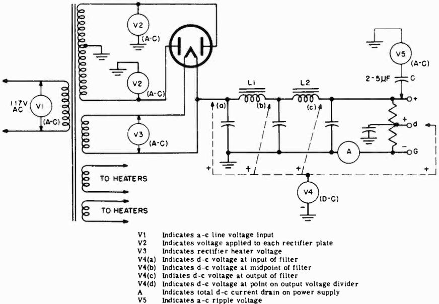
Fig. 10-44. Conventional full-wave B supply.
