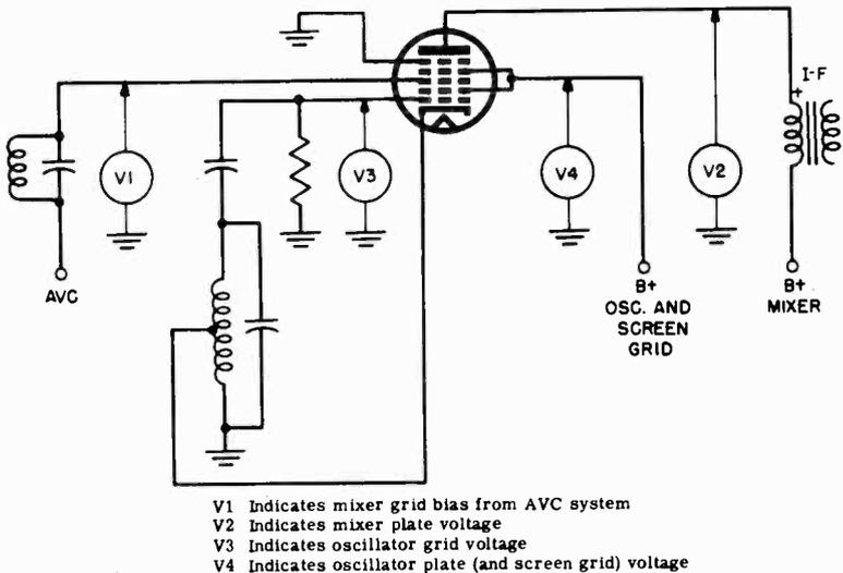
Fig. 10-42. Typical converter circuit with voltage-checking points.
