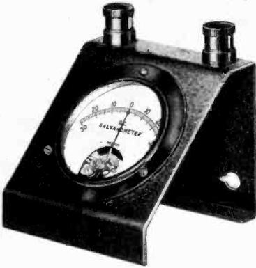
Fig. 1-5. A Weston center zero galvanometer.
