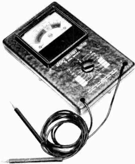
Fig. 10-7. RCA battery tester.
