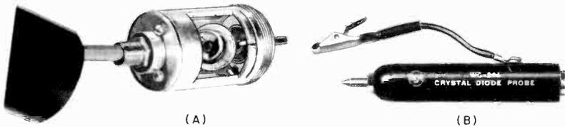
Fig. 9-14A. Vacuum tube diode probe.
