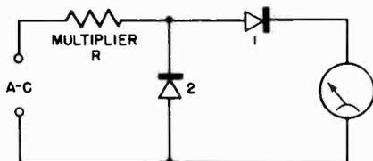
Fig. 6-5. Use of multiplier resistance in rectifier type a-c voltmeter.
