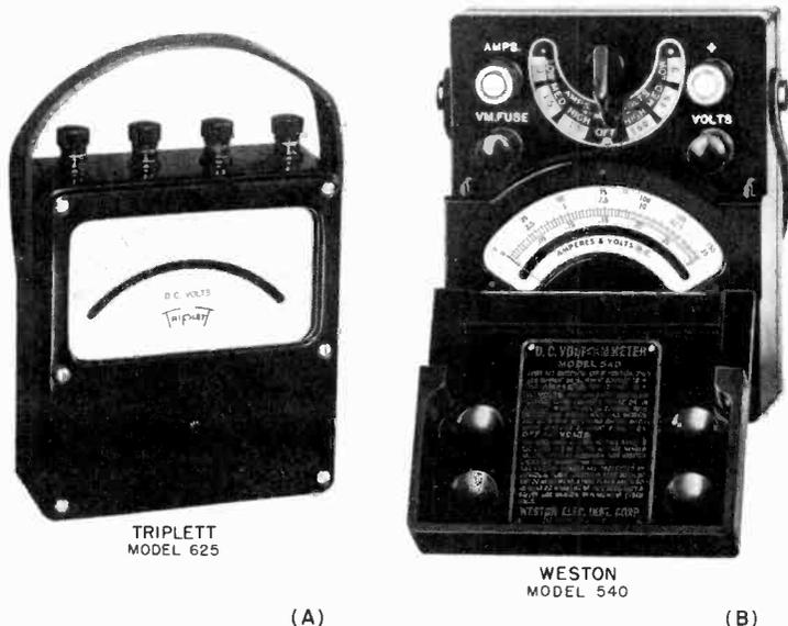
Fig. 8-1. Photos of multi-range instruments with terminals and with switch selector. (A) Triplet, (B) Weston.
