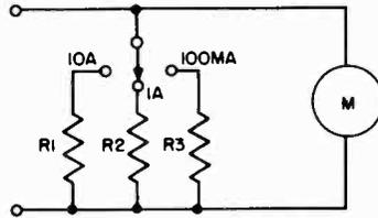
much more convenient arrangement is to select such shunts as enable the use of the original meter scale, multiplying the pointer indication by specific amounts as set by the shunt in use.
