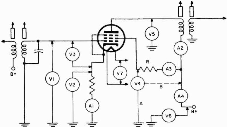
Fig. 10-35. A pentode transformer-coupled amplifier stage, showing locations for current and voltage readings. In a triode stage, readings are the same except that those connected with the screen grid and suppressor grid circuits are eliminated.
