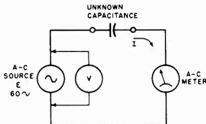
Fig. 10-16. Use of a-c source and current meter to measure capacitance. The a-c voltage source can be an isolation transformer with 120-volt output.
