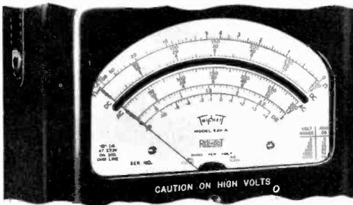
Fig. 8-14. View of scale on Triplet Model 630A VOM.
