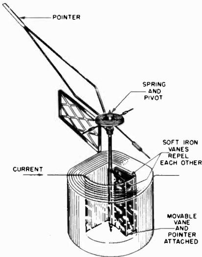
Fig. 2-4. Details of construction of the radial-vane type of moving iron meter.
