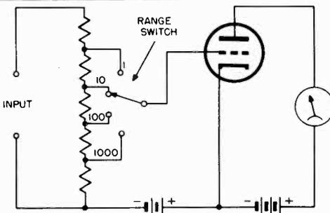
Fig. 9-2. Use of voltage divider in basic circuit.
