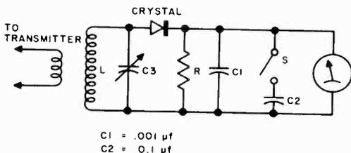
Fig. 11-6. Circuit suitable for measuring modulation percentage.
