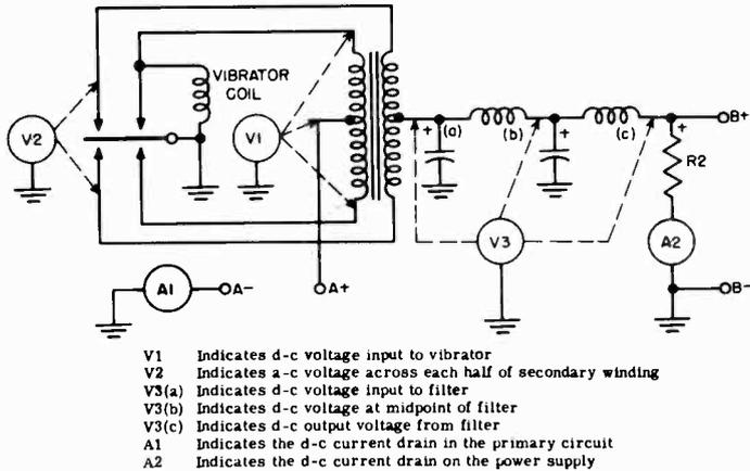
Fig. 10-46. Full wave synchronous vibrator power supply.
