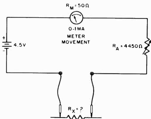
Fig. 4-2. Circuit of simple series type ohmmeter.
