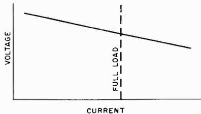
Fig. 10-20. Typical voltage regulation characteristic.
