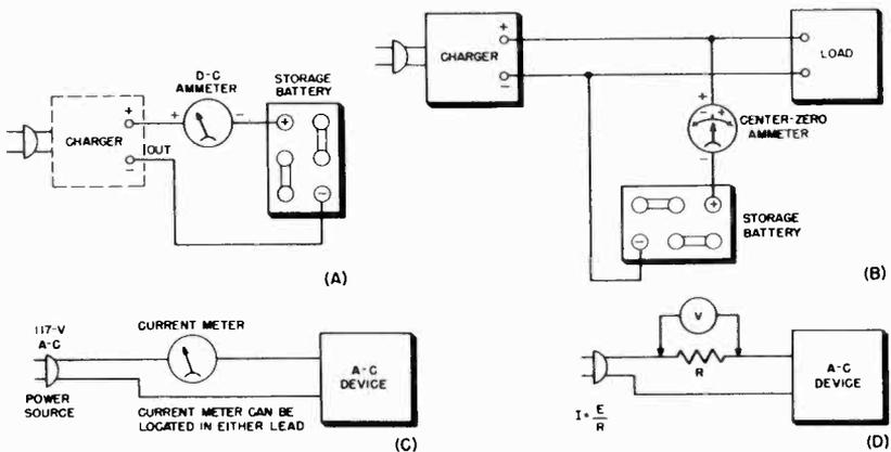
Fig. 10-9. (A) An ammeter connected to indicate rate of battery charge. (B) A center-zero meter used as a charge-discharge instrument. (C and D) Ammeter and voltmeter connected to measure current drain and power of device operated from the power line.
