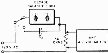
Fig. 10-17. Comparison method for measuring capacitance.
