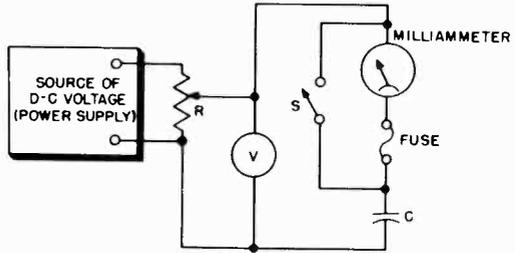
Fig. 10-14. Arrangement for measuring leakage current of capacitors.
