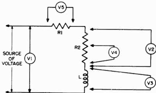
Fig. 3-11. Application of voltmeters for voltage measurement.
