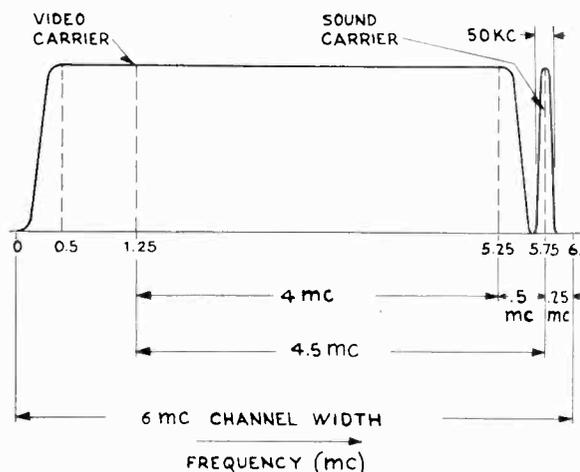
Fig. 2-4.—Actual over-all response curve of a television channel. Note that the response drops off and then rises again to a sharp peak at the sound carrier.
