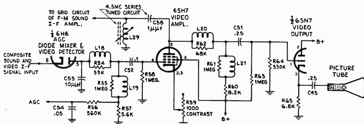
FIG. 6-36.—The video detector and amplifier unit of the Hallicrafters model T-54 makes use of the interaction of the video and sound signals, and the composite signal is fed to a 6H6 duo-diode tube which functions as diode detector, diode mixer, and source for agc.
