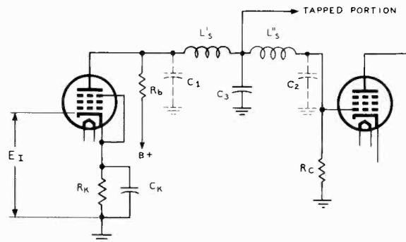
FIG. 7-10.—In order to improve amplification and phase-shift characteristics, two series peaking coils are employed, thus bettering the response characteristics that one such coil provides.
