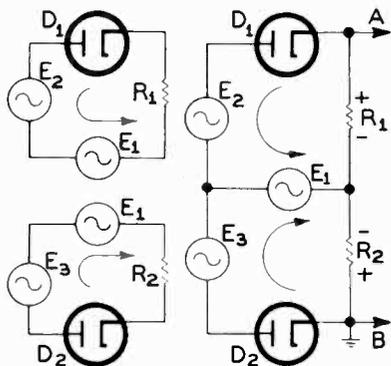
Fig. 5-11. — Simplified schematics of the diodes of Fig. 5-8 and their respective load resistors. These two schematics are combined on the right. This is permissible since the voltage  $E_1$  is common to both diodes.
