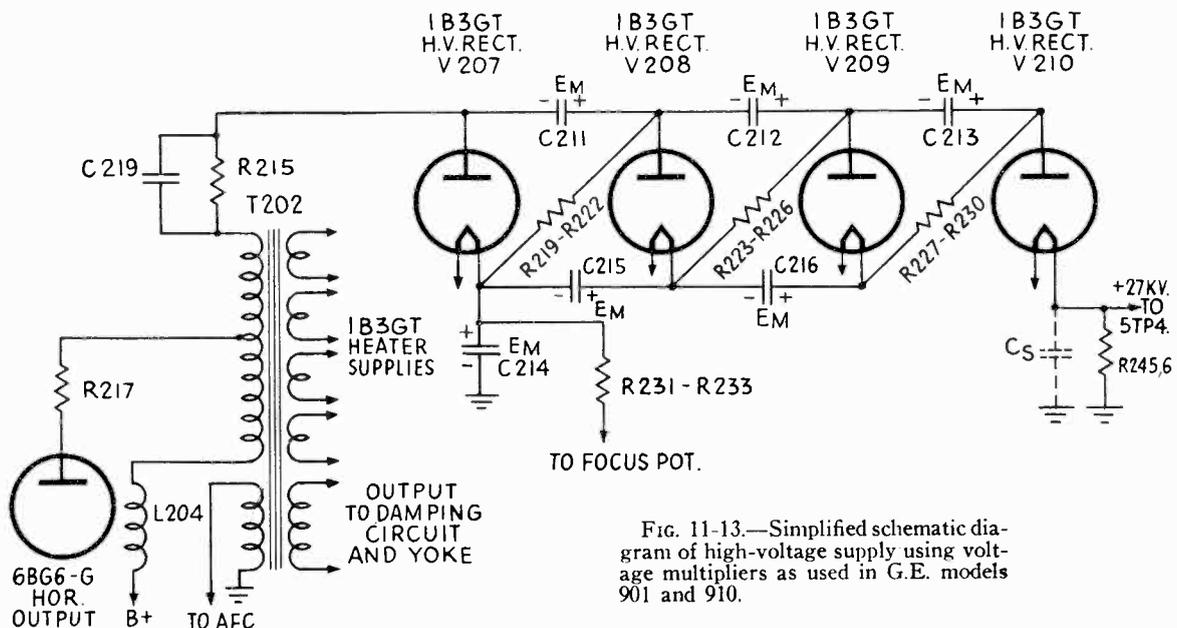
FIG. 11-13.—Simplified schematic diagram of high-voltage supply using voltage multipliers as used in G.E. models 901 and 910.
