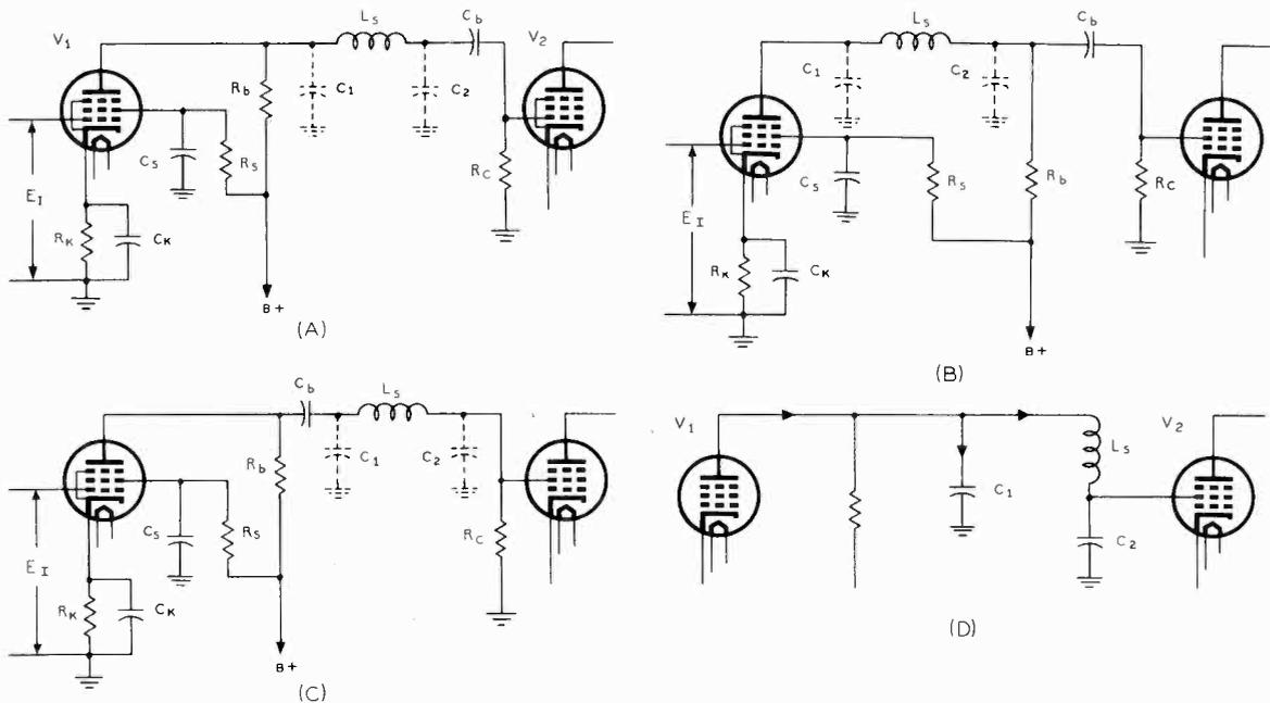
FIG. 7-8.—A typical series peaking high-frequency compensated video amplifier circuit is shown in (A) and a simplification of this circuit in (D). The circuits in (B) and (C) are variations of (A), these being sometimes used to isolate the shunting capacities at some specific ratio.
