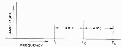
mentioned, according to the FCC, each television channel occupies an over-all bandwidth of 6 mc. This includes the video-modulated signals and the sound f-m signals.
