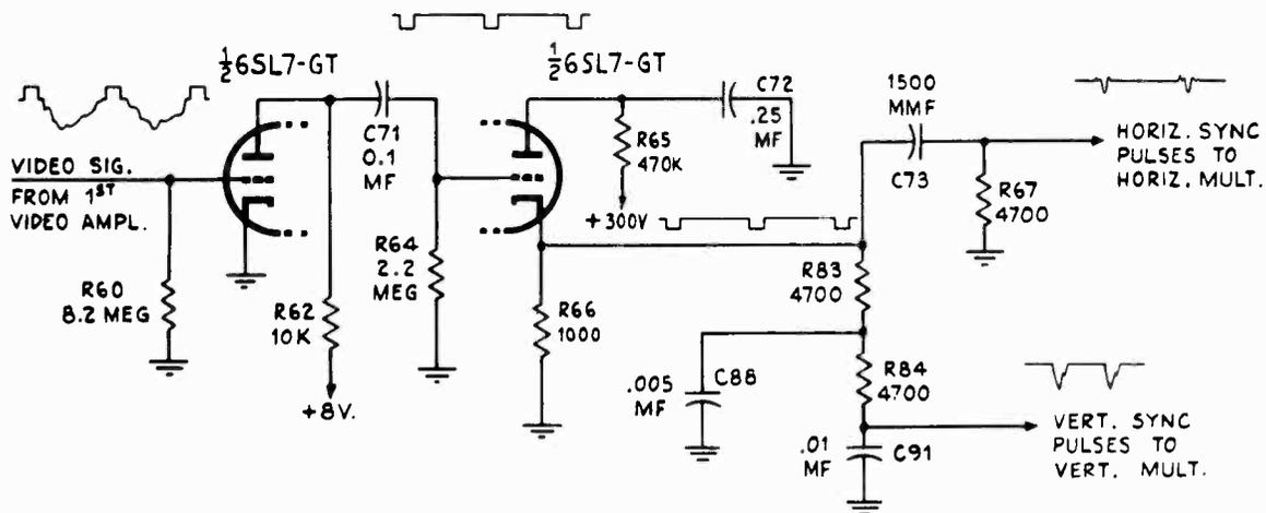
FIG. 8-5.—Partial schematic of the sync circuits of Belmont models 22A21, 22AX21, and 22AX22.
