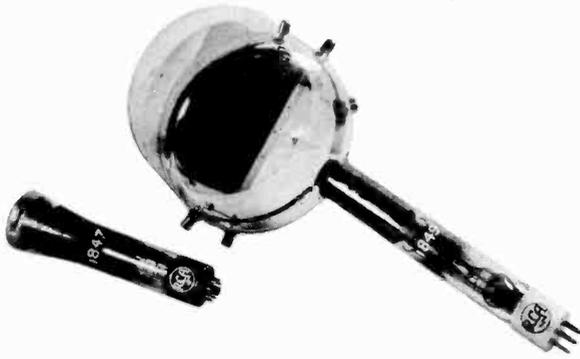
Fig. 1-10.—Both a large and a small Iconoscope are shown.
