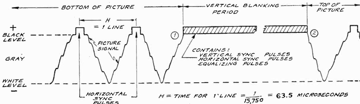
Fig. 1-20.—The video signal showing the last two lines of a field followed by a vertical blanking period. Horizontal sync pulses are shown on the horizontal pedestals and the vertical sync pulse is transmitted during the vertical blanking period.
