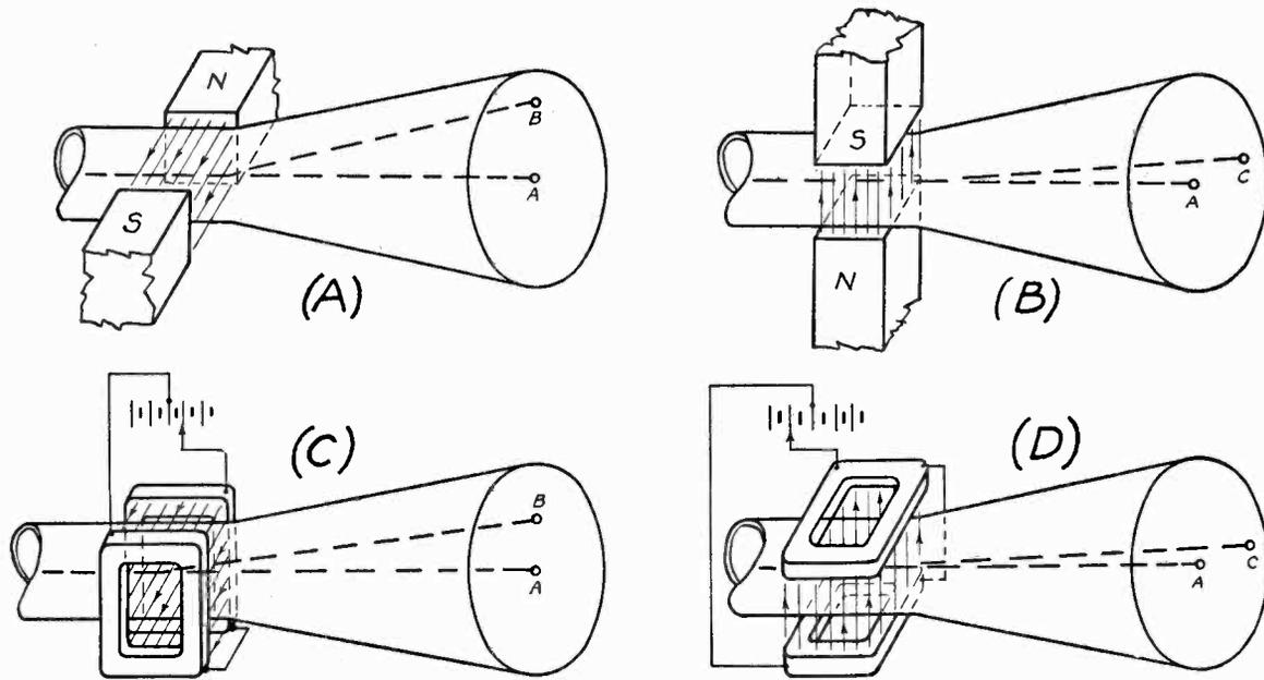
Fig. 1-8.—The magnetic deflection coils in (C) and (D) provide a magnetic field similar to that of the permanent magnets in (A) and (B). Note that the beam is deflected at right angles to the lines of force.
