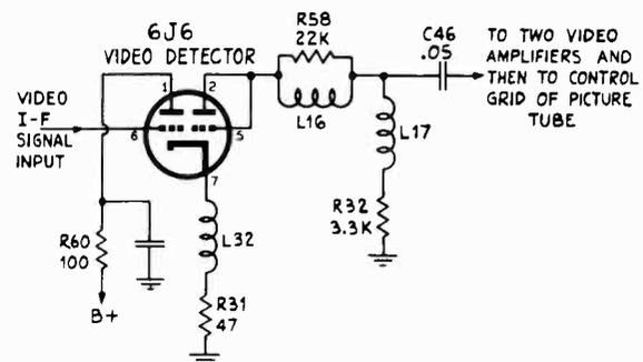
FIG. 6-35.—Unlike any of the models previously illustrated, the Television Assembly model F1-101 employs a duo-triode 6J6 tube as a video detector. The circuit is a diode rectifier driven by a cathode-follower stage, with the first triode section acting as the cathode-follower driver and the second as the diode detector.
