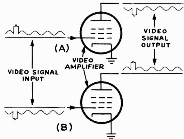
FIG. 6-29.—Because signals undergo a phase reversal of 180° between the input and output circuits of an amplifier tube, the video signals shown in Fig. 6-28 (A) and (B), when applied to the video amplifier grid, are reversed in phase in the amplifier output, as shown in (A) and (B) above.
