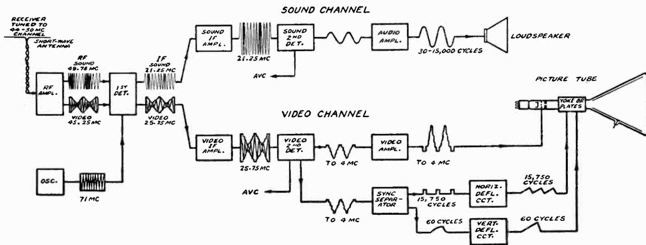
Fig. 1-24.—A block diagram of a typical television receiver. Note the changes in the signal as it passes through the receiver.
