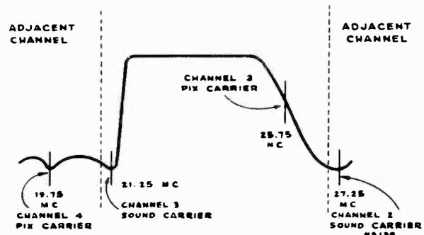
FIG. 12-5.—An over-all video response characteristic for channel 3, showing the interfering frequencies which must be eliminated by means of traps.
