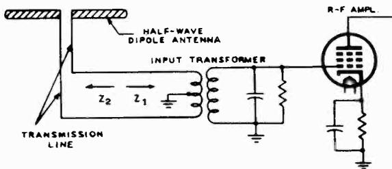
FIG. 3-9.—In order to effect a maximum transfer of energy from the antenna to the control grid of the r-f amplifier tube, the impedance  $Z_2$  of the transmission line and antenna should equal the impedance  $Z_1$  seen looking into the primary of the input transformer.
