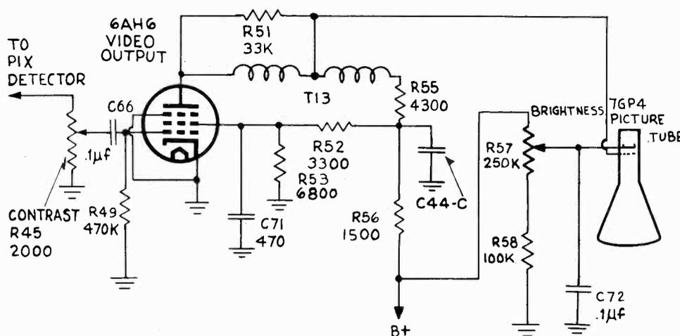
FIG. 7-20.—The video output circuit of the Belmont model 21A21 is an example of the grid leak-capacitor type of d-c restorer, which is the same as the basic circuit shown in Fig. 7-19.
