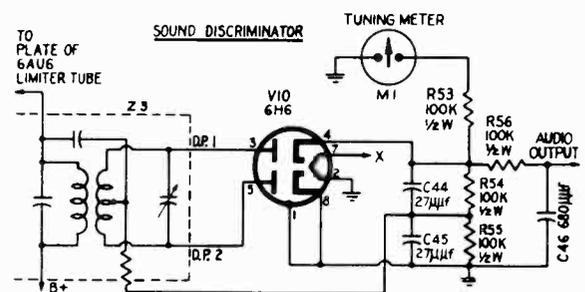
Fig. 5-17.—Sound discriminator circuit of the Du Mont television receiver model RA-102. Note that the coil  $L$  in Fig. 5-8 has been replaced by resistor  $R$ .
