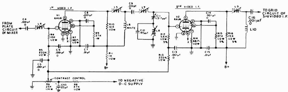
FIG. 6-21.—The d-c potential across the contrast control is often obtained from a negative d-c source in the power supply as in this Du Mont RA-102 receiver in which the contrast control is within the 40-volt d-c supply.
