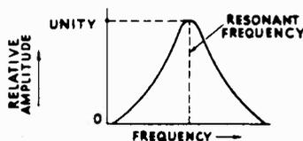
Fig. 5-2.—Typical response characteristic of a sound i-f stage in a television receiver.
