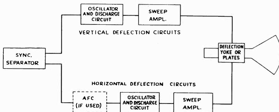
FIG. 9-1.—Block diagram which shows the essential portions of the sweep circuits which are used in television receivers. Horizontal and vertical sync pulses go from the sync separator to the respective deflection circuits as shown. Both sweep circuits are basically similar, the differences being due to the operating frequencies.
