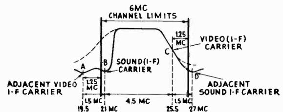
FIG. 6-15.—A normal over-all video i-f response curve with an ideal flat top is shown by the solid-line part of this curve. If traps were not used, the curve would probably end as indicated by the dashed lines, allowing undesired signals at *A*, *B*, and *D* to pass. Reduced in amplitude through the use of traps, their interference becomes negligible.
