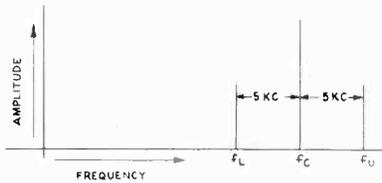
Fig. 2-1. — The frequency spectrum of a typical 100-percent-modulated a-m wave. The amplitude of the sidebands is half that of the carrier.
