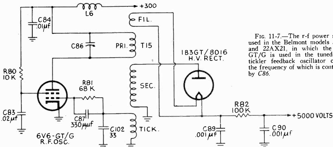
FIG. 11-7.—The r-f power supply used in the Belmont models 22A21 and 22AX21, in which the 6V6-GT/G is used in the tuned-plate, tickler feedback oscillator circuit, the frequency of which is controlled by C86.
