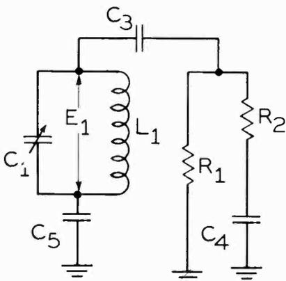
Fig. 5-23.—A simplified drawing of the i-f paths that appear across the transformer primary to ground in Fig. 5-22.
