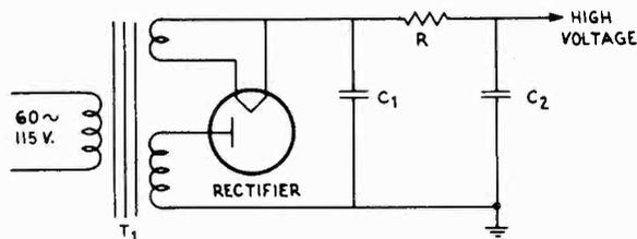
FIG. 11-5.—The basic 60-cycle power supply circuit. Here large values of filter resistance rather than large values of capacitance are used to obtain the necessary filtering.
