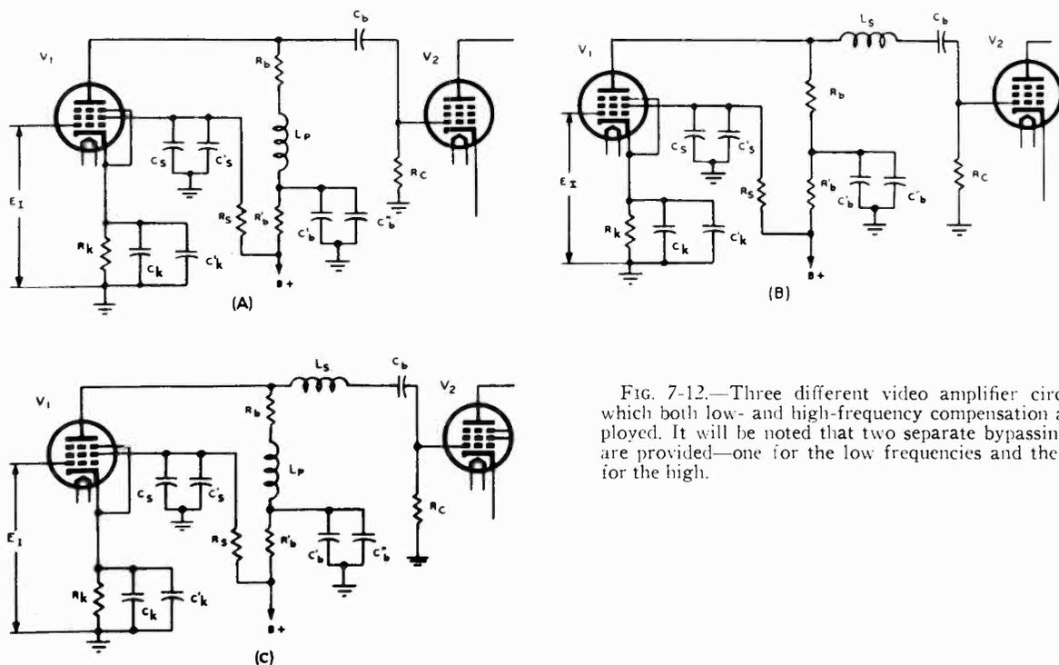
FIG. 7-12.—Three different video amplifier circuits in which both low- and high-frequency compensation are employed. It will be noted that two separate bypassing paths are provided—one for the low frequencies and the second for the high.
