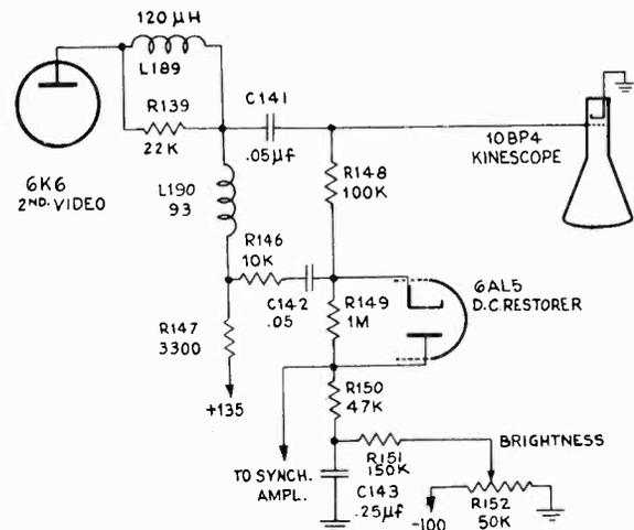
FIG. 7-21.—The video output stage of the RCA model 630TS is an example of a diode d-c restorer. It will be noticed that several changes have been made when it is compared with the basic circuit of Fig. 7-17.
