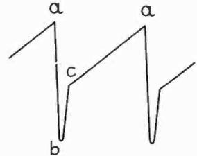
FIG. 11-10.—The saw-tooth waveform with a negative pulse, that is applied to the grid of the 6BG6G tube.
