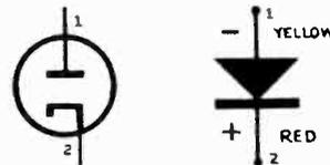
Fig. 11-3, left.—In the schematic symbol for the selenium rectifier on the right, the electron flow is from 2 (identified by a red dot) upward to 1 (identified by a yellow or no dot).
