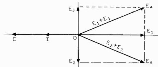
Fig. 5-12.—Vector diagram of the current and voltage relationships of the phase discriminator of Fig. 5-8 at resonance when both secondary voltages  $E_2$  and  $E_3$  have a  $90^\circ$  phase difference from  $E_1$ .
