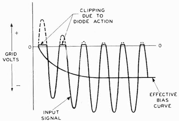
Fig. 5-7.—The solid curves above the zero axis show a uniform amplitude due to clipping; the dotted portions above the zero axis show what the signal would be if no clipping occurred.
