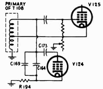
FIG. 8-9.—Schematic diagram of the horizontal sweep oscillator circuit of RCA model 630TS.
