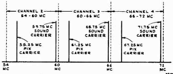
FIG. 12-4.—A typical television channel, No. 3, with adjacent channels 2 and 4.
