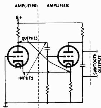
FIG. 9-4.—Simple form of the Potter sweep circuit, which is arranged to correspond with the block diagram of Fig. 9-3.
