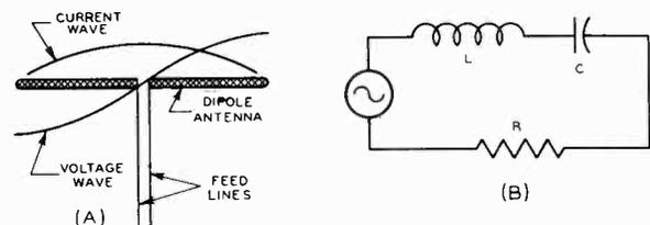
FIG. 3-6.—A half-wave dipole antenna (A) and its equivalent series resonant circuit (B), where the resistive component  $R$  is primarily the radiation resistance of the antenna.
