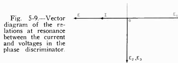
Fig. 5-9.—Vector diagram of the relations at resonance between the current and voltages in the phase discriminator.
