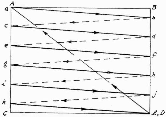
Fig. 1-14.—A simple progressive scanning pattern in which the picture is scanned in a series of lines which start at the upper left and slope down to the right.
