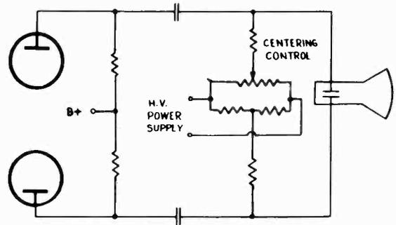
FIG. 9-8.—When electrostatic deflection is used on the picture tube, the final sweep amplifier can be connected to the deflection plates as shown in this schematic.
