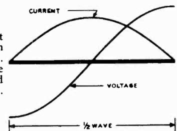
FIG. 3-4.—The current and voltage distribution along a half-wave antenna. Note that at the ends the current is a minimum and the voltage a maximum. Compare with Fig. 3-3.
