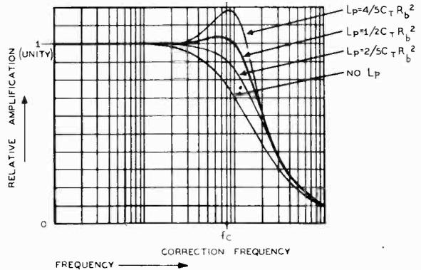
FIG. 7-7.—The manner in which the peaking inductance affects the high frequencies is shown in these typical response curves, each utilizing a different value of  $L_p$ .
