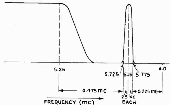
Fig. 2-5.—An enlargement of the upper frequency end of the television channel.
