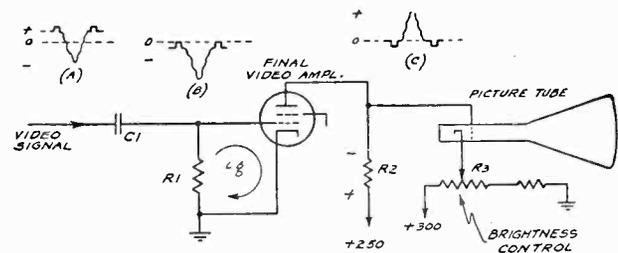
FIG. 7-19.—A widely used type of d-c restorer circuit in which the video amplifier output tube is operated at zero bias so that the grid-cathode elements function as a diode to reinsert the d-c component.
