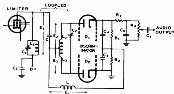
Fig. 5-8.—Schematic of a conventional phase discriminator detector.
