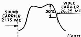
FIG. 6-6.—The over-all video i-f response curve of the overcoupled i-f transformer stages of the Farnsworth model GV-260. Courtesy Farnsworth Tel. and Radio Corp.
