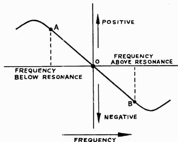
Fig. 5-15.—The S curve represents the typical output characteristic of the discriminator circuit with the output a-f voltage plotted against the instantaneous values of input frequency.
