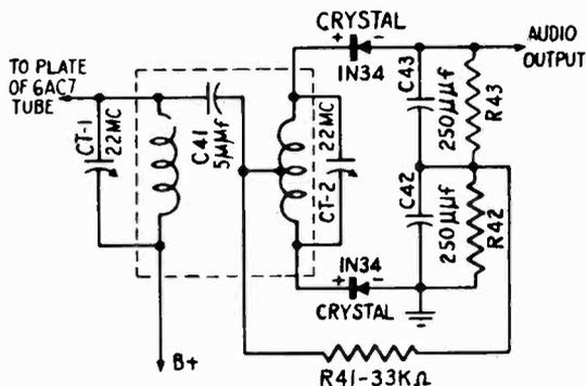
Fig. 5-24.—The discriminator circuit used in the Consolidated Television model 2315. Note that a resistor is used in place of the usual coupling coil.
