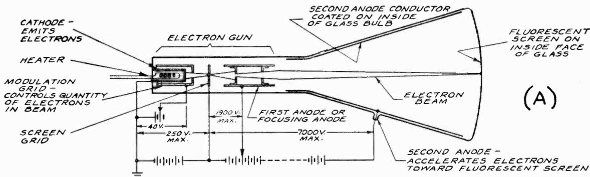
Fig. 1-6.—The different elements of a picture tube are shown in (A) with typical operating voltages. (B) shows a common schematic representation of this tube; K is the cathode, G the modulation grid, S the screen grid, F the focusing anode, and A the second anode.
