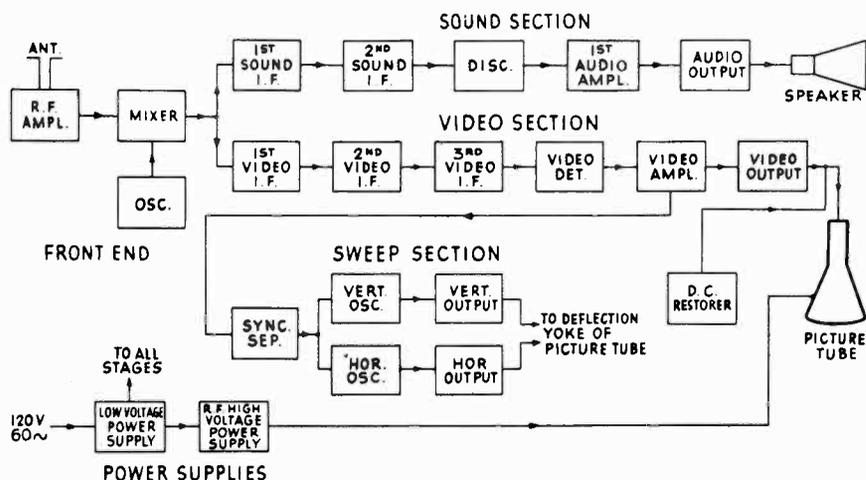
FIG. 12-1.—Block diagram of a television receiver, which can be divided into five sections: the radio frequency or front end, the sound, video, sweep and sync sections, and the power supplies. In order for the set to function properly, the tuned circuits in these sections must be aligned to certain frequencies.
