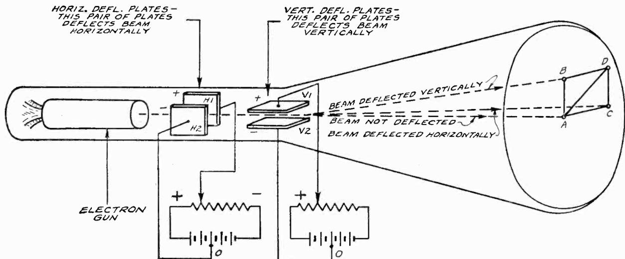
Fig. 1-7.—The electron beam in this picture tube is electrostatically deflected by the two pairs of plates.  $H_1$  and  $H_2$  deflect the beam horizontally, and  $V_1$  and  $V_2$  deflect it vertically.
