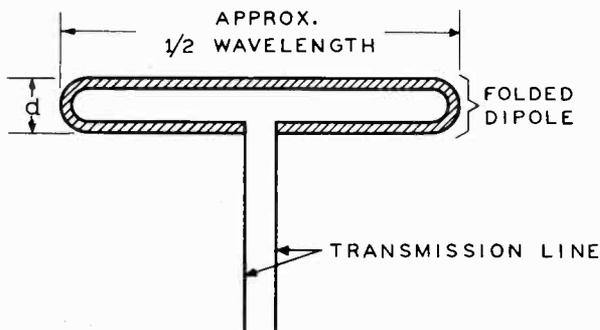
FIG. 3-11.—A folded half-wave dipole antenna, where  $d$ , the distance between the two half-wave sections, is small in comparison with the wavelength.
