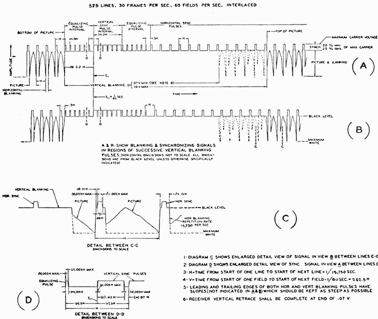
Fig. 1-21—The standard television signal. Part (A) shows the signal at the end of any one field; part (B) shows the signal at the end of the next field, 1/60 second later. The difference between the two fields is caused by interlacing.
