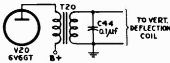
FIG. 9-12.—In the GE model 802, this circuit is used to produce a trapezoidal waveform by adding suitable pulses to a saw-tooth wave.
