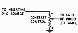
FIG. 6-20.—This type of contrast control, in which a d-c potential exists across the contrast control and its positive side is grounded, is common in television receivers.
