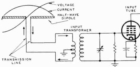
FIG. 3-19.—Half-wave dipole and input circuit to the r-f amplifier. The arrows indicate the current flow, which being a maximum in the transformer primary, induces a maximum voltage in the secondary at the frequency of operation.
