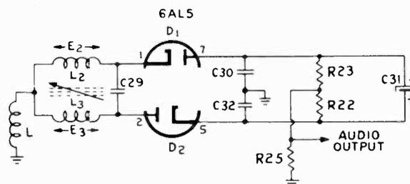
Fig. 5-29.—The conduction current flowing in coil  $L_3$  will induce a voltage in coil  $L_2$ . This induced voltage in turn causes an induced current to flow in  $L_2$ .
