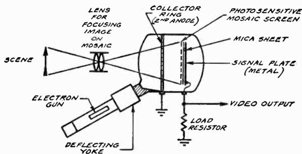
Fig. 1-11.—The elements of the large tube shown in Fig. 1-10 are easily identified. Light images formed on the signal plate are transformed into electrical energy by the scanning beam.
