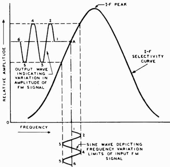
Fig. 5-30.—When an f-m i-f signal falls on the sloping characteristic of the i-f response curve, detection of an f-m signal is possible.
