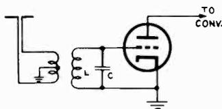
Fig. 4-1.—The simplest type of transformer coupling is the single-tuned circuit.
