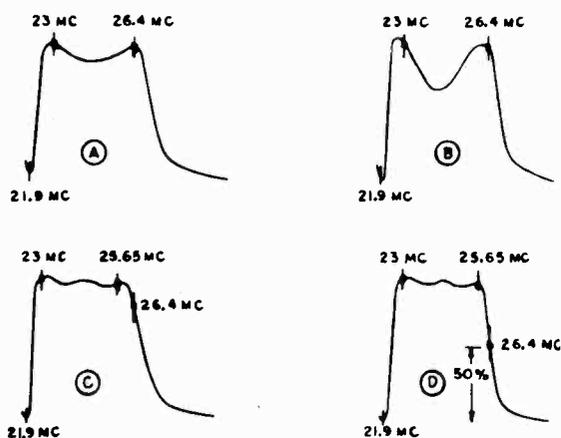
FIG. 6-4.—Curves representing the video i-f signal of the GE model 802 at different points in the i-f system. The double-peaked curves *A* and *B* represent, respectively, the response of the fourth i-f stage and the additive signal of the third and fourth stages. The single-peaked curve *C* represents the addition of the second, third, and fourth stages, and *D* the over-all video i-f response curve of the receiver.
