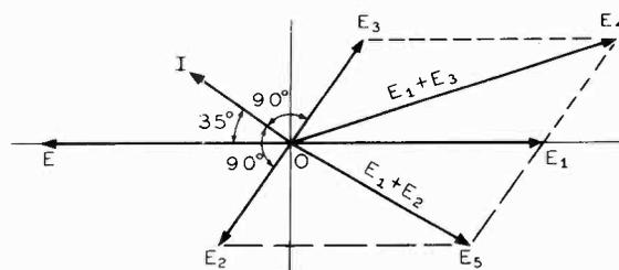
Fig. 5-13.—Vector diagram of the current and voltage relationships in the phase discriminator when the instantaneous frequency of the signal is higher than the resonant frequency of the transformer.
