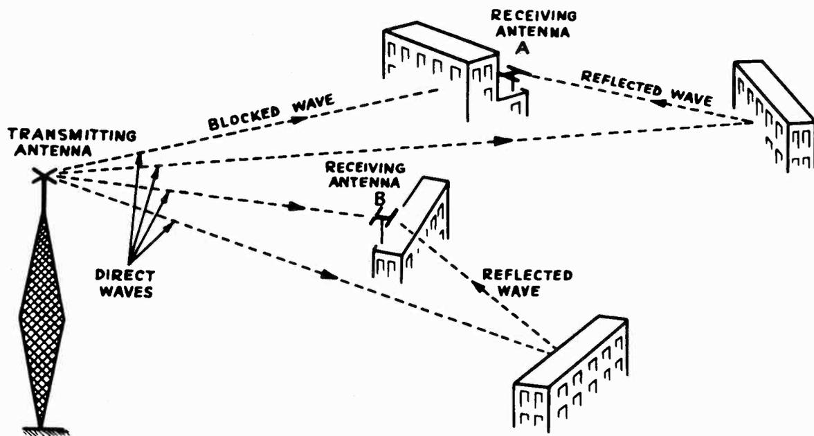
FIG. 3-16.—Receiving antenna *A* picks up only a reflected wave because the building it is on blocks the direct waves. Receiving antenna *B* is in the open and receives both a direct wave and a reflected wave, thus creating ghosts in the television receiver.
