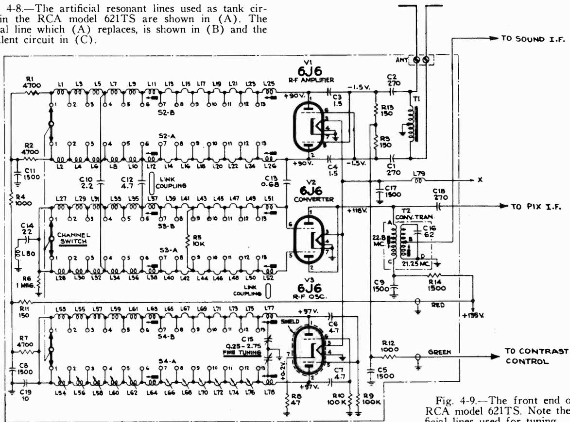
Fig. 4-9.—The front end of the RCA model 621TS. Note the artificial lines used for tuning.
