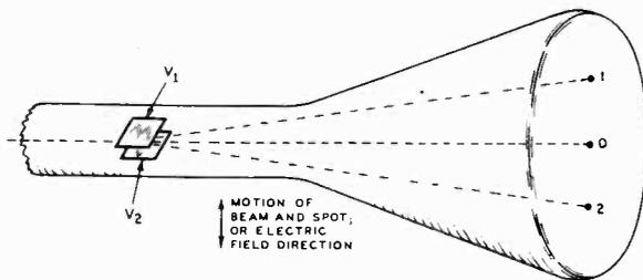
FIG. 10-3.—When a positive voltage is applied to  $V_1$  and a negative voltage to  $V_2$ , the spot caused by the beam will rise to point 1 from 0 at the center of the screen. When the voltages are reversed in polarity, the spot will descend to point 2.
