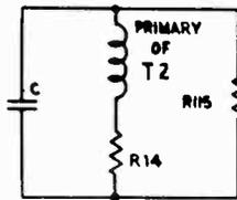
FIG. 6-8.—In this simple network representing the primary of  $T2$ ,  $C$  is the over-all capacitance in the circuit;  $R115$  is the grid-leak resistor and together with  $R14$  the load resistor, reduces the  $Q$  and makes the response less sharp than it otherwise would be.
