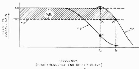
FIG. 7-9.—Typical response characteristic curves, wherein the voltage gain is relative, its maximum value being taken as unity at the intermediate frequencies.
