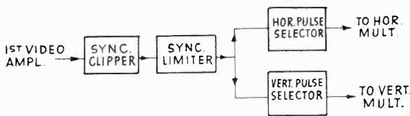
FIG. 8-4.—Block diagrams of the sync circuits used in the Belmont models 22A21, 22AX21, and 22AX22.
