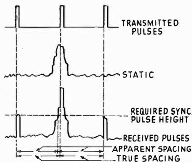
FIG. 8-1. — Apparent change in sync pulse spacing caused by static.
