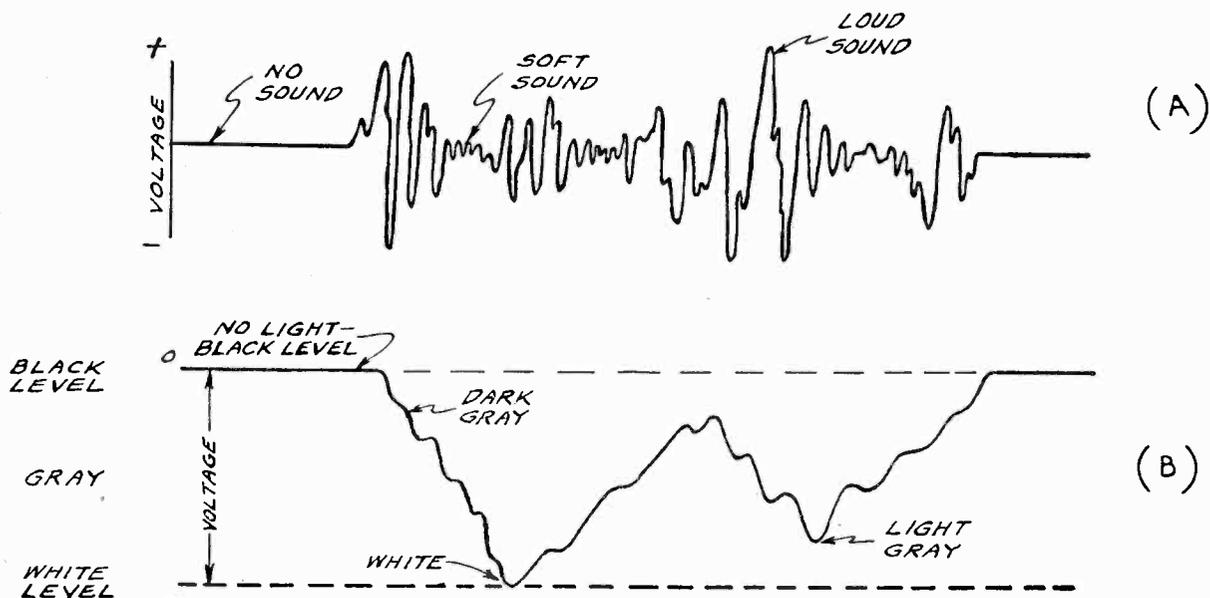
Fig. 1-18.—Comparison between a sound and video signal. In the video signal, black is represented by a fixed level, and various shades of brightness are represented by voltages displaced proportionately from the black reference level.
