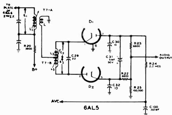
Fig. 5-28.—The modified ratio detector circuit appearing in the Belmont model 22A21.
