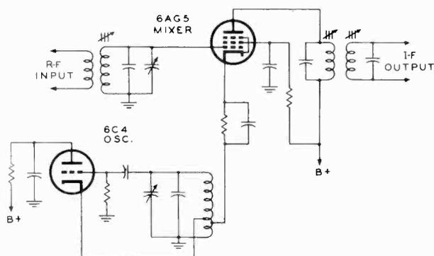
Fig. 4-4.—A typical oscillator-mixer circuit as used in television receivers.
