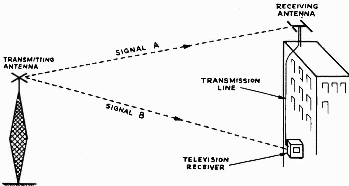
FIG. 3-18.—Two signals are received at the television receiver, one is picked up by the antenna and the other signal is picked up directly by the receiver.
