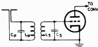
Fig. 4-2.—The gain of this double-tuned circuit is improved over that of Fig. 4-1.
