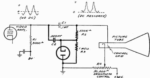
FIG. 7-17.—The heavy portion of the circuit shows a typical d-c restorer circuit arranged to restore the d-c component to the video signal before it is applied to the control grid of the picture tube.
