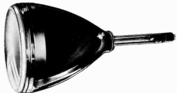
Fig. 1-5.—A Kinescope (picture tube) with a 12-inch screen.
