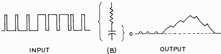
FIG. 8-3, right.—Effect of series resistance-capacitance circuit on input pulses, showing (A) the signal observed when like narrow pulses are applied and (B) when the input consists of two different kinds of pulses.
