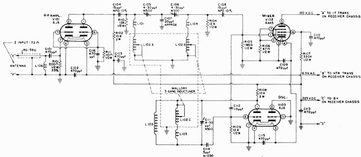
Fig. 4-10.—The r-f amplifier, oscillator, and mixer circuits of the Du Mont model RA-103.
