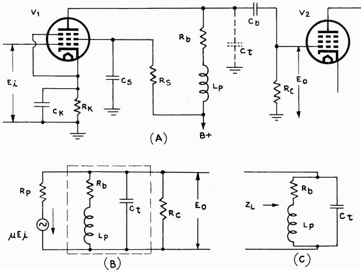
FIG. 7-6.—A typical video amplifier compensated only at the high-frequency end is shown in (A) and its equivalent circuit in (B) and (C).
