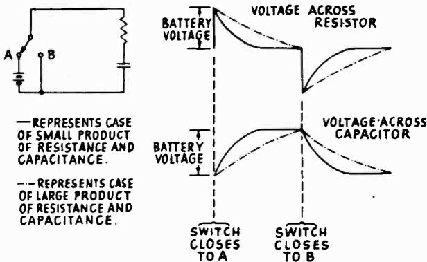
FIG. 8-2, above.—Sync separator circuit consisting of a resistor and capacitor in series. The voltages that appear across each when the capacitor is charged from a battery and then discharged, in both cases through the resistor, are shown at the right.
