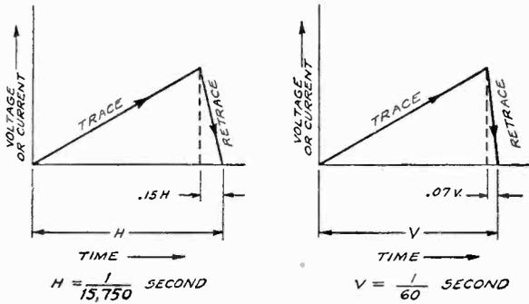
Fig. 1-16.—At the left is shown the saw-tooth waveform required for horizontal scanning. A similar waveform, but of much lower frequency is required for vertical deflection and is shown on the right.
