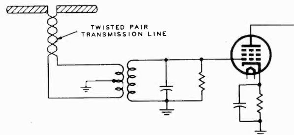
FIG. 3-10.—In order to match the impedance of a half-wave dipole antenna with that of the transmission line, the latter can be formed of twisted pair, which has a characteristic impedance of approximately 75 ohms.
