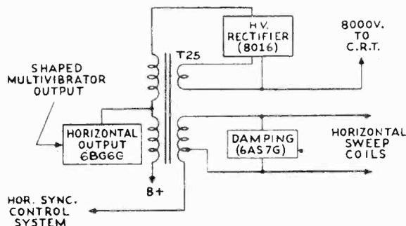
FIG. 11-8.—The "kick-back" type of power supply such as is used in the G.E. model 802. Here the rectifier plate voltage is obtained from the horizontal deflection system during the fly-back periods.
