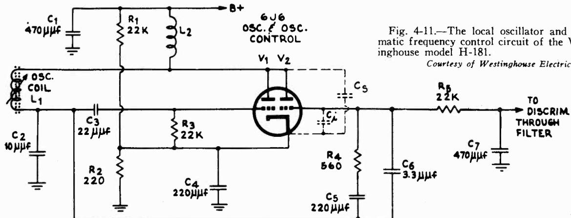
Fig. 4-11.—The local oscillator and automatic frequency control circuit of the Westinghouse model H-181.
