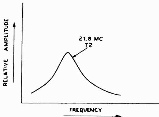
FIG. 6-9.—Response curve for the first video i-f stage which is peaked at a frequency of 21.8 mc.
