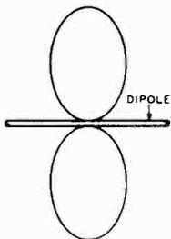
FIG. 3-21.—The ideal field pattern of a half-wave dipole. Note that each side of the pattern is identical.
