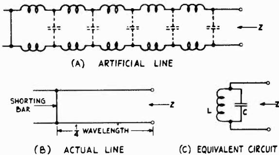
Fig. 4-8.—The artificial resonant lines used as tank circuits in the RCA model 621TS are shown in (A). The physical line which (A) replaces, is shown in (B) and the equivalent circuit in (C).
