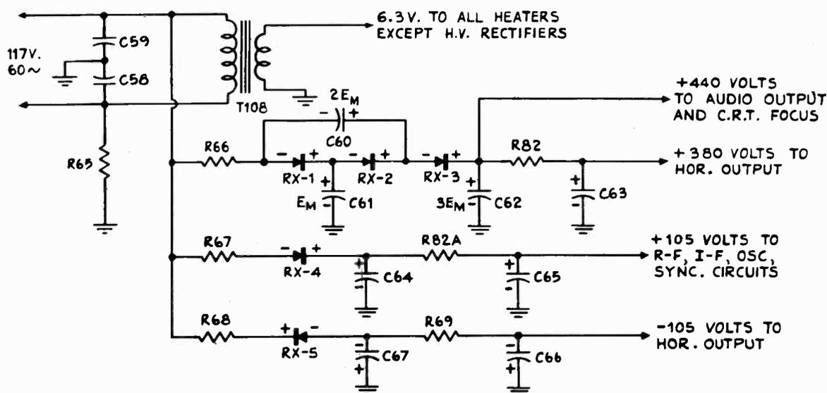
FIG. 11-4.—The low-voltage power supply of the Consolidated Television model 2315. Note the use of the selenium rectifiers.
