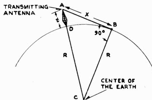
FIG. 3-2.—The horizon range is the distance between points  $A$  and  $B$ . The horizon range from the transmitting antenna and the horizon range from the receiving antenna can be added together to obtain the line of sight.
