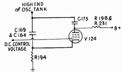
FIG. 8-11. — Simplified circuit of reactance tube used in RCA model 630TS.
