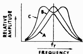
FIG. 6-2.—Response curves for different coefficients of coupling: A low coefficient produces the single-peaked curve *A*. The broader curve *B* has reached the critical point beyond which any increase in the coefficient produces a still broader but double-peaked curve *C*.
