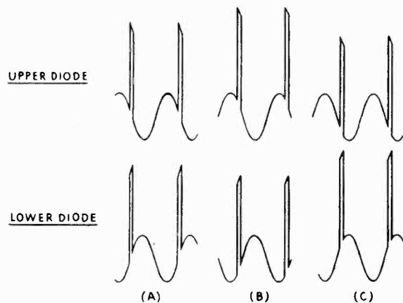
FIG. 8-12.—Combined sync pulse and sine-wave signals at the diode plates when (A) the natural frequency of the horizontal oscillator is correct, (B) the natural frequency is low, and (C) the natural frequency is high. In (B) and (C) the shift of the pulses with respect to the sine waves has been exaggerated to make it more apparent.
