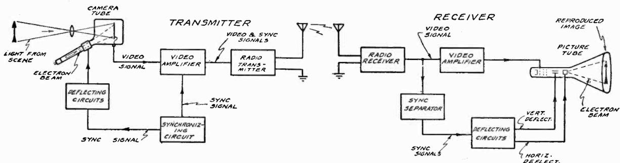
Fig. 1-17.—The principal elements of a complete television system. Note the provision made for synchronizing the scanning at the picture tube with that at the camera tube.
