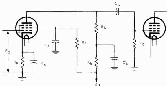
FIG. 7-4.—Typical low-frequency compensated  $RC$  coupled amplifier. The decoupling network  $R'_bC'_b$  has been added to the circuit of Fig. 7-3 to better the low-frequency response.
