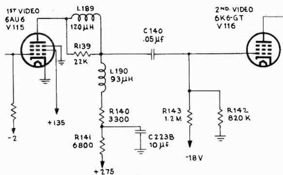
FIG. 7-13.—The first video amplifier circuit of the RCA model 630TS receiver.
