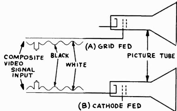
FIG. 6-26.—For correct operation of the picture tube the black parts of the video signal should drive the grid more negative and the white parts, less negative. Depending upon the polarity of the signal, it may be fed to either the grid (A) or the cathode (B) of the tube.
