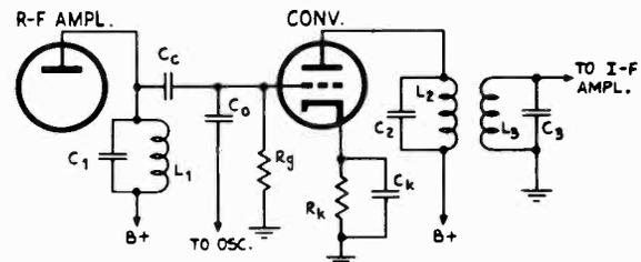
Fig. 4-3.—Simplified schematic of a converter (mixer) stage.
