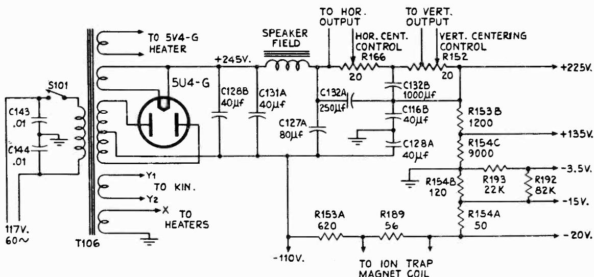
FIG. 11-1.—The low-voltage power supply circuit used in the RCA model 621TS receiver.
