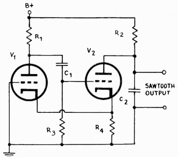
FIG. 9-5.—The Potter sweep circuit. The output of the left-hand amplifier is fed to the grid of the second amplifier  $V_2$ , which functions as a cathode follower, as far as its output that is fed to  $V_1$  is concerned.
