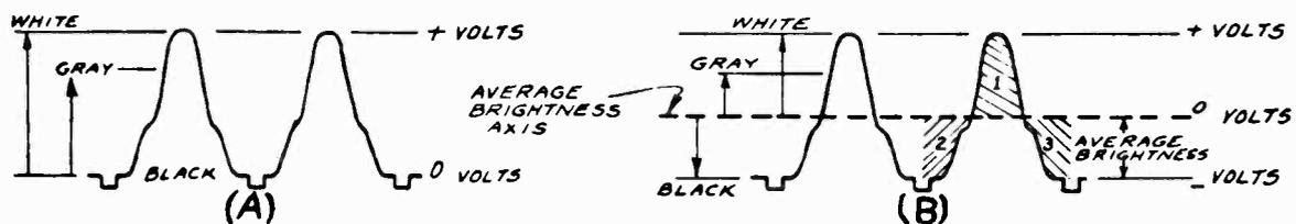
FIG. 7-14.—The light values in a video signal can be reckoned in two ways as here illustrated: in (A) the various light values are referred to the black level; in (B) the same light values are referred to the average brightness of the signal.
