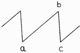
FIG. 11-9.—The current in the sweep coils must have a saw-tooth form, *a-b* being the trace period and *b-c* the retrace.
