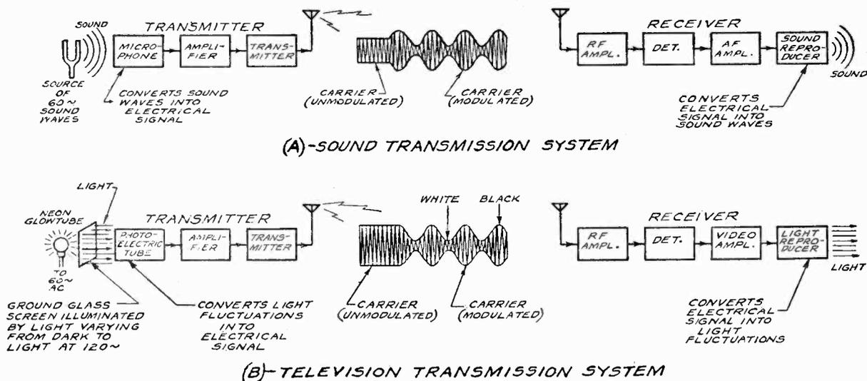
Fig. 1-1.—Part (A) shows an a-m sound transmission system and (B) shows a television transmission system. In the television system the photoelectric tube replaces the microphone and the light reproducer replaces the speaker.
