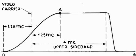
Fig. 2-6.—The over-all bandwidth characteristics of the video channel.
