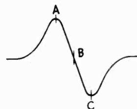
FIG. 12-3.—The response curve of the sound section obtained at the output of the discriminator. A, B, and C are pips obtained from the marker generator.
