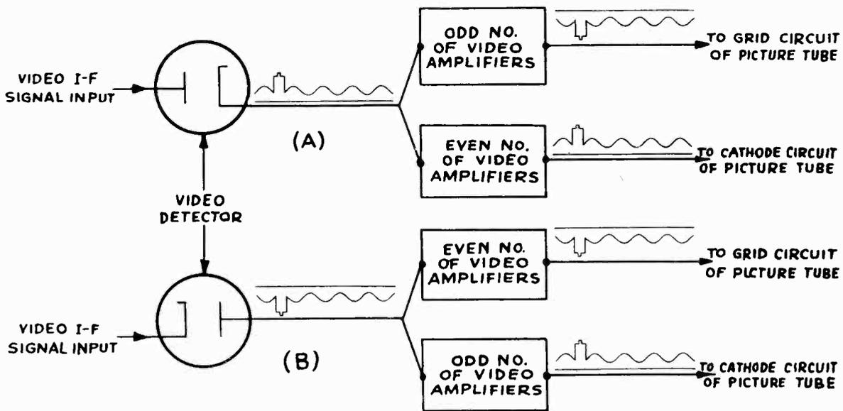
FIG. 6-27.—These various circuit arrangements are possible in the video section when the video signal output is fed to the picture tube from the plate circuit of the last video amplifier. The video modulating signal is assumed to be a sine wave.
