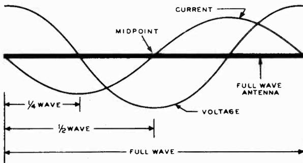
FIG. 3-3.—A full-wavelength straight-wire antenna with standing current and voltage waves. Note that at the midpoint of the antenna the current is a minimum and the voltage a maximum.
