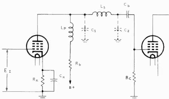
FIG. 7-11.—A typical circuit combining the effect of series and shunt peaking with the shunting capacities  $C_1$  and  $C_2$  indicated across the coil  $L_s$ .
