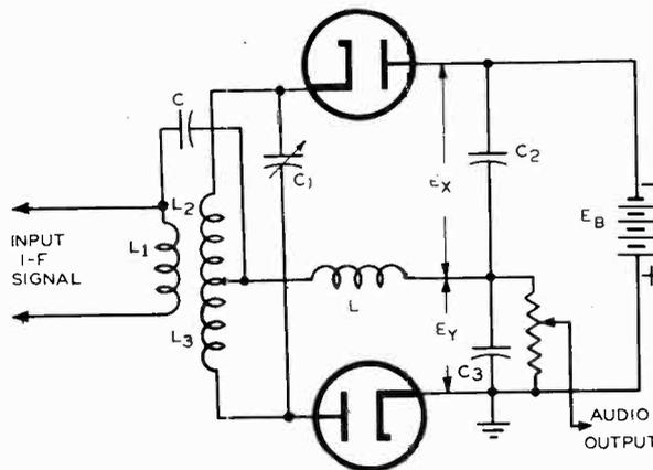
Fig. 5-25.—Simplified schematic of a ratio detector circuit. Note that the diodes are connected in *series aiding* rather than *series opposing* as in the discriminator detector.
