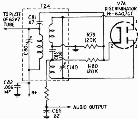
Fig. 5-20.—The discriminator circuit used in the General Electric model 802.
