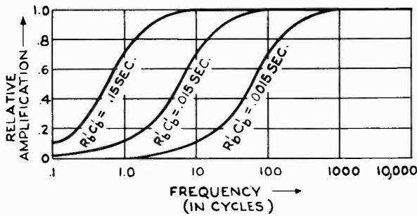
Fig. 7-5.—The effect of inserting different values of the  $R'_b C'_b$  network is shown. As the time constant of the decoupling network is increased, the low-frequency response increases.
