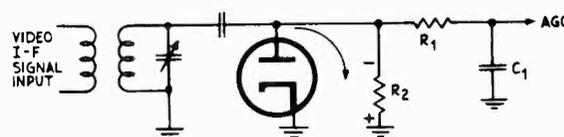
FIG. 6-23.—Due to the direction of the current flow in this simple agc circuit (indicated by arrow), the potential on  $R_2$  will be negative with respect to ground, presenting a ready point for tapping of agc.
