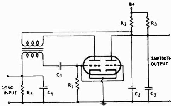
FIG. 9-7.—The addition of the second triode in this blocking oscillator enables the production of a saw-tooth wave having a large amplitude and rapid retrace.
