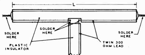
FIG. 3-13.—Construction details of a folded dipole antenna made from a 300-ohm twin-lead transmission line.
