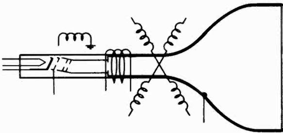
FIG. 10-5.—In order to get rid of the negative ions in the electron stream, the "gun" is placed at an angle so that the ions are aimed at one side of the anode while a bending coil causes the ion-free electrons to turn and go along the axis of the tube.
