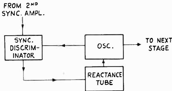
FIG. 8-6.—Block diagram of sweep afc circuit as used in RCA model 630TS. In this circuit the pulses from the second sync amplifier are of primary importance in determining the output from the discriminator.
