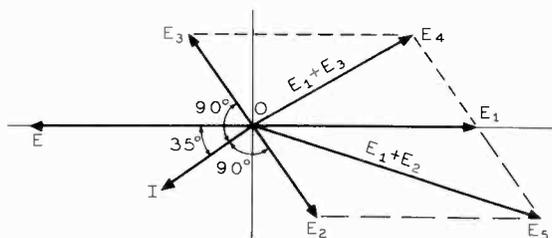
Fig. 5-14.—When the instantaneous frequency of the f-m signal is lower than the resonant frequency of the transformer, the current  $I$  will lead the induced voltage  $E$ . Compare with Figs. 5-12 and 5-13.
