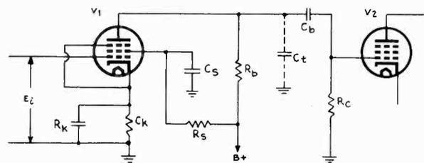
FIG. 7-3.—Typical  $RC$  coupled amplifier.
