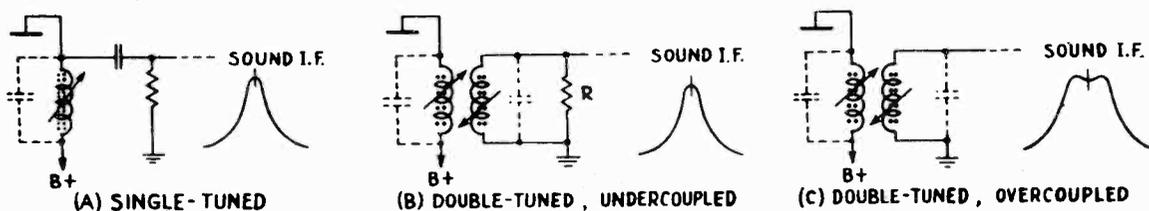
FIG. 12-2.—The coupling circuits in the sound i-f section may be single- or double-tuned as indicated above. Note the similarity between the response curves of (A) and (B) and how the overcoupling of the double-tuned circuit in (C) results in a widened response curve.
