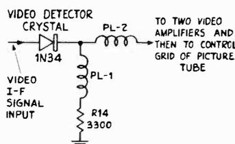
FIG. 6-34.—In the Consolidated Television model 2315 a 1N34 germanium crystal is used as a video diode detector.
