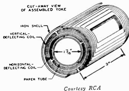
Fig. 1-9.—The magnetic deflecting yoke contains the horizontal and vertical deflection coils which are designated here.
