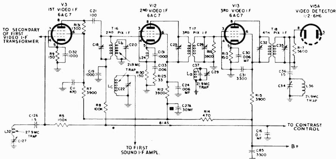
FIG. 6-16.—Schematic diagram of the video i-f section of the GE model 802 showing the five individual traps employed in this receiver.
