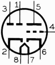
Fig. 5-21 (left) — Schematic of the 6AQ7-GT duo-diode high-mu triode tube.
