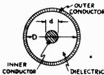
FIG. 3-8.—Cross-sectional view of a coaxial transmission line.  $D$  is the inner diameter of the outer conductor and  $d$  is the outer diameter of the inner conductor.
