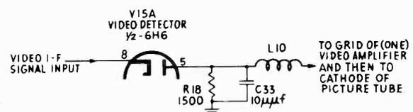
FIG. 6-33.—The video detector circuit of the GE model 802 feeds the video i-f signal through one video amplifier to the cathode of the picture tube.
