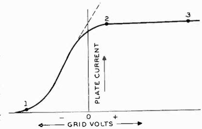
number of special operating conditions are combined to make the limiter function properly. First, the amplifier tube used is usually of the sharp cut-off type like the 6SJ7 or 6SH7 tubes or the miniature type 6AU6 tube. Low values of screen and plate voltage and little or no initial control grid bias are applied to the tube, so that it will quickly overload and plate current cutoff will be rapidly reached.
