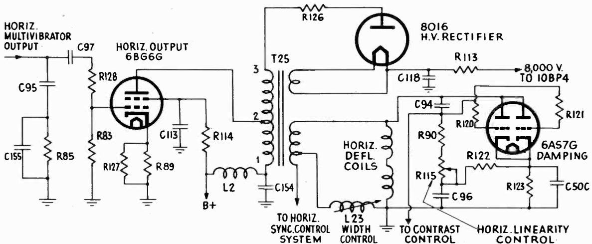
FIG. 11-11.—Schematic diagram of the high-voltage supply circuit of the G.E. model 802. The block diagram of this circuit is shown in Fig. 11-8.
