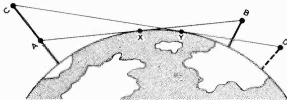
FIG. 3-1.—The line of sight is shown between two antennas at *A* and *B*. If the antenna *A* were raised to position *C*, the line of sight would be extended to *D*.
