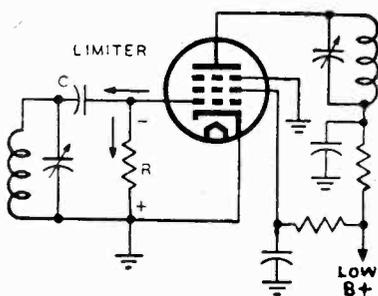
Fig. 5-5—The  $RC$  combination determines how quickly grid bias on the limiter tube will occur, thus causing automatic bias regulation.
