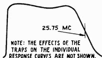
FIG. 6-14.—The over-all curve for the entire stagger-tuned system is shown to be fairly flat and capable of covering the necessary bandwidth. The 25.75 mark indicates the position of the video i-f carrier.
