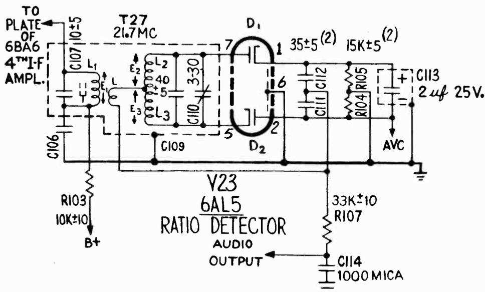
Fig. 5-27.—Modified ratio detector circuit as used in the Andrea television chassis VJ12. Courtesy Andrea Radio Corp.
