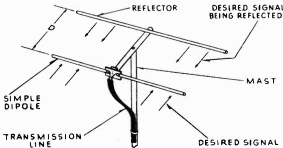
FIG. 3-14.—In order to increase the pickup, a reflector element is placed behind the dipole in the same plane at a distance  $D$ , that is between one-tenth and one-quarter of the wavelength for which the dipole is cut.
