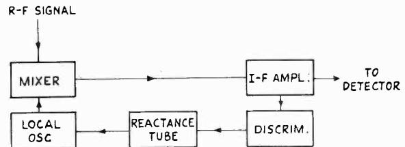
FIG. 8-7.—Block diagram of type of afc scheme used for correcting errors in superheterodyne tuning. In contrast with the circuit of Fig. 8-6, the oscillator does not feed the discriminator directly, and, more important, there is only one input to the discriminator.
