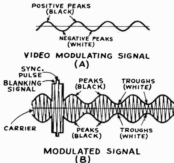
FIG. 6-25.—How negative transmission is used for television is here illustrated by representing the video signal as a sine wave. In (A) the positive peaks are the black regions of the picture and the negative peaks are the white regions. In (B) the peaks represent the black regions and the troughs the white regions.
