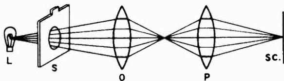
FIG. 10-2.—An optical system which is analogous to the elements of a cathode-ray tube which bring the electron stream to a focus on the screen.
