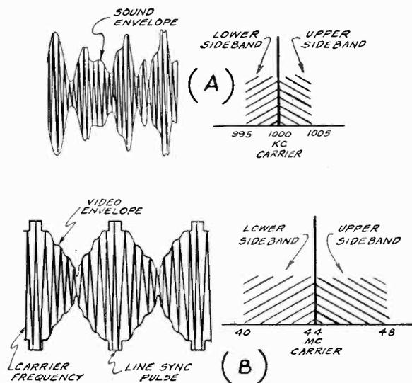
Fig. 1-22.—The sidebands in an a-m sound signal occupy a bandwidth of only about 10 kc, whereas the sidebands in a television signal require a bandwidth of about 8 mc.
