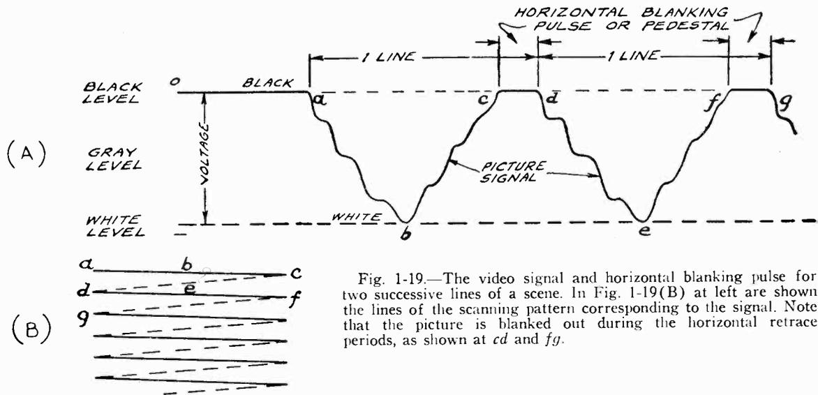
Fig. 1-19.—The video signal and horizontal blanking pulse for two successive lines of a scene. In Fig. 1-19(B) at left are shown the lines of the scanning pattern corresponding to the signal. Note that the picture is blanked out during the horizontal retrace periods, as shown at *cd* and *fg*.
