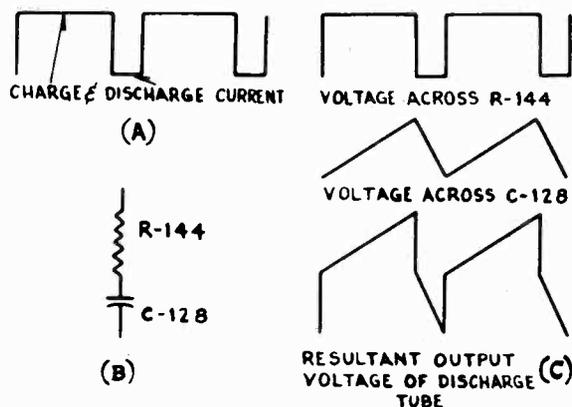
FIG. 9-11.—When a rectangular current wave (A) is applied to a resistor and capacitor in series (B), the individual waveforms are as shown in (C) with the resultant waveform at the bottom.
