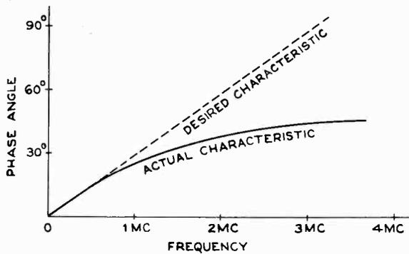
FIG. 7-2.—The dotted line represents the desired linear phase shift and the solid line represents the actual phase shift as it varies with frequency.
