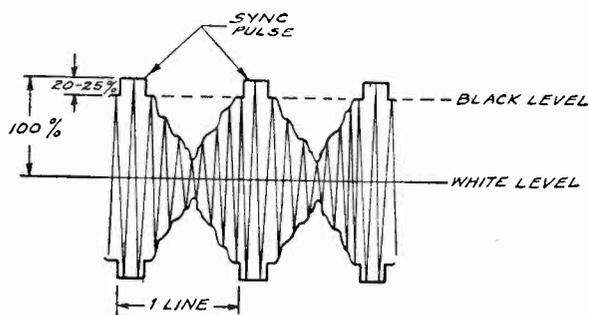
Fig. 1-23.—A video wave with negative modulation. The sync pulses are located in the blacker-than-black region and occupy from 20 to 25 percent of the maximum carrier amplitude.
