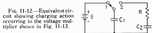
FIG. 11-12.—Equivalent circuit showing charging action occurring in the voltage multiplier shown in Fig. 11-13.
