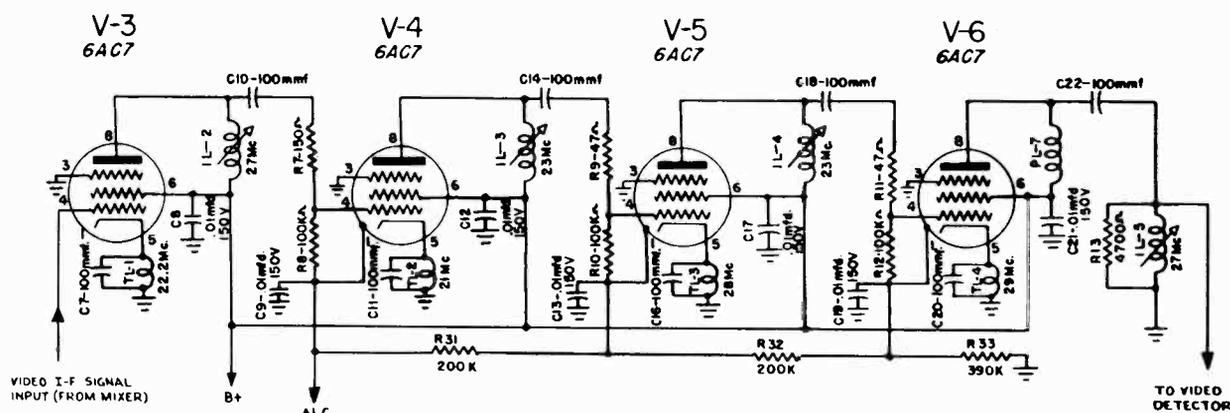
FIG. 6-19.—In this Consolidated Television model 2315, all the traps employed are situated in the cathode circuits of the video i-f amplifiers.
