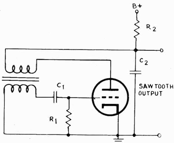
FIG. 9-6.—A saw-tooth wave is obtained from the plate circuit of this blocking oscillator and very sharp pulses may be derived from the grid circuit.
