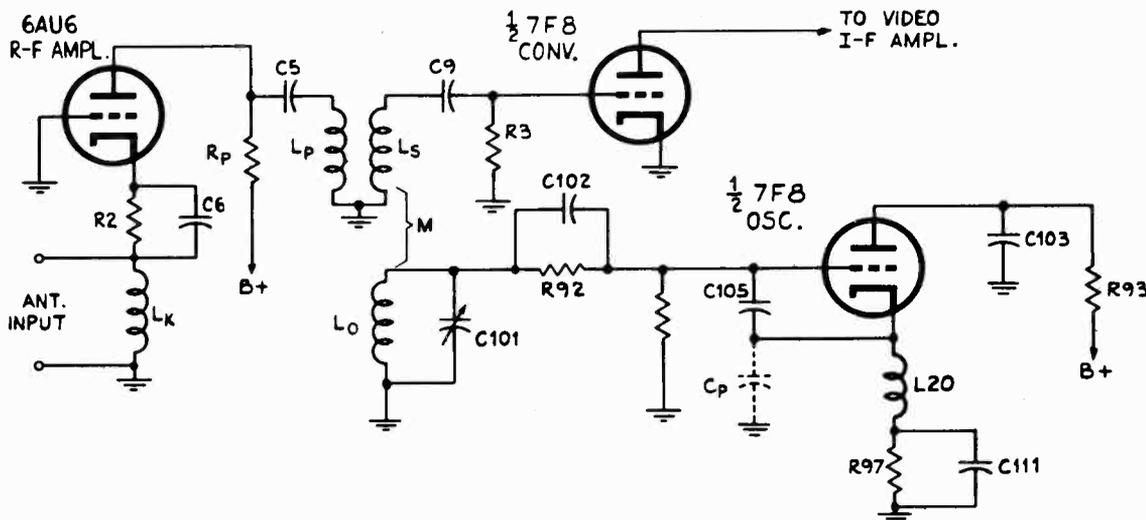
Fig. 4-6.—The r-f amplifier, converter, and oscillator of the GE model 802.
