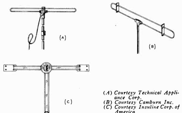
FIG. 3-12.—Three types of folded dipole antennas. Those illustrated in (A) and (B) are for outdoor use and that in (C) is for indoor or outdoor use.
