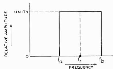
Fig. 5-1.—An ideal selectivity curve that is flat-topped would pass all frequencies between the limits  $f_a$  and  $f_b$  with equal amplitude; such a curve cannot be realized in practice with the use of a single i-f transformer network.
