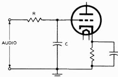
Fig. 5-16.—A typical de-emphasis network as used in the sound section of television receivers.
