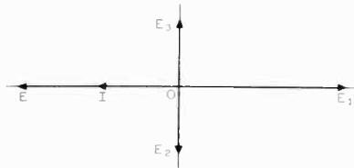
Fig. 5-10. — Revised vector diagram of Fig. 5-9. Note that the vector  $OE_3$  is shifted  $180^\circ$  in phase from its position in the previous figure.
