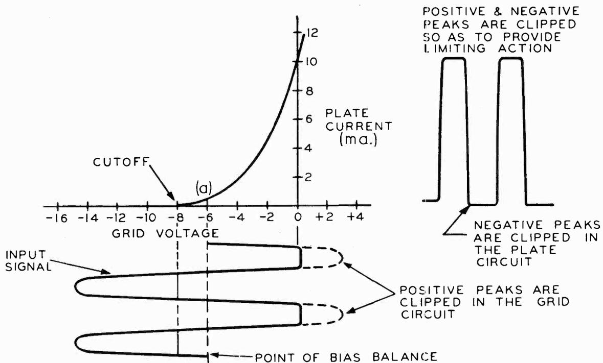
Fig. 5-6.—The clipping action of the input signal to the limiter circuit of Fig. 5-5 is illustrated in the characteristic curve shown here.
