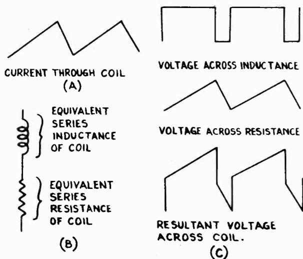
FIG. 9-10.—When a saw-tooth current (A) flows through a coil, the combined waveforms of the voltages due to the inductive and resistive properties of the coil (B) produce the resultant waveform shown at the bottom of (C).
