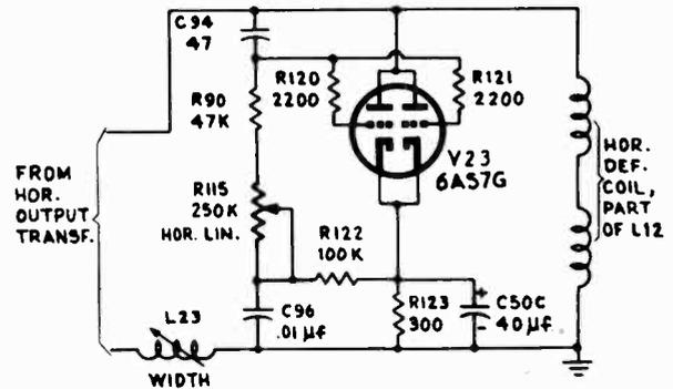
FIG. 9-13.—The damping tube and its associated components in the horizontal sweep circuit of the GE model 802.
