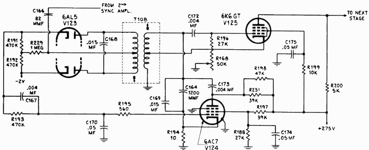
FIG. 8-8.—Complete schematic diagram of the horizontal sweep oscillator and its associated afc circuit used in the RCA model 630TS.
