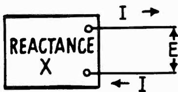
FIG. 8-10. — This closed box having two terminals and containing an unknown circuit illustrates in a simple way how it is possible to obtain a controllable reactance using a pentode tube.
