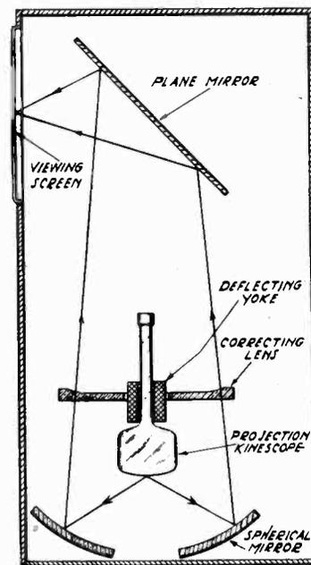
FIG. 10-6.—The optical system of a projection television receiver, which employs the principles originated by Schmidt for use in telescopes. The image of the picture on the screen of the picture tube is reflected upward by the spherical mirror going through the correcting lens into the inclined mirror. From here it is reflected onto the viewing screen.
