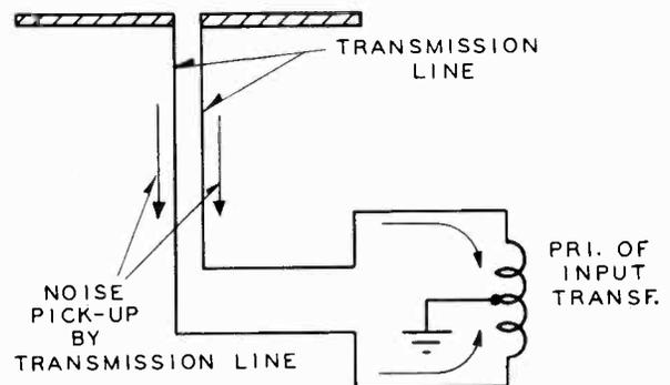
FIG. 3-20.—In order to reduce noise pickup through the medium of the transmission line, the center of the primary winding of the r-f transformer is grounded. This increases the signal-to-noise ratio at the input of the receiver.
