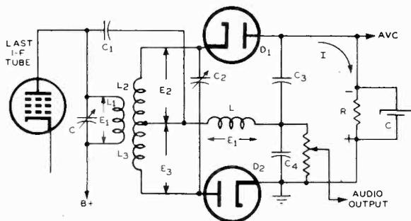
Fig. 5-26.—A typical ratio detector circuit. A parallel RC network has replaced the battery of Fig. 5-25 in the output of the circuit.
