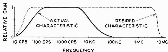
FIG. 7-1.—The solid line represents the bandwidth of an audio amplifier. The dotted line represents the desired bandwidth of a video amplifier.
