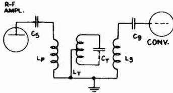
Fig. 4-7. — The triple-tuned coupling circuit used for channels 1 and 2 in the GE model 802.
