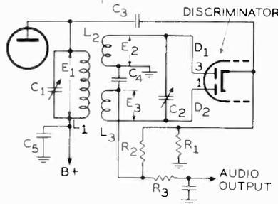
Fig. 5-22 (right) — The discriminator circuit of Fig. 5-20 has been redrawn to show the use of the 6AQ7-GT more clearly.
