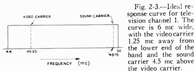
Fig. 2-3.—Ideal response curve for television channel 1. The curve is 6 mc wide, with the video carrier 1.25 mc away from the lower end of the band and the sound carrier 4.5 mc above the video carrier.
