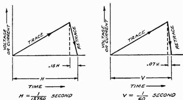
FIG. 9-2.—At the left is shown the saw-tooth waveform needed for horizontal scanning and on the right, the waveform for vertical scanning. While the "trace" voltage is applied to the deflecting system, the screen is illuminated, but during "retrace," it is blanked out.
