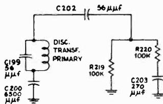
Fig. 5-19.—The two paths of Fig. 5-18 from the top of the discriminator primary coil to ground are redrawn for the sake of the discussion.
