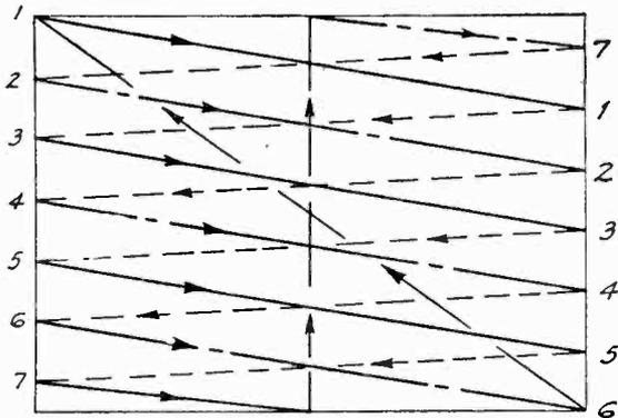
Fig. 1-15.—An interlaced scanning pattern in which the odd and even lines are scanned on successive fields.
