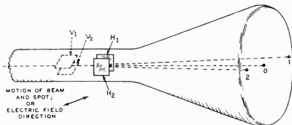
FIG. 10-4.—If horizontal deflection plate  $H_1$  be made positive and  $H_2$  negative, the spot will move to the right from the center of the screen O to point 1. When the polarity of the voltages is reversed, the spot will move toward point 2.
