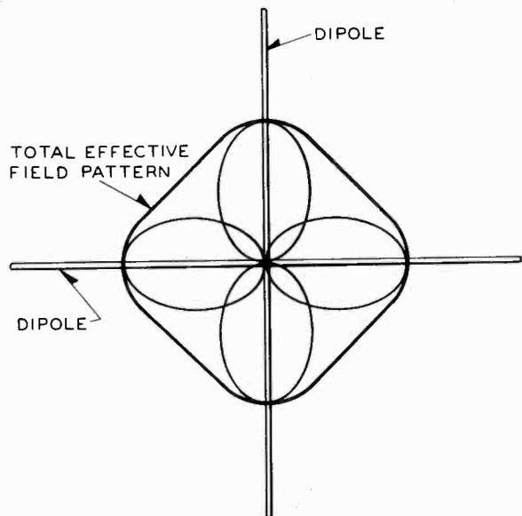
FIG. 3-29.—The total effective field pattern of two crossed dipoles is virtually circular in shape.
