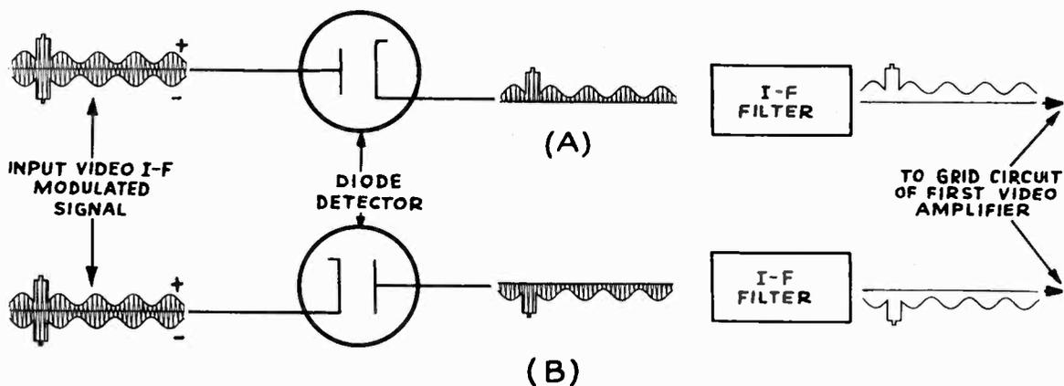
FIG. 6-28.—How the phasing of the video modulated signal is controlled by the diode detector is shown here. In (A) the signal is fed to the plate of the diode rectifier which will conduct only when the plate is more positive than the cathode. That is, only that part of the signal above the reference line will cause the diode to conduct. When, as in (B), the signal is fed to the cathode of the detector, the reverse is true.
