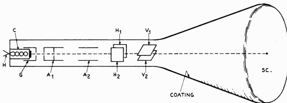
FIG. 10-1.—The elements of a cathode-ray tube:  $H$  is the heater;  $C$  the cathode;  $G$  the control grid;  $A_1$  and  $A_2$ , the first and second anodes respectively;  $H_1$ ,  $H_2$  and  $V_1$ ,  $V_2$ , the horizontal and vertical deflection plates, respectively; and  $SC$ , the screen.
