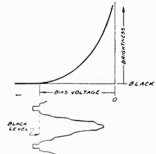
FIG. 7-18.—The effect of bias voltage on the brightness of the image. The brightness control should be adjusted so that the black level on the signal occurs approximately at the cutoff of the picture tube characteristic.
