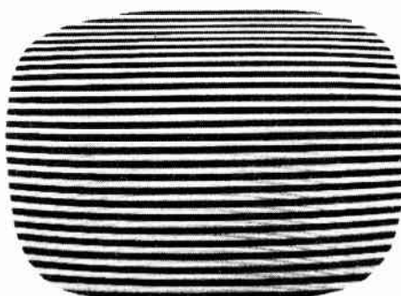
Fig. 5. 1500-cycle modulation with poor vertical linearity.
