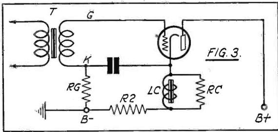
This is a simplified version of the first section or input of the Triple-Twin tube. It will better serve to clarify the action of this part of the tube as an amplifier. The function of the resistor Rg is to supply bias to the grid
