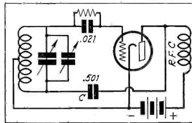
**Fig. A. Circuit of a capacity-coupled Hartley oscillator**
