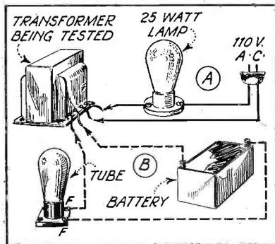
Showing simple methods of locating the respective windings of a power transformer
