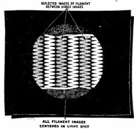
Fig. 1. This shows the correct projector lamp filament images
