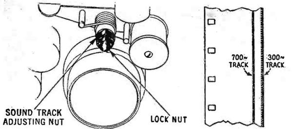
Fig. 4. (left) This sketch shows the pressure roller adjusting screws referred to in the text. Care should be taken in tightening the lock nut. Fig. 5. (right) A section of Buzz Track Film, which carries sound tracks of 300 and 700 cycles
