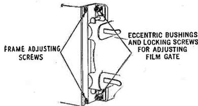
Fig. 6. Showing the location of screws for adjusting film gate and frame
