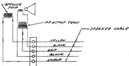
Fig. 2. In some of the models a five-lug speaker terminal board is used. The correct connections, as well as the color coding, is shown in the above diagram
