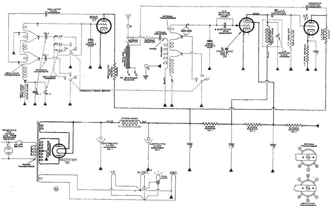
The schematic diagram of the Atwater Kent Model 93 Short-Wave Converter, with its attendant power unit. An intermediate frequency of 1,000 kc. is employed. Note that tapped coils are used in connection with a series of condensers to effect a change of waveband. The lettering on the terminals of the antenna and oscillator transformers, as shown in the right hand corner, correspond to the lettering in the circuit diagram above. (Courtesy, Atwater Kent Mfg. Co.)
