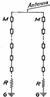
**Fig. 1. Manner of connecting Multicouplers when two downloads are used. Maximum, thirty Multicouplers**
