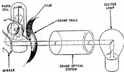
Fig. 2. View of the sound system. Note the slits through which the light must pass
