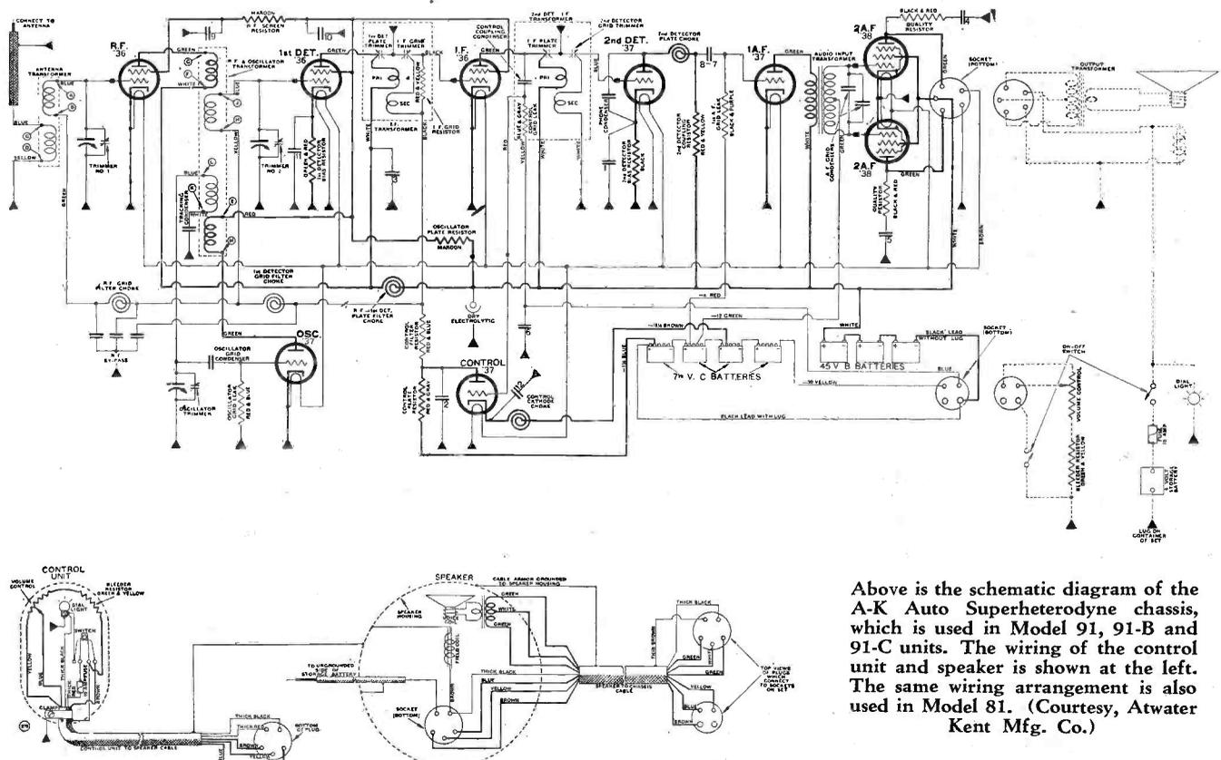
Above is the schematic diagram of the A-K Auto Superheterodyne chassis, which is used in Model 91, 91-B and 91-C units. The wiring of the control unit and speaker is shown at the left. The same wiring arrangement is also used in Model 81. (Courtesy, Atwater Kent Mfg. Co.)
