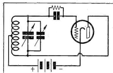
**Fig. B. Circuit of the conventional Hartley oscillator**
