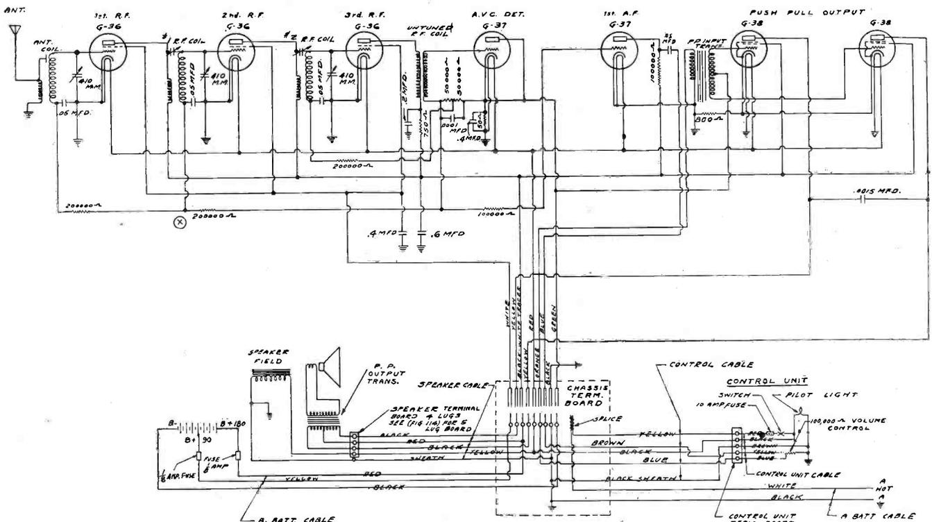
Fig. 1. Circuit diagram of the Majestic Model 110 Auto Radio. Note that this chassis utilizes an automatic volume control system in combination with a diode detector, the G-37 tube serving both functions. (Courtesy, Grigsby-Grunow Co.)
