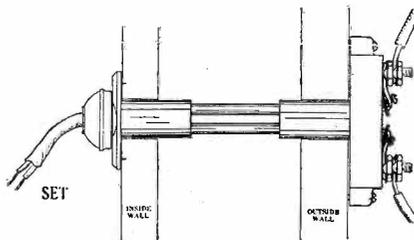
That section of the Super-Thru which is mounted on the outside wall is both the connecting link for the aerial and ground, and a resistance-type lightning arrester.
