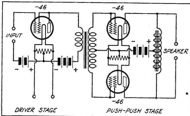
Diagram of a Class B amplifier, employing three of the new type '46 tubes. Note that there is no bias placed on the tubes in the "push-push" stage
