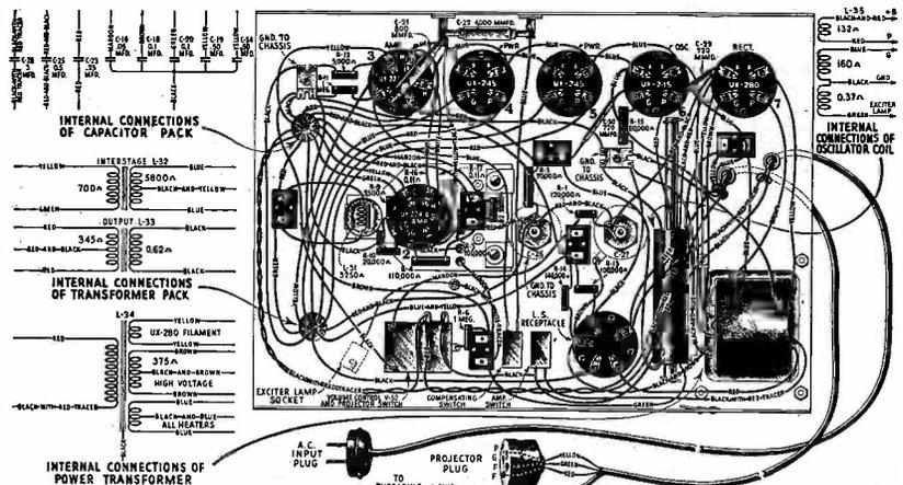
Wiring diagram of the amplifier unit of the RCA, PG-38 Home-Talkie Outfit
