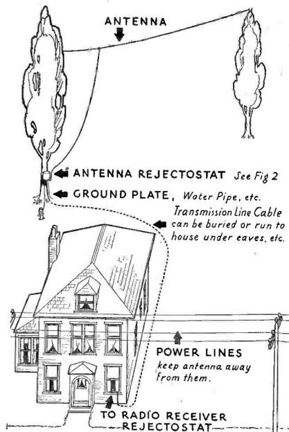
Fig. 2. A typical installation. The aerial should be free of power lines, etc., and free of any obstructions
