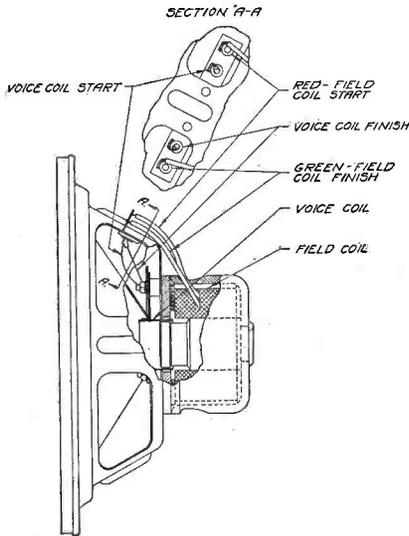
Color-coded connections to the G-1503, 400-ohm field, dynamic speakers in the Clarion AC-280 and 25-280 receivers
