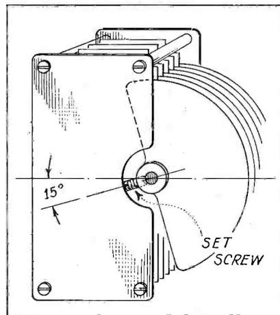
An odd case: The set screw on the rotor shaft became loose and touched the stator section when about 15 degrees below the center line, as shown
