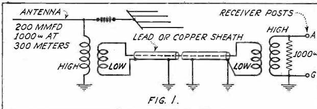
Here are the details of a typical noise-reducing transmission line, using shielded lead-in wire in connection with two impedance-matching transformers. The 1000-ohm termination resistance across the aerial and ground posts of the receiver is used only with low-impedance inputs
