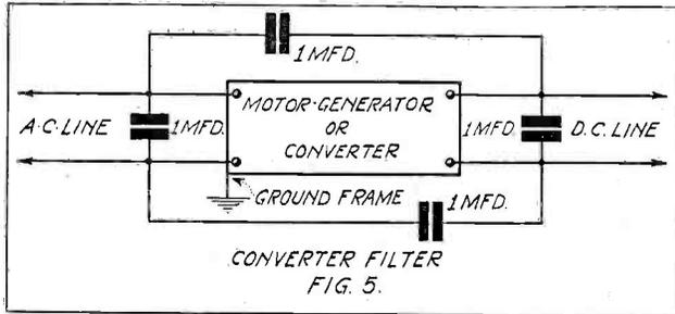
A very effective arrangement for use with motor-generators and converters. Note that the frame of the machine is grounded
