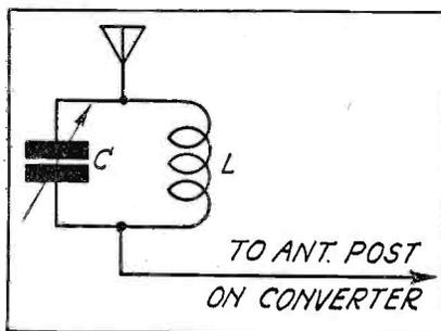
This form of wave trap is satisfactory for the elimination of an interfering signal of broadcast frequency which falls on the i-f. frequency of the short-wave converter. The coil and condenser should be mounted in a shield
