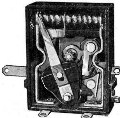
duction remains the same for all volume control settings. The new tapped Bradleyometer achieves this result in any one of several audio-frequency networks and automatically accomplishes tone correction with volume changes.
