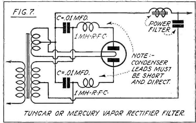
The effectiveness may be increased by the addition of condensers. The r-f. chokes and rectifier tube should be enclosed in a grounded shield, as in Fig. 6
