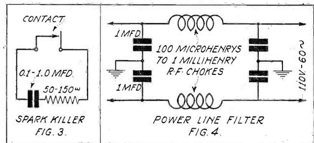
The arrangement shown in Fig. 3 is effective for most any type of make-and-break circuit. The circuit of Fig. 4 will quell line surges
