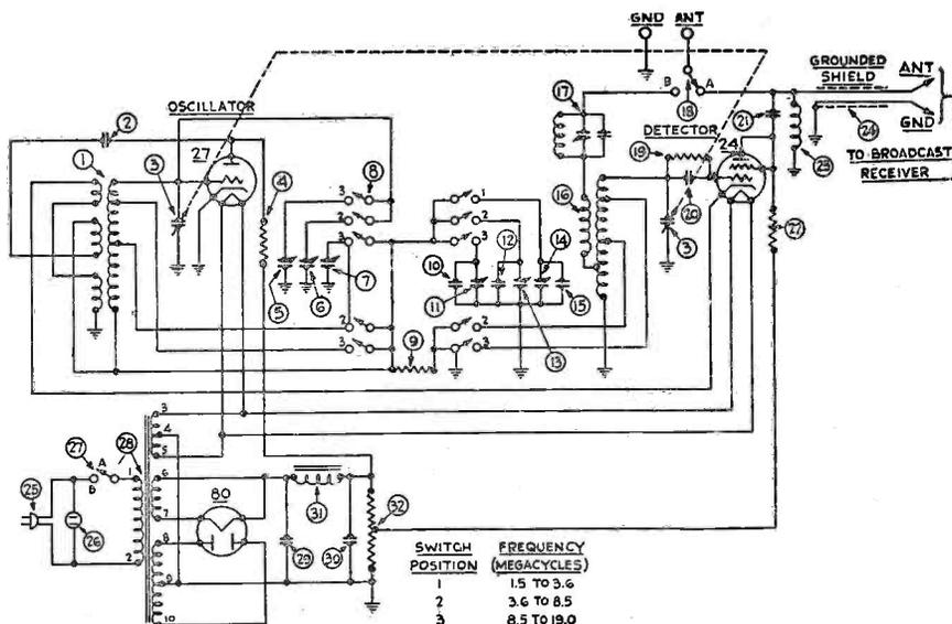
Schematic diagram of the Philco 4 and 4C Short Wave Converter. The numbers in this diagram correspond to the numbers on the chassis and in the parts list on the opposite page. The voltage data for the three tubes is given in Table 1
