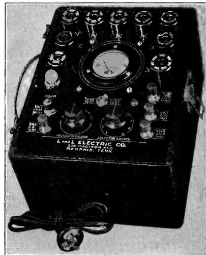
The L & L Model E-33 Tube Tester. This instrument also contains an oscillating circuit which can be used for other purposes aside from tube testing
