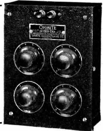
The DETERM-OHM is a necessary part of the modern service man's equipment. By connecting it in place of a defective resistor and adjusting the dials, the value of the correct replacement unit is easily determined. It has many other applications in the service field. The cost of the DETERM-OHM is surprisingly low. See it at your jobbers or write for Bulletin D-2 for complete details.
