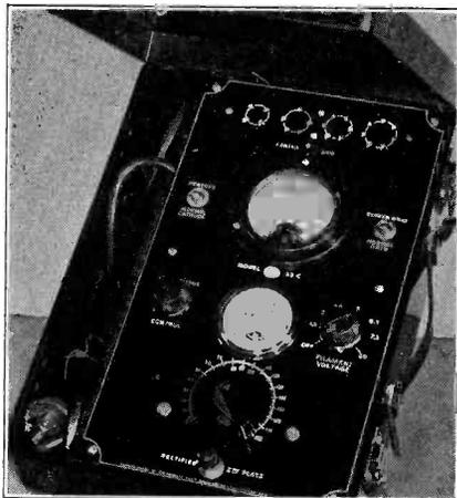
The Franklin Model 33-C English Reading Tube Checker, which uses a single scale meter for all tests. The tube sockets are at the rear
