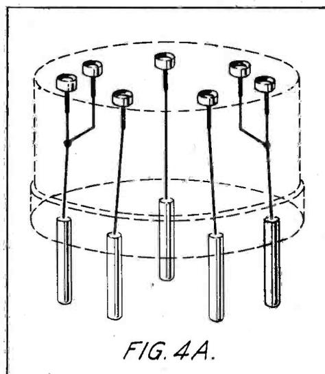
This illustrates the adapter connection when the seven-pin tube is arranged for test as a '27
