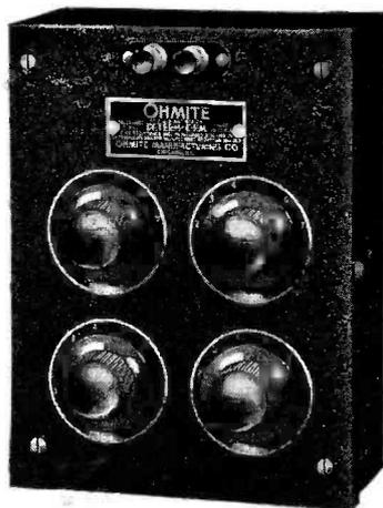
found that the resistor in a receiver has been completely destroyed, and that it is impossible to read the value of the unit or measure it. In such a case, the "Determ-Ohm" is connected in place of the defective resistor and the radio set turned on. The dials on the "Determ-Ohm" should be set at the maximum resistance before the set is operated and then the resistance is gradually reduced until the set functions properly. Then, a glance at the dials shows the proper replacement resistor value.
