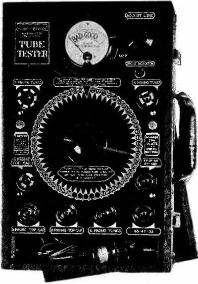
Above: The Confidence English-Reading Tube Tester. The large scale carries the type numbers of the different tubes which can be tested. Five blank spaces are left for new tube numbers
