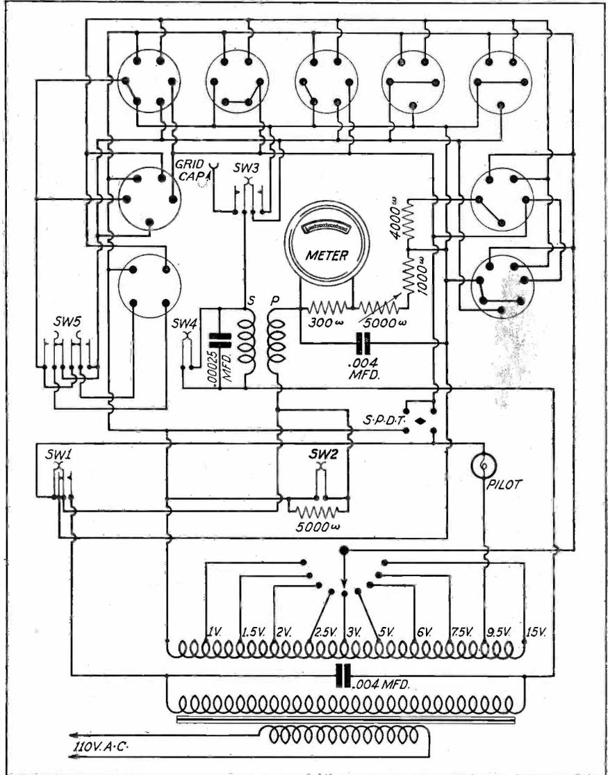
Below: The schematic diagram of the Confidence English-Reading Tube Tester. Note that tube filament voltages are altered automatically
