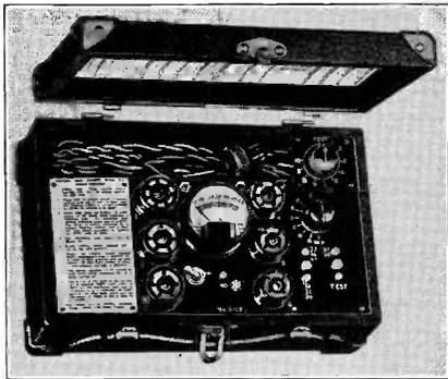
Front panel view of Readrite No. 407 Tube and Short Tester. The rotary switch to the right provides short tests
