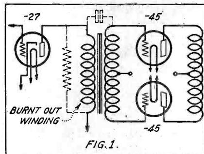
Here is a simple little stunt for temporarily repairing an audio circuit when the primary of the transformer opens. A resistor and coupling condenser keeps the set going until a transformer can be obtained
