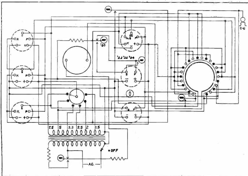
The schematic diagram of the Readrite No. 407 Tube Tester illustrated above. This shows the connections for the special rotary switch which provides short tests
