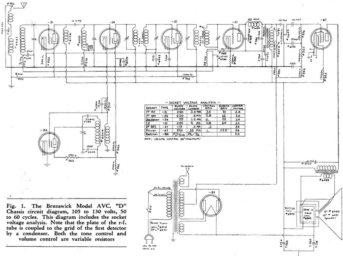
Fig. 1. The Brunswick Model A.V.C. "D" Chassis circuit diagram, 105 to 130 volts, 50 to 60 cycles. This diagram includes the socket voltage analysis. Note that the plate of the r-f. tube is coupled to the grid of the first detector by a condenser. Both the tone control and volume control are variable resistors
