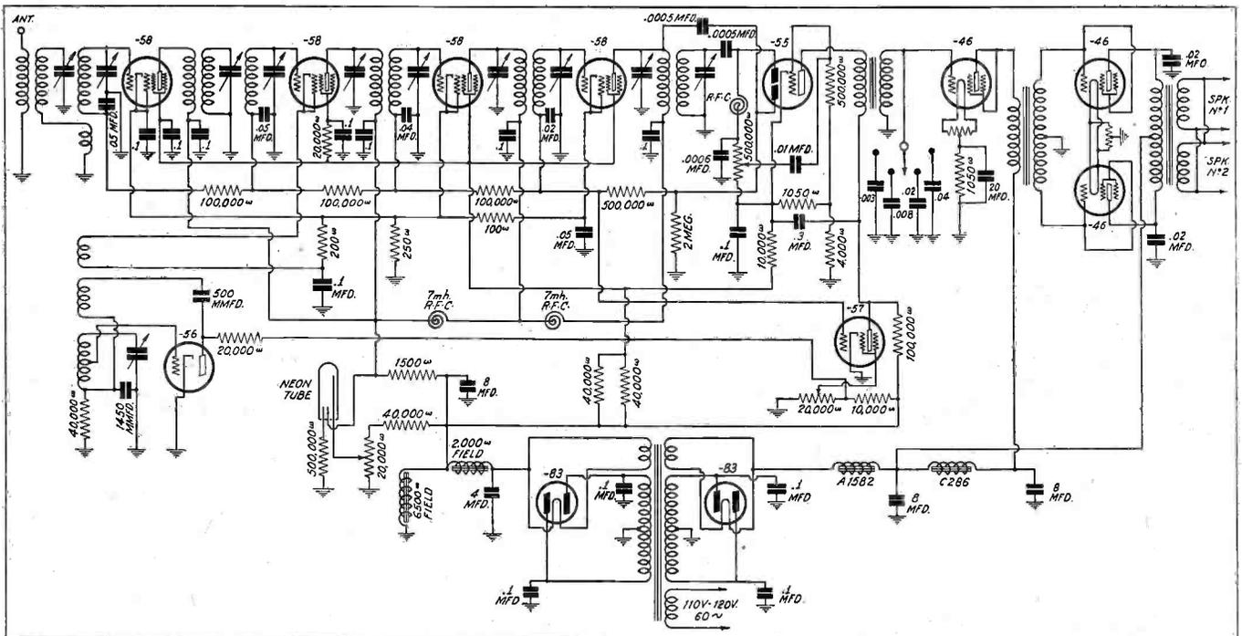
The diagram of the Atwater-Kent Model 612. This is practically the same as the Model 812, with different values for some of the units and slight circuit alterations. For example, in the Model 812 the two speaker field coils obtain their exciting current from the same rectifier that supplies the audio amplifier, while in this model just the reverse holds true
