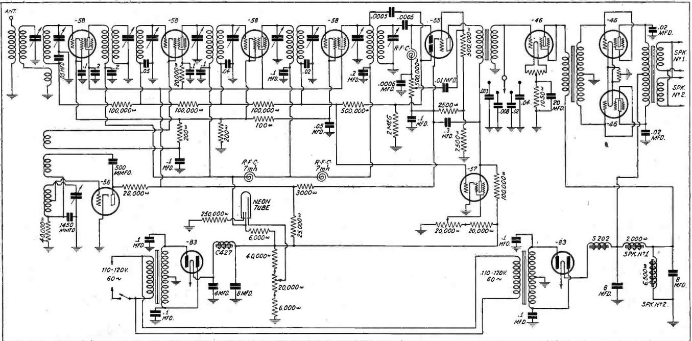
The complete schematic diagram of the Atwater-Kent Model 812 superheterodyne, including all resistance and capacity values. The first tube is an r-f. amplifier, second tube is first detector, the next two are i-f. amplifiers and the fifth tube a type 55 duo-diode AVC second detector. The type 57 tube just below the type 55 provides the silent tuning feature of the set
