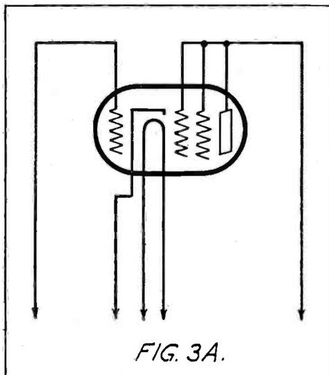
This illustrates the equivalent diagram of the tube circuit with the links shown in Fig. 3
