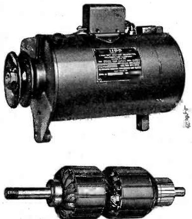
Both a d-c. and a-c. armature are wound on the same shaft. The d-c. end of the generator is of the shunt type, and when running at 1,000 R.P.M. is so designed that it will generate 6 to 8 volts for charging the car storage battery. The a-c. end is of the armature type, and when running over 1,000 R.P.M. will produce 110 volts a-c. and hold the voltage constant.
