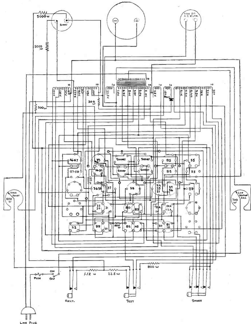
This is the schematic diagram of the Weston-Jewell Model 676 Tube Seller. The diagram of the Model 677 is identical, except that some of the extra sockets shown are wired in for use. The short indicator in this instrument is a neon lamp
