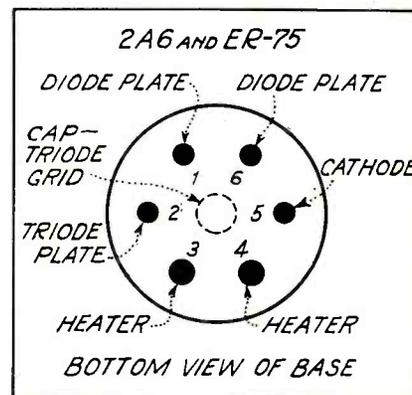
Fig. 6. Base connections for the 2A6 and ER-75 tubes. This is the new small six-pin base
