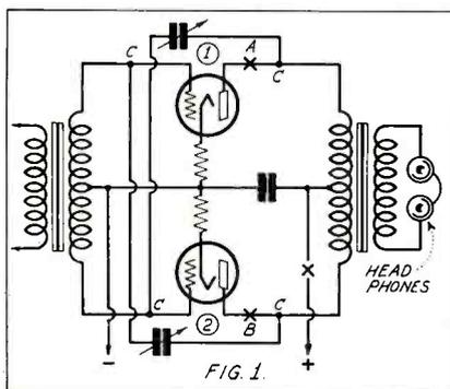
Neutralizing-condenser method of stopping oscillation in the circuits of a push-pull amplifier
