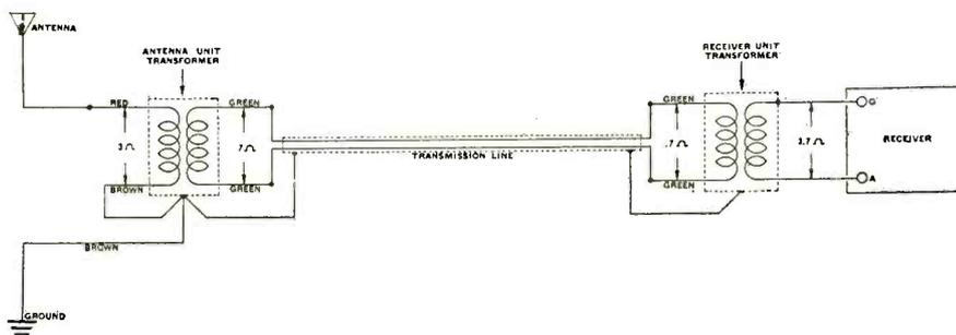
Here is the connection diagram of the Atwater-Kent Type 2-E Interference Eliminator for use in connection with broadcast receivers. The resistance values are given
