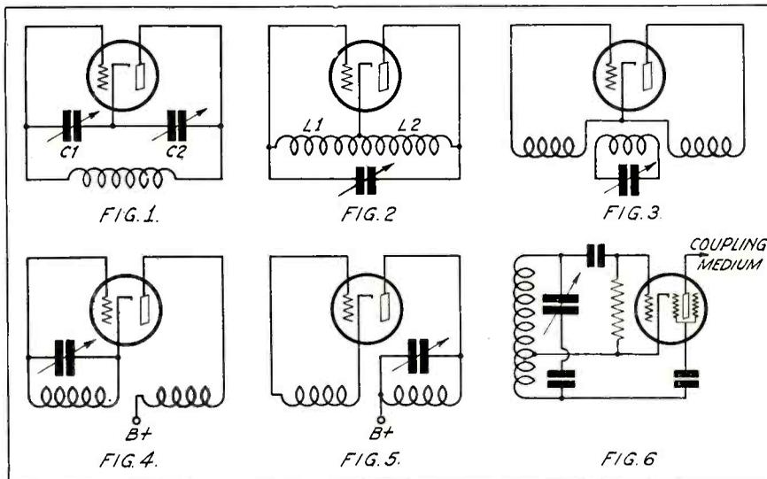
Six different forms of oscillator circuits, most of which are based on the circuit of Fig. 3. Those of Figs. 4 and 5 are most commonly used in superheterodynes. Fig. 6 is an electron-coupled oscillator
