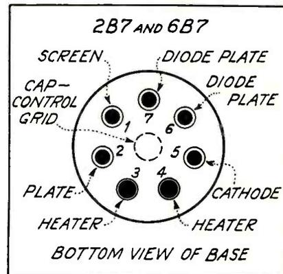
Fig. 5. Base connections for the 2B7 and 6B7 tubes. This is the new small seven-pin base
