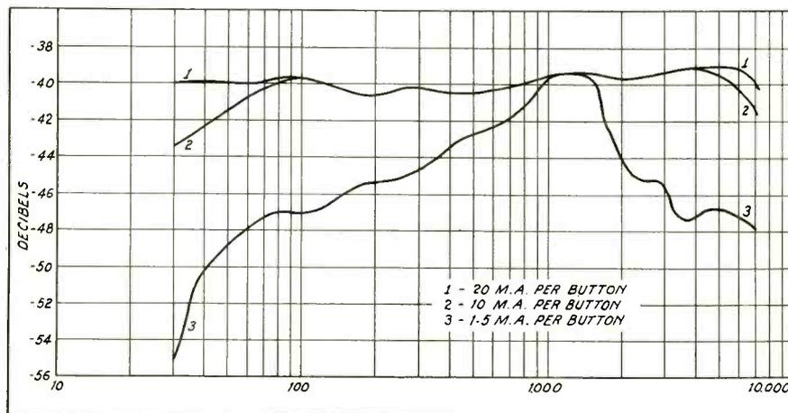
Three curves showing the effects on frequency response of a double-button carbon microphone with changes in button current
