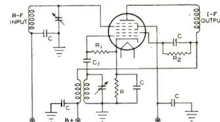
Fig. 2. How a 2A7 or 6A7 is connected up for use as a composite oscillator and mixer in a superheterodyne receiver
