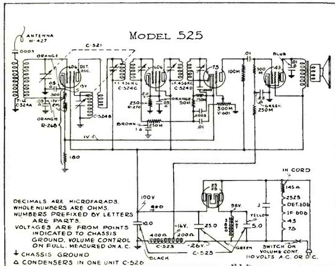
Fig. 1. The schematic diagram of the Belmont Model 525 Midget Super for a-c. or d-c. use. Note that this receiver uses the new 6D6 and type 75 tubes, as well as a 25Z5 rectifier in double half-wave connection
