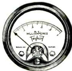
used, it is said. The aluminum needle and other parts are ribbed and made unusually strong throughout. The moving coil is light in weight. The scales are extra long, uniform and easy to read. Sealed cases of one-piece construction means strength and absence of foreign materials.
