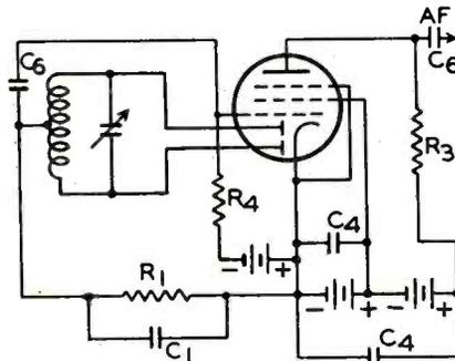
Fig. 4. The 2B7 or 6B7 used as a full-wave rectifier and audio amplifier. In this case the diode plates are used separately
