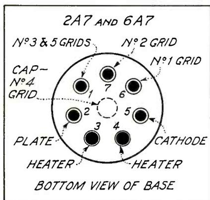
Fig. 1. Base connections for the 2A7 and 6A7 tubes. This is the new small seven-pin base
