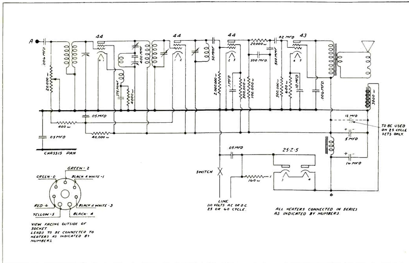
Circuit diagram of the All-American Model U-55 midget receiver. The first tube is a combination oscillator and mixer
