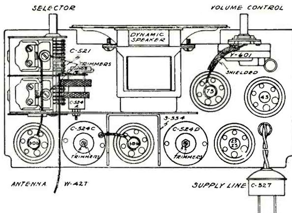
Fig. 2. Top view of the Belmont Model 525 chassis, showing the locations of the tubes, trimmer condensers, etc. The 6D6 tube to the left (as shown here) is the composite oscillator and modulator
