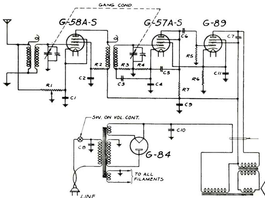
Here is the circuit of the new Majestic Model 380 Midget receiver. This is for a-c. only, with heaters connected in parallel
