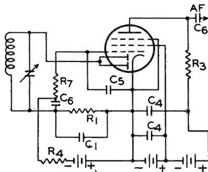
Fig. 3. The 2B7 or 6B7 used as a half-wave rectifier and audio amplifier. The two diode plates are connected together
