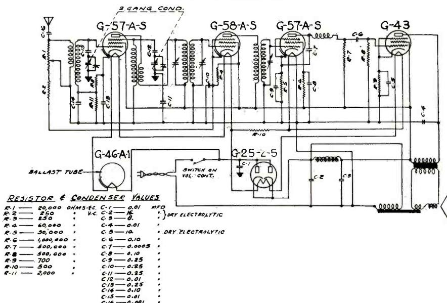
The circuit for the Majestic Model 400—also a midget—which has the heaters of all tubes connected in series, including the ballast tube. The first tube is a composite oscillator and mixer
