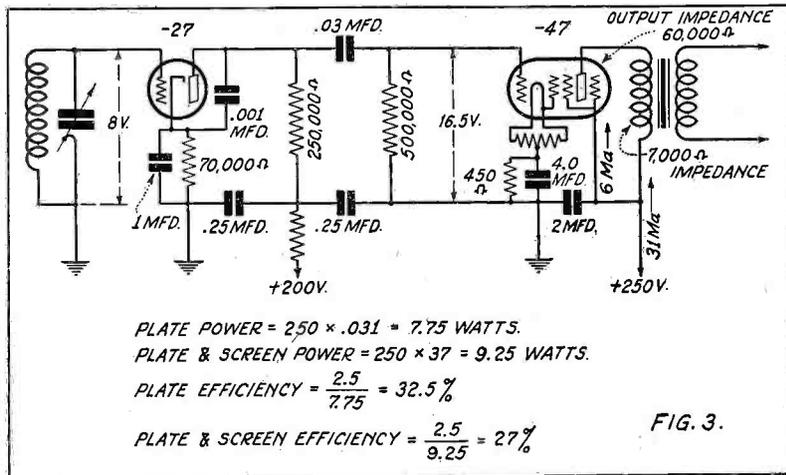
FIG. 3. Circuit with pentode power tube which, because of the high amplification factor of the pentode, requires no intermediate audio stage and works direct from the detector
