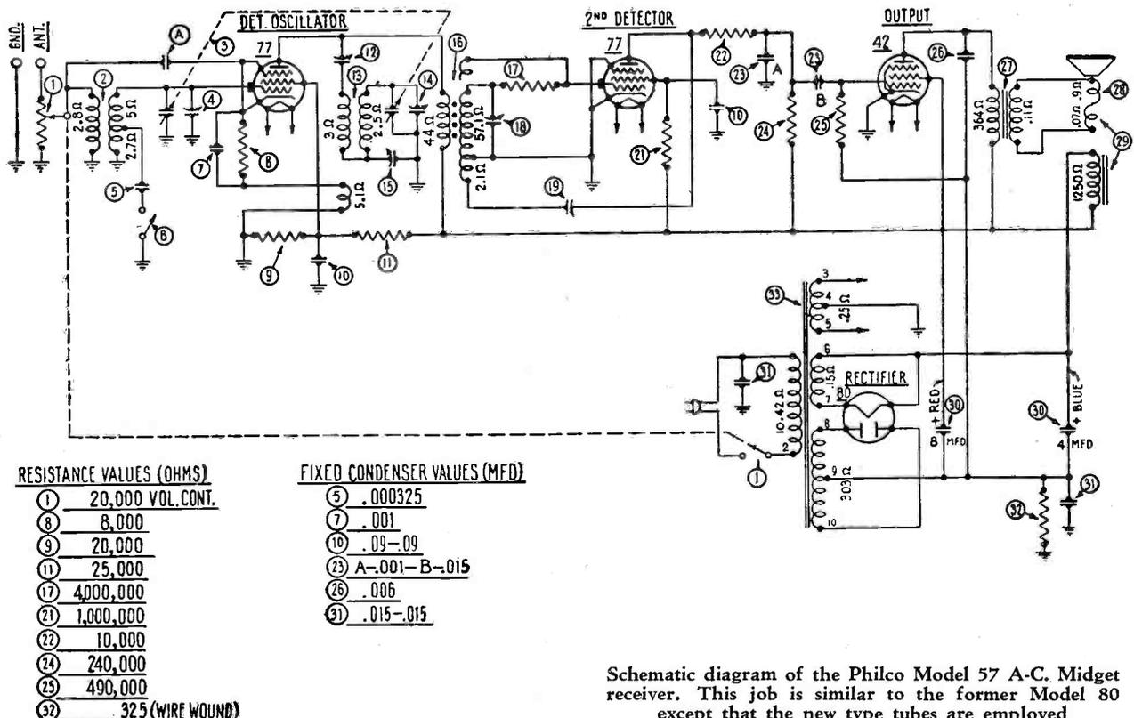
Schematic diagram of the Philco Model 57 A-C. Midget receiver. This job is similar to the former Model 80 except that the new type tubes are employed
