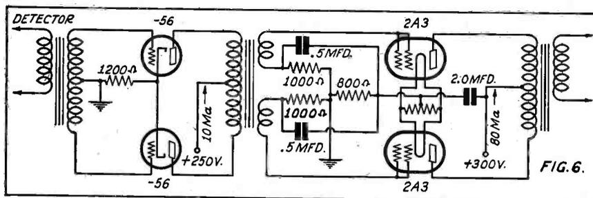
Circuit employing two type 2A3 tubes, with self bias, which operate as semi-Class B tubes at high power
