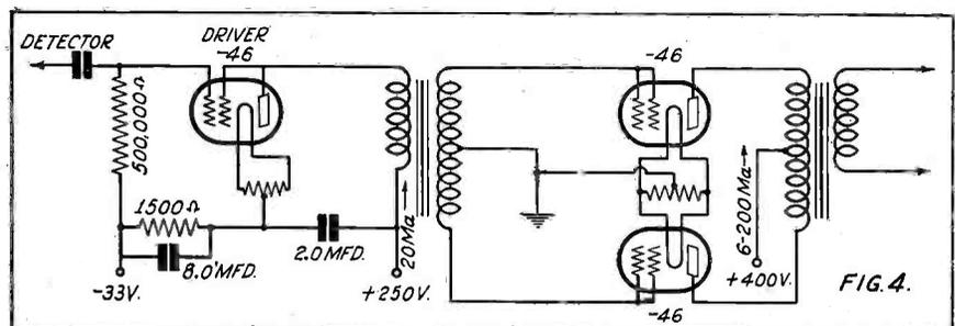
FIG. 4. Circuit of a Class B amplifier using one type 46 as a Class A driver and two type 46s in Class B connection, the two latter tubes operating at zero bias
