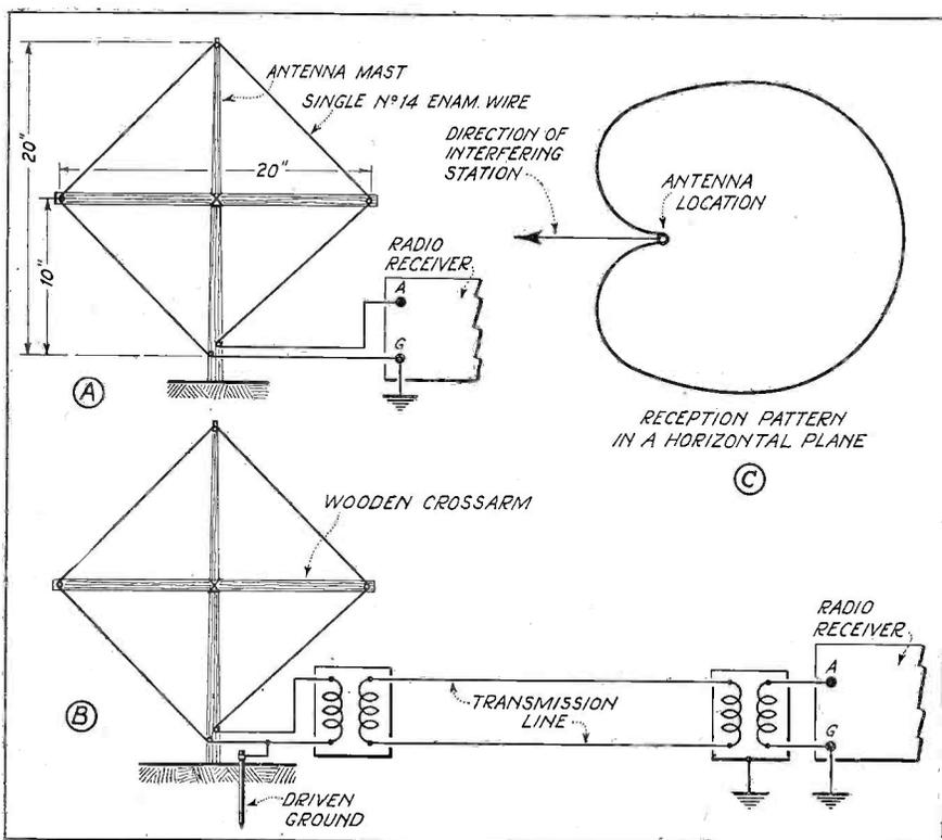
Constructional details and circuit connections of the directional antenna for broadcast reception
