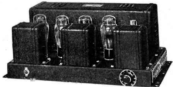
Specifications? WEBSTER SERIES No. 358 AMPLIFIERS are a genuine contribution to the industry. Built around new type tubes, they are the most modern amplifiers obtainable. The Class "A" is 12-15, the "B" 20-26 Watt.
