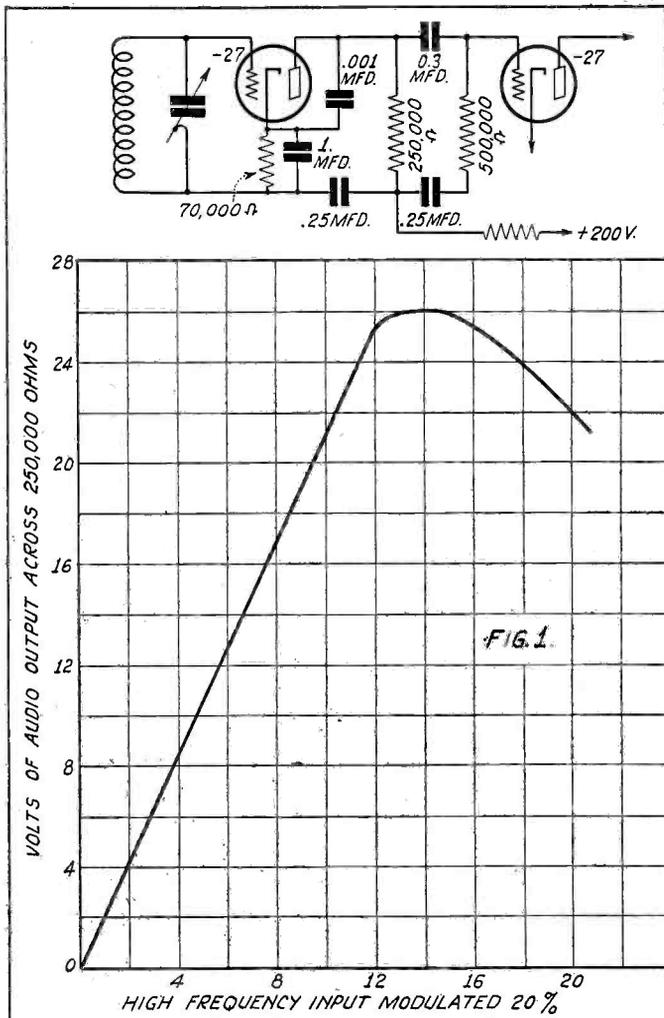
Fig. 1. (Left) The input-output characteristics of a type '27 tube used as a biased detector, with 20 per cent modulation of r-f. or i-f signal
