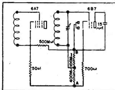
Fig. 5. Skeleton of the I-F. and AVC circuit, with 6A7 and 6B7 tubes
