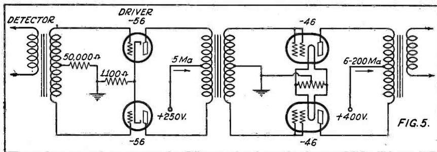
Another Class B circuit, employing two 56's in Class A push-pull as drivers for the 46's. Typical voltage and current values are given
