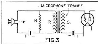
Circuit with the resistance load in the primary circuit
