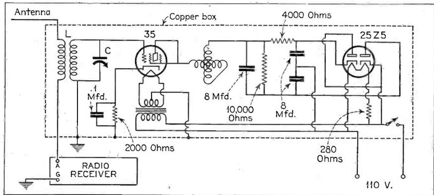
Fig. 3. Complete diagram of the regenerative wave trap
