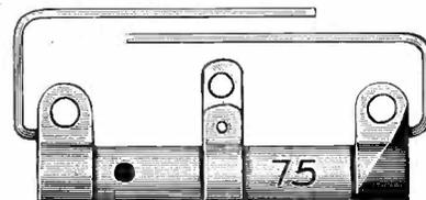
tion of these units the resistance wire is wound over a porcelain core and covered with a special insulating material. Tinned lugs and tinned wire leads on the end terminals are used for connecting the units. Resistors are color-coded and are also marked in numerals.
