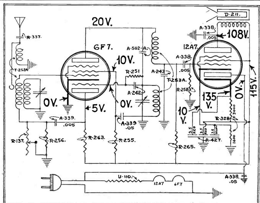
Fig. 2. Diagram of the second Kadette Jr. Values are given in the table above. Color coding and connections of units are shown in Fig. 5 on the next page
