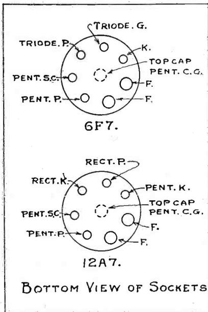
Fig. 3. Socket connections for the Kadette Jr. tubes
