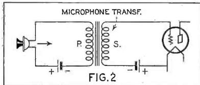
An unloaded condition such as shown causes distortion due to phase shift
