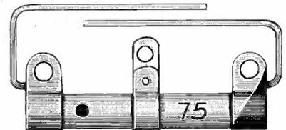
tion of these units the resistance wire is wound over a porcelain core and covered with a special insulating material. Tinned lugs and tinned wire leads on the end terminals are used for connecting the units. Resistors are color-coded and are also marked in numerals.
