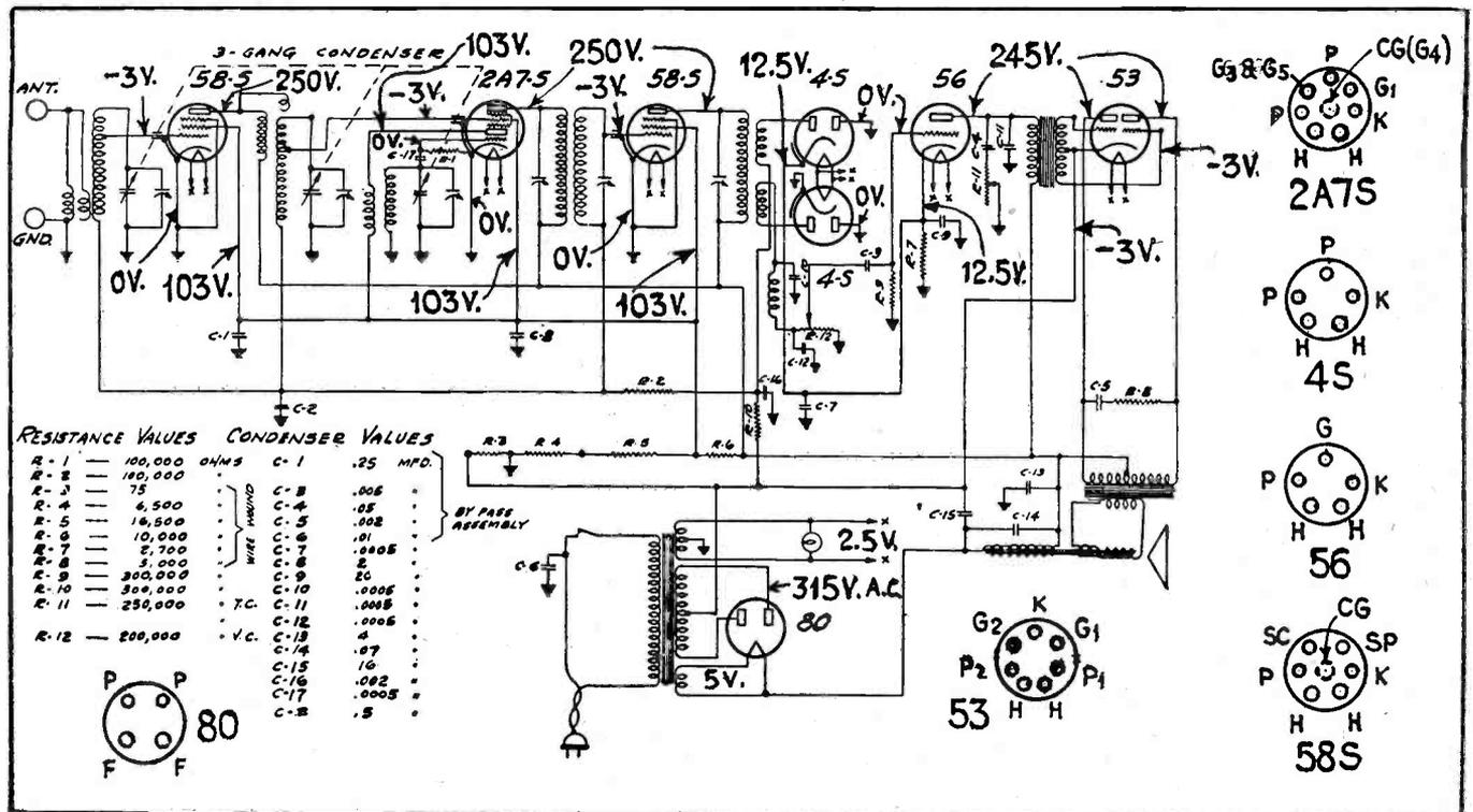
Diagram of the Majestic Model 800 Chassis. Class B is used in the output
