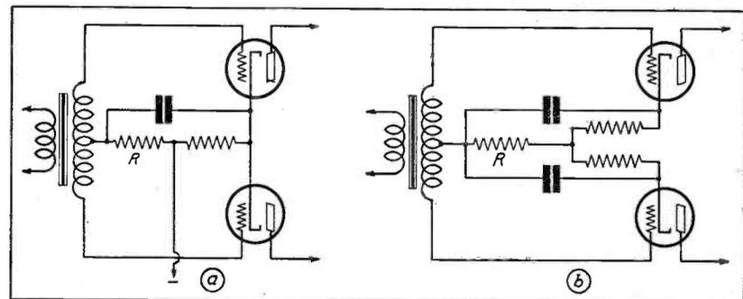
Fig. 4. The filter resistance, R, in either circuit, will tend to eliminate motorboating with fairly low values of bypass capacity
