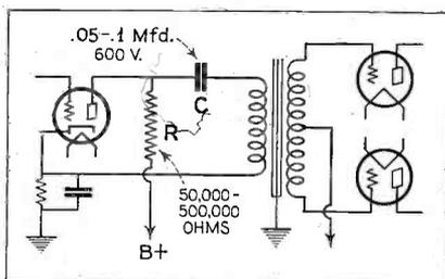
Fig. 2. The primary is now completely isolated, as return goes to cathode
