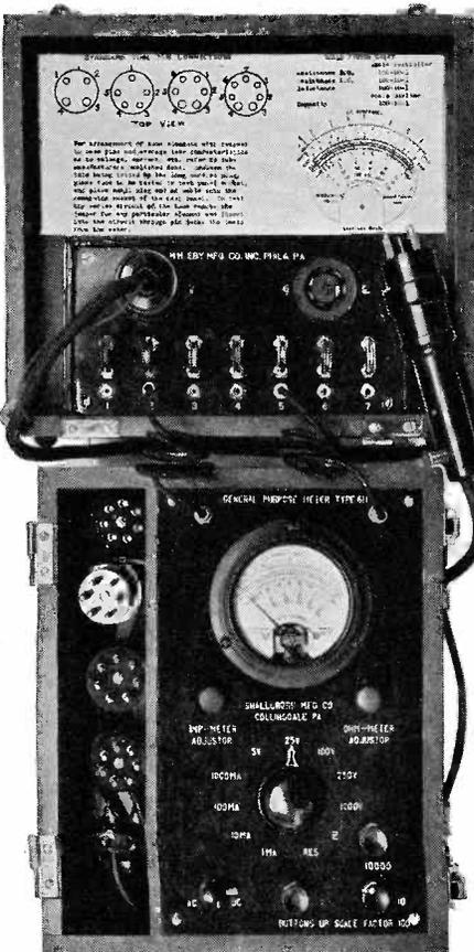
The ranges of this instrument are as follows: D-C Voltage Range (1,000 ohms per volt):—5-25-100-250-1,000 volts. D-C Current Range:—1-10-100-1,000 milliamperes. A-C Voltage Range (1,000 ohms per volt):—5-25-100-250-1,000 volts. Resistance (D-C):—0.5-5,000,000 ohms. Resistance (A.C.):—25-3,000,000 ohms. Capacity:—100-10 mfd. Inductance:—100-10,000 henrys.
