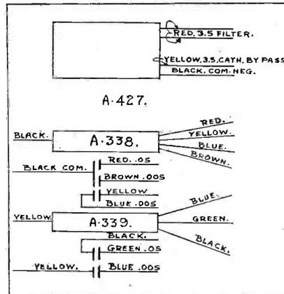
Fig. 5. Coding and connections for the circuit shown in Fig. 2
