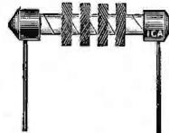
This choke has been designed for high frequency receivers and has extremely low distributed capacity. It consists of four narrow sections, each universally wound. Spaced on an Insulex form. Supplied with several leads, for mounting. May be mounted in grid leak clips if desired.
