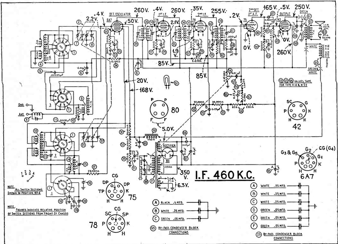
Diagram of the Philco Model 44 All-Wave receiver. Wave change switches progressively short out portions of the coils
