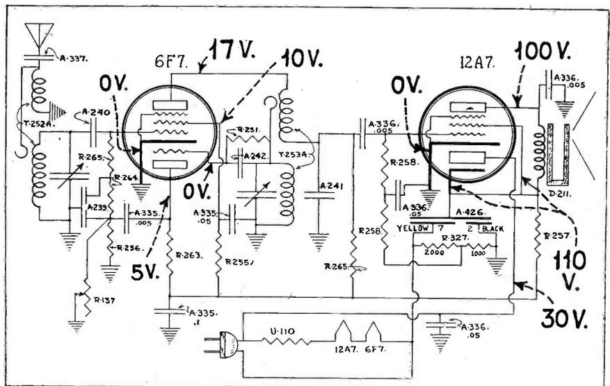
Fig. 1. Diagram of first Kadette Jr. Values are given in the table below. Color coding and connections of units are shown in Fig. 4 on the next page
