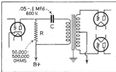
Fig. 1. The primary is not completely isolated from the high voltage
