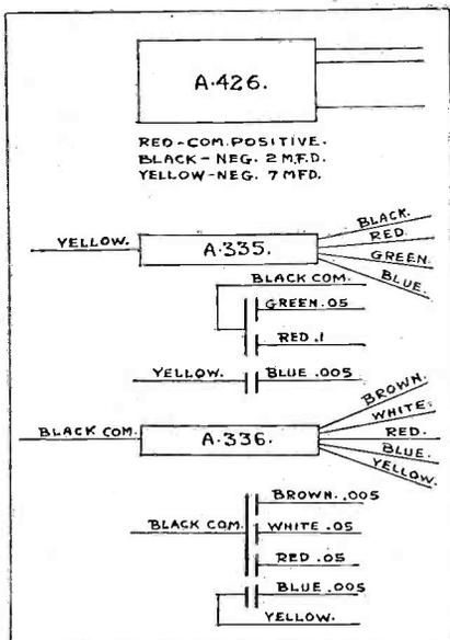
Fig. 4. Coding and connections for the circuit of Fig. 1
