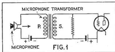
Microphone circuit with secondary of transformer loaded
