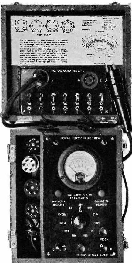
The ranges of this instrument are as follows: D-C Voltage Range (1,000 ohms per volt):—5-25-100-250-1,000 volts. D-C Current Range:—1-10-100-1,000 milliamperes. A-C Voltage Range (1,000 ohms per volt):—5-25-100-250-1,000 volts. Resistance (D-C):—0.5-5,000,000 ohms. Resistance (A.C.):—25-3,000,000 ohms. Capacity:—0.001-10 mfd. Inductance:—100-10,000 henrys.
