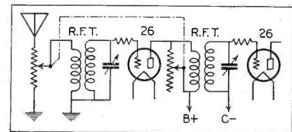
with both tracks of 10,000 ohms or more, connect one side in the antenna circuit much like the Majestic 70, and use the other side for a shunt across the plate winding of the 1st r-f tube. This is shown in the accompanying diagram.
