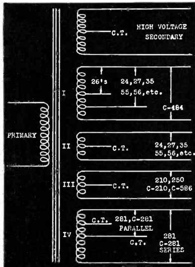
replacement in receivers using such tubes as the '81 half-wave rectifier and 210 amplifier tubes. This transformer also will supply such tubes as the C-484 and C-586 which have 3-volt filaments, as well as the C-210 and one or more '81's in either series or parallel.
