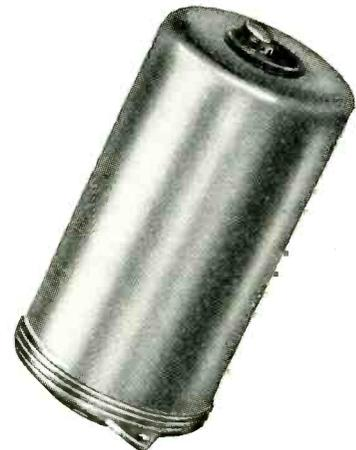
full-wave mechanical rectifier, and it is shielded by a double aluminum case with a felt insulator, the entire vibrator unit being rubber-mounted. It has an efficiency of about 60 percent.
