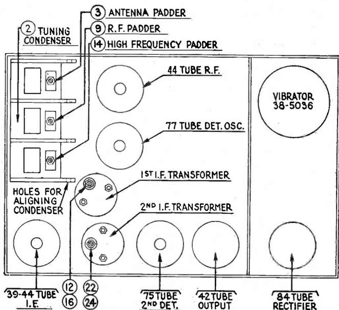
Fig. 2. Diagram showing the location of the various parts and the holes used in aligning the condenser.
