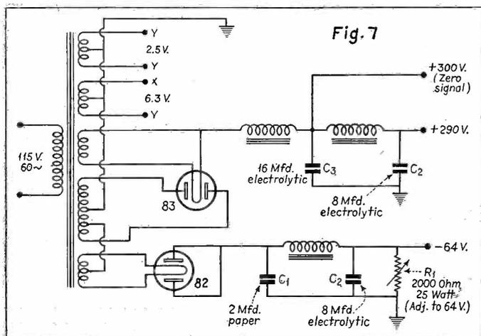
Diagram of the power supply unit. An 83 rectifier is used for supplying the plate voltages and a type 82 rectifier, in half-wave connection, for supplying the bias voltage for the power tubes.
