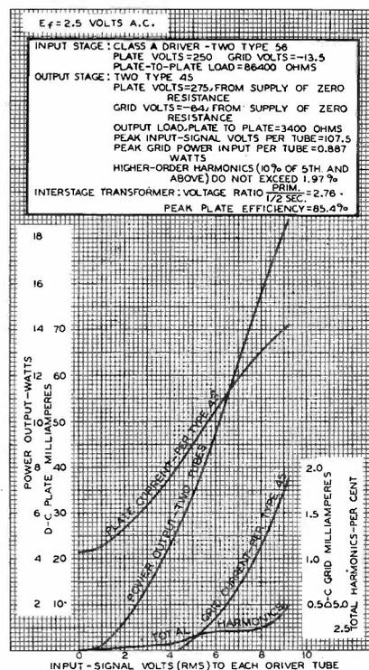
Courtesy RCA Radiotron Co., Inc. Fig. 1. Operating characteristics of type 45 tubes operated Class A-B.
