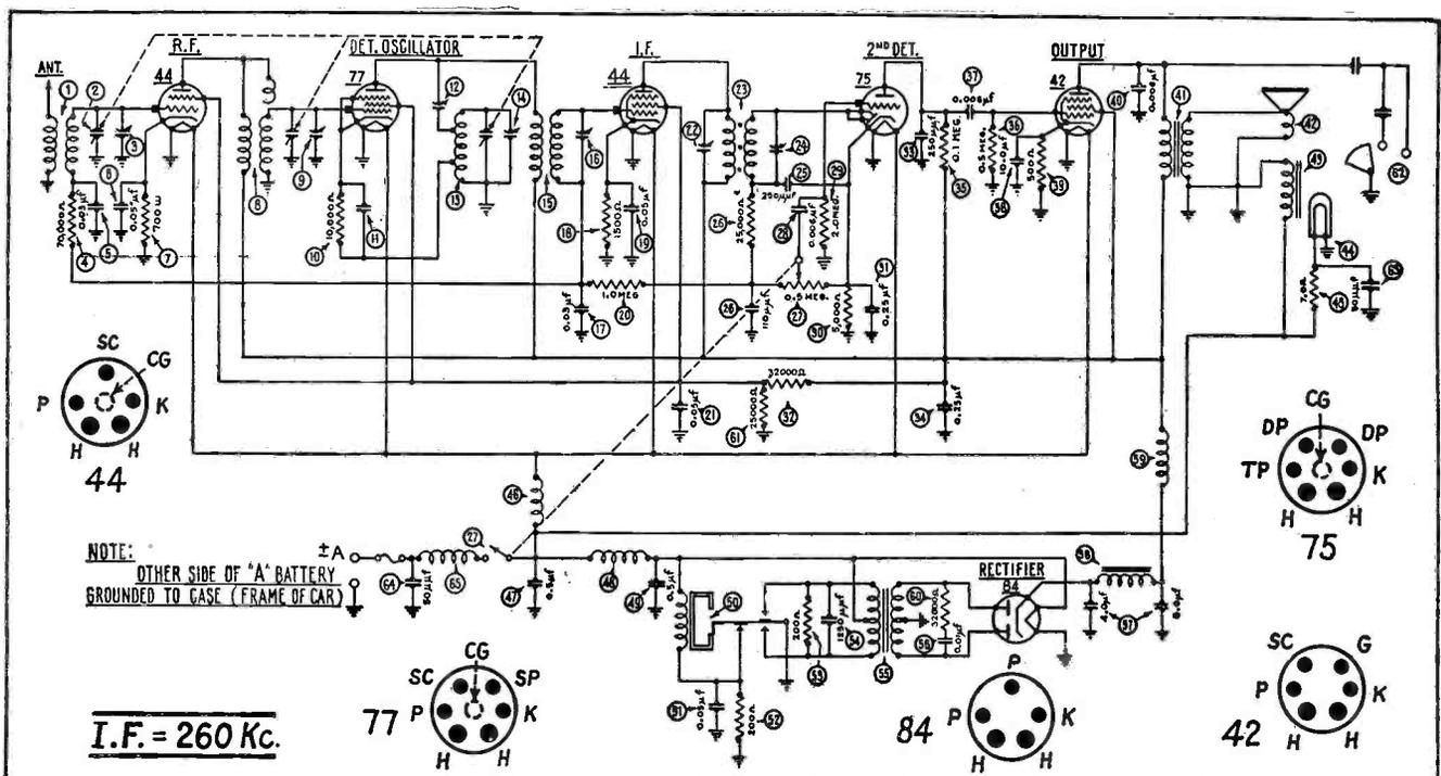
Fig. 1. Schematic of Philco 700.
