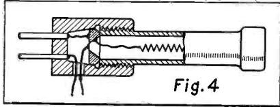
Illustrating a typical series type of receiver wall plug.
