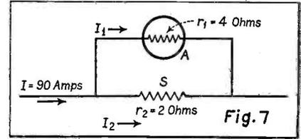
Circuit containing an ammeter and shunt.
