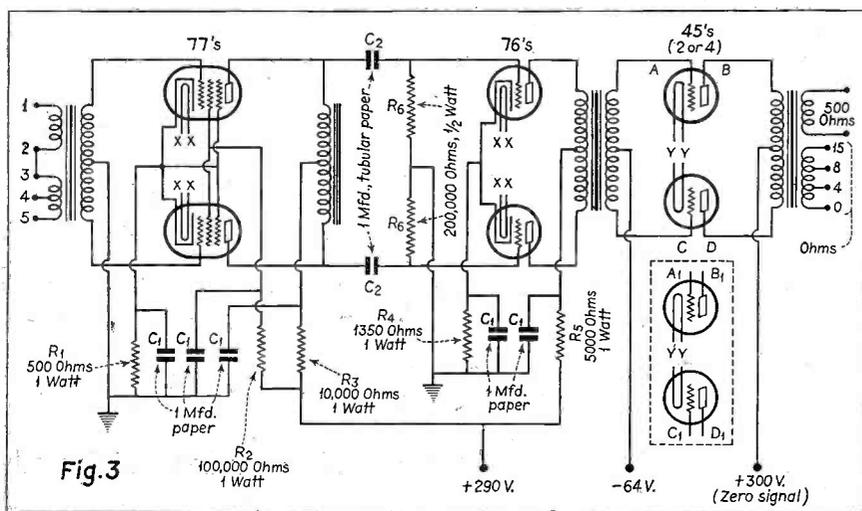
Circuit of the Class A-B amplifier audio channel. Either two or four 45s may be used.
