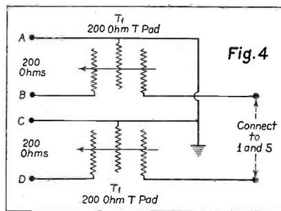
Circuit of the series mixer, for use with 200-ohm input lines.
