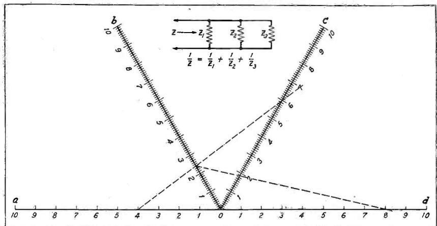
Fig. 6. Chart for finding resultant values of resistances in parallel.
