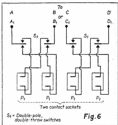
The switching circuit used to change from series to parallel mixer.
