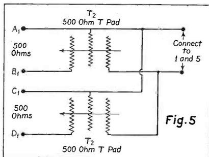
Circuit of the parallel mixer, for use with 500-ohm input lines.
