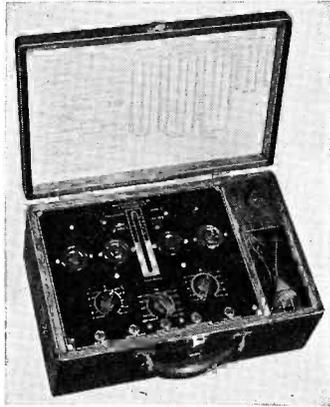
super-sensitive Neon Glow Discharge Tube, which has a two-color scale; this scale indicates at a glance whenever a tube is in good or bad condition. Only four sockets, a 4, a 5, a 6 and a 7-7, are employed in order to simplify the handling of tubes. There are two spares for future tubes and it is also designed to prevent obsolescence.
