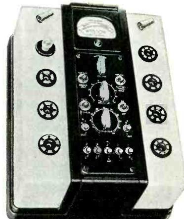
incorporates a fundamental advance in testing tubes on the basis of total emission, in that three separate loads, one for general purpose tubes, one for battery types and one for diodes, are available as required at the throw of a switch. Thus, total emission tests for each type of tube may be obtained on a specific load basis, and without possibility of damage to the tube structure itself.
