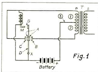
Circuit of typical full-wave shunt vibrator.
