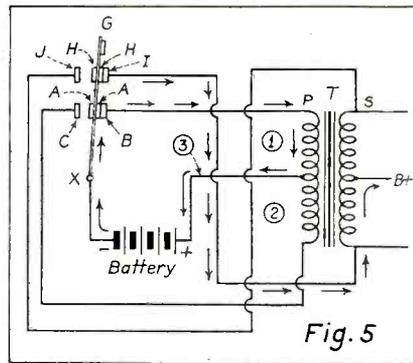
First action of the full-wave synchronous vibrator.
