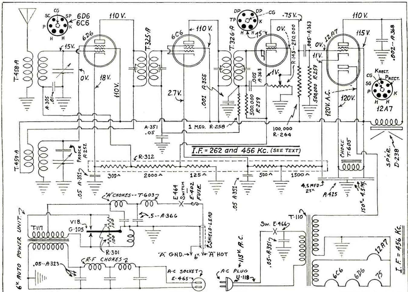
Circuit of International Model 90, together with circuit of attachment for 6- or 32-volt operation.
