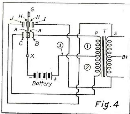
Circuit of typical full-wave synchronous rectifier.
