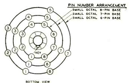
Fig. 2. Base and socket pin-numbering arrangements for the new metal tubes. See Table III on this page.
