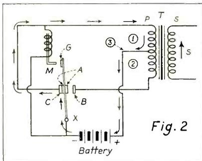
The first functional position of the full-wave shunt vibrator.
